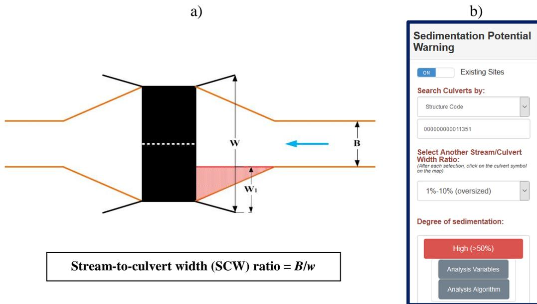
Figure 21. “Sedimentation Potential Warning” workflow: a) definition sketch for the stream-to-culvert (SCW) ratio; and b) forecasting interface for existing culvert sites.
