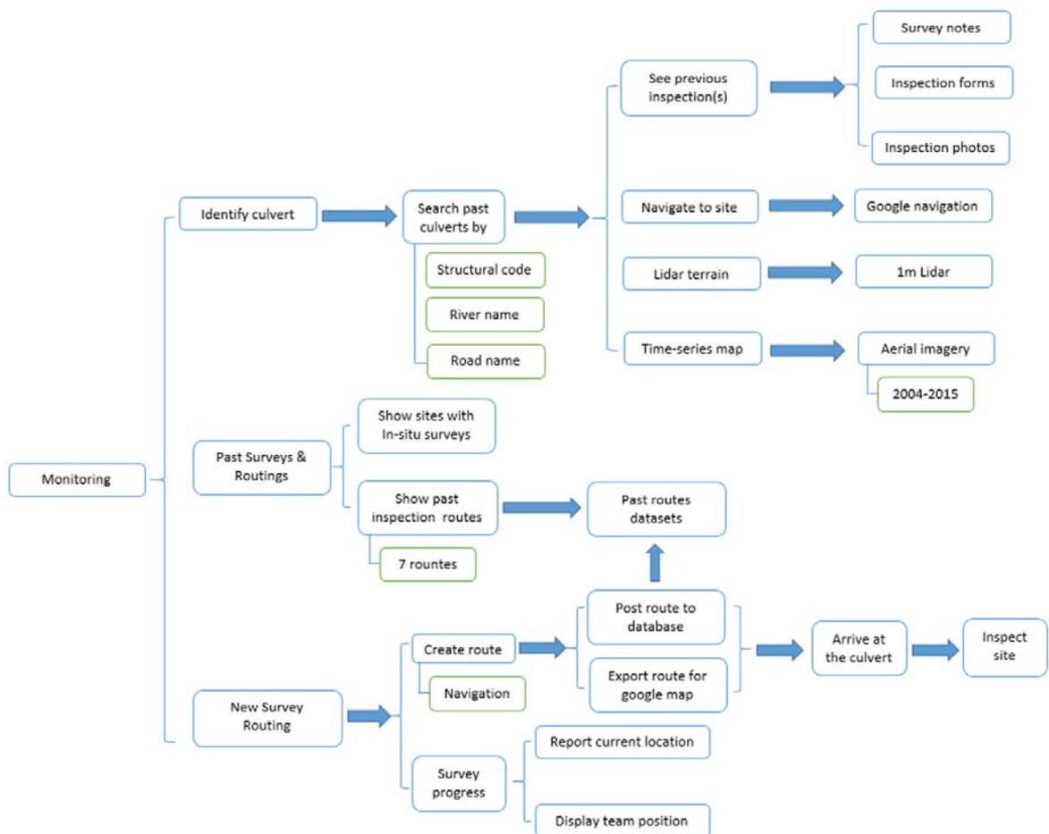
Figure 16a. Flowchart for the “Monitoring” workflow
