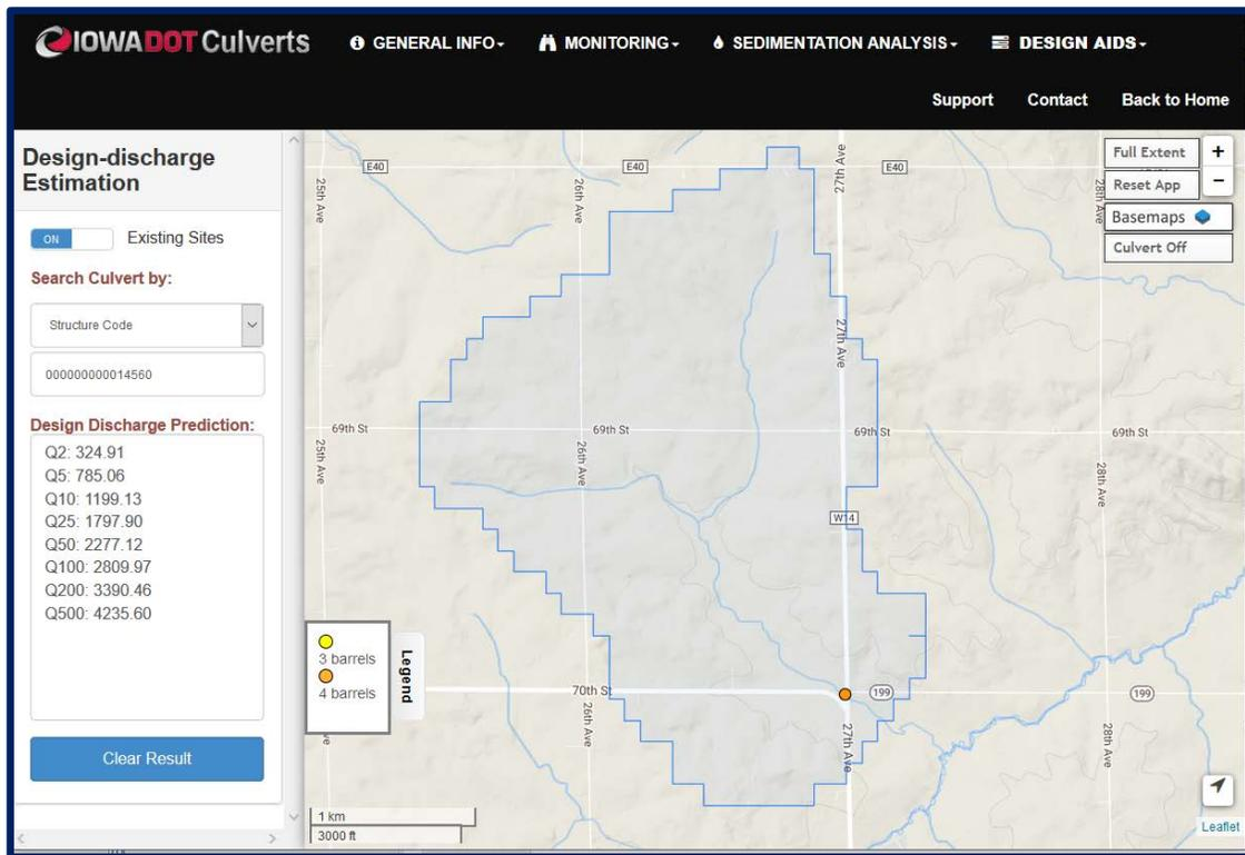
Figure 20. The interface for the estimation of the culvert design discharge (discharge estimates for various return periods are provided in the lower box of the left info panel).
