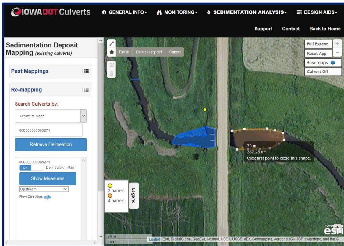
Figure 17. The geo-processing tools associated with the “Sediment Deposit Mapping” workflow. All numerical and textual information are retrieved from the specialized IDOT database (SIIMS), while the graphical information produced during geo-processing is transmitted through Web Map Services (WMS). As the SIIMS information is continuously updated after culvert construction, it is very useful in aiding the mapping process by providing a
