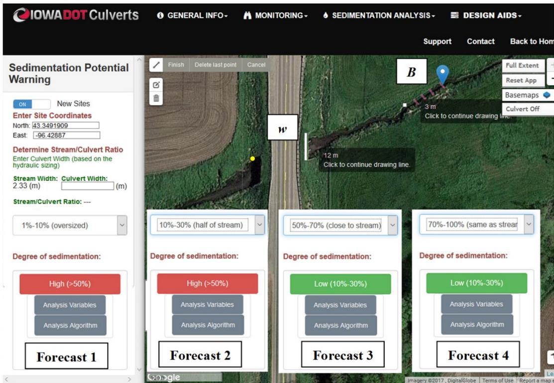
Figure 22. “Sedimentation Potential Warning” workflow for new culvert sites: a) flowchart of the workflow; and b) forecasting interface for new culvert sites.
