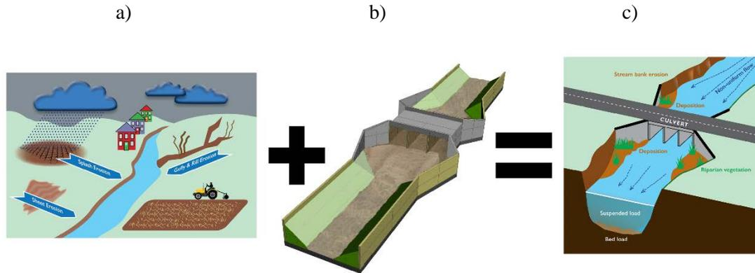
Figure 3. Overview of the processes involved in sedimentation at culverts: a) upland processes (sediment production); b) alteration of the stream geometry in the culvert vicinity; and c) in-stream processes in the vicinity of multi-box culverts.
