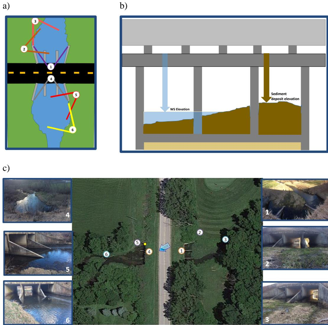
Figure 6. Field measurement protocols: a) positioning of the photo camera for the survey; b) illustration of the measurement acquired for the degree of sedimentation blockage; and c) illustration of the photodocumentation acquired at the culvert site.
