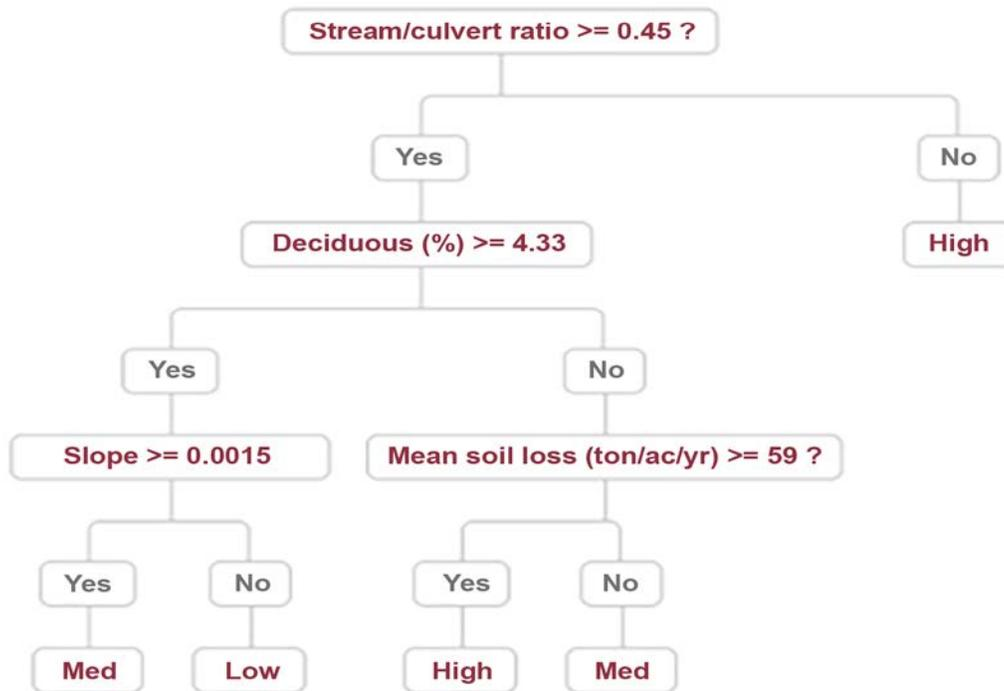
Figure 11. Decision tree representation of the cause-effect relationship between culvert sedimentation and its drivers.
