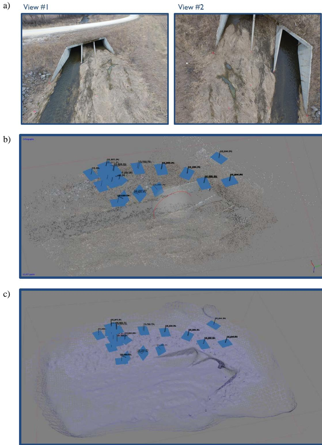
Figure 9. Structure From Motion (SFM) image reconstruction: a) raw images of the culvert inlet; b) image stitching; and c) identification of the tie points for image reconstruction.
