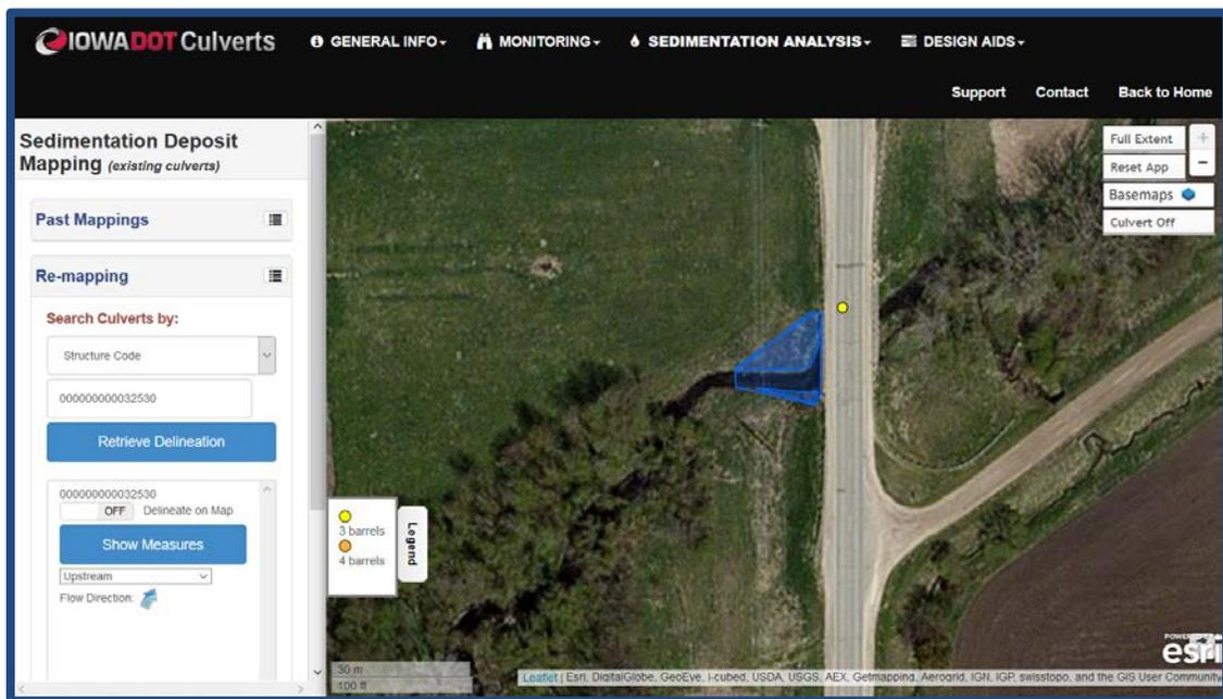
Figure 10. Geo-portal interface for the geo-processing tools associated with the estimation of the degree of sedimentation at culverts.
