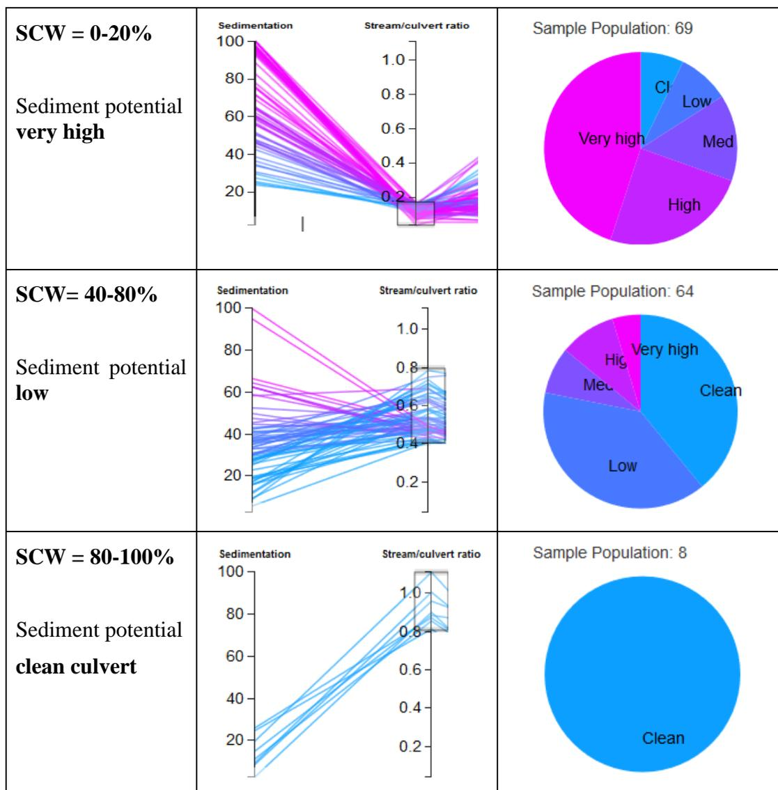
Figure 24. Relationship between the stream-to-culvert width (CSW) ratio and degree of sedimentation at culvert.
