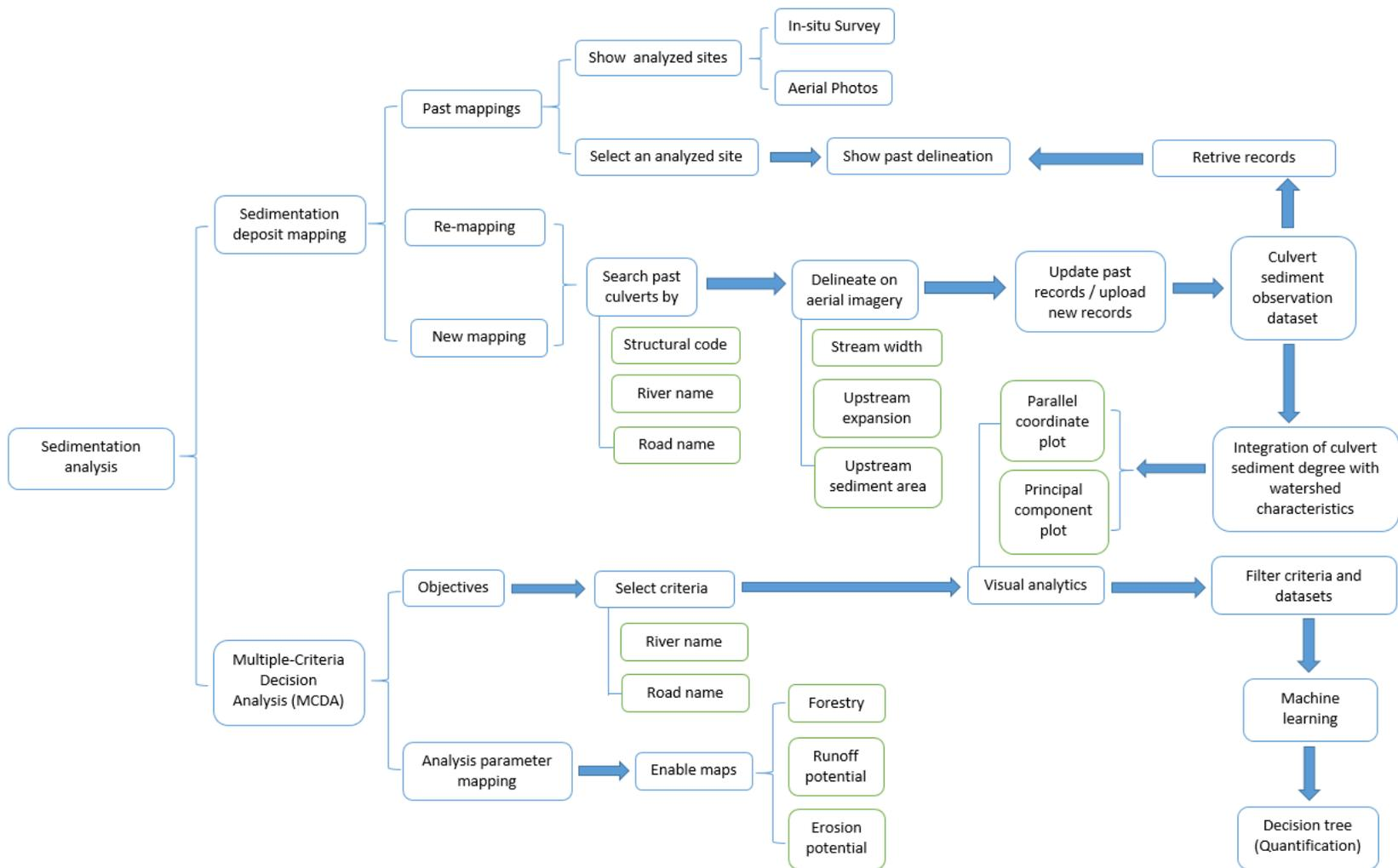
Figure 18b. The tree-like structure used for the Multi-Criteria Decision Analysis applied to the sedimentation at culverts.
