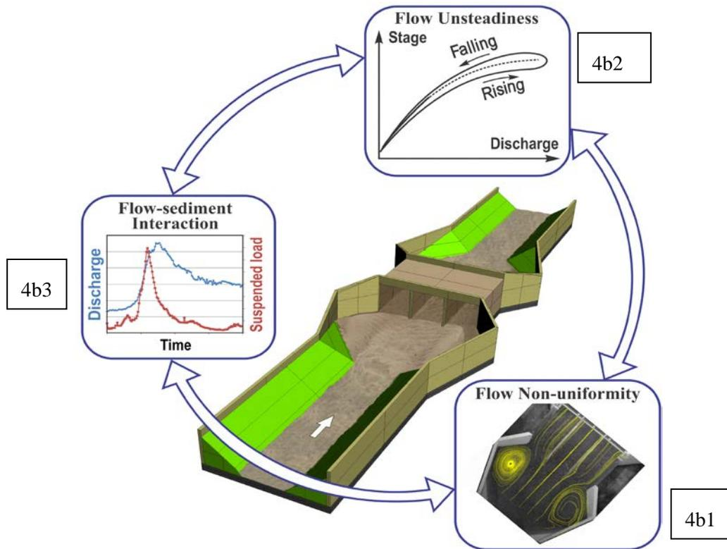
Figure 4. Flow configuration and behavior at culverts: a) non-uniform flow patterns in the vicinity of the culverts (patterns vary with the streamflow magnitudes); b) flow complexities due to flow unsteadiness.
