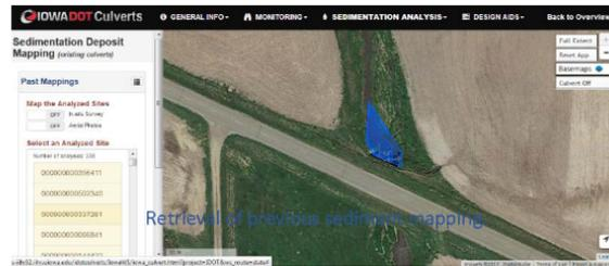
The tools under the “Re-mapping” tab allow users to update and modify past sediment delineations when the latest aerial imageries become available. The “New Mapping” tab, in contrast, allows users to search and map sediment at new culverts. Both tabs have a built-in culvert search tool that only allows users to search and select culverts that have sediment mapping records.
