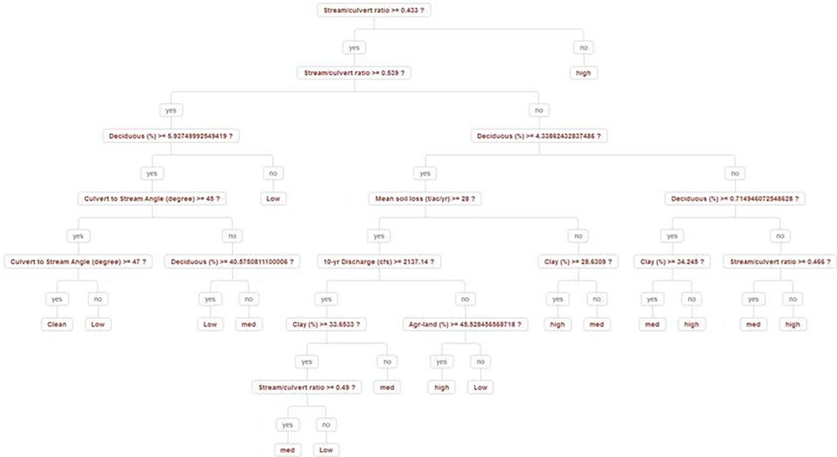
Figure 18a. The tree-like structure used for the Multi-Criteria Decision Analysis applied to the sedimentation at culverts.
