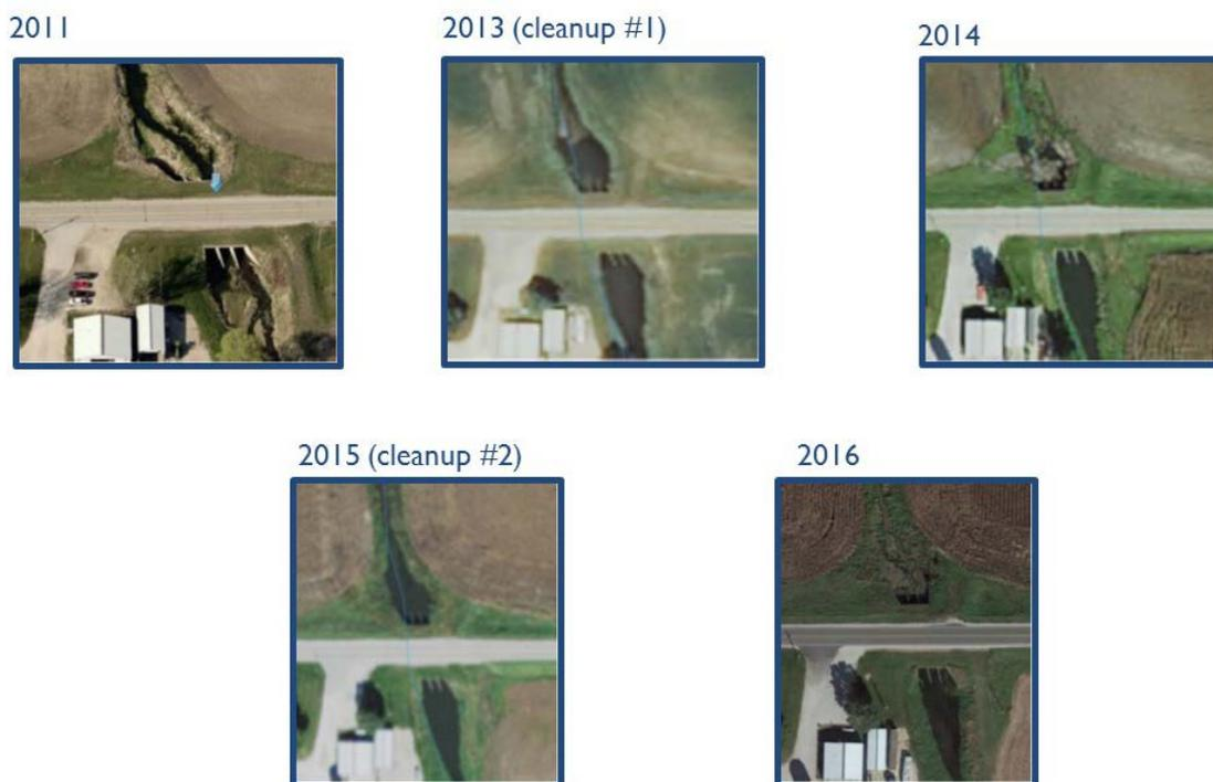
Figure 2. Sedimentation is fast and can quickly reduce a culvert’s conveyance capacity.
