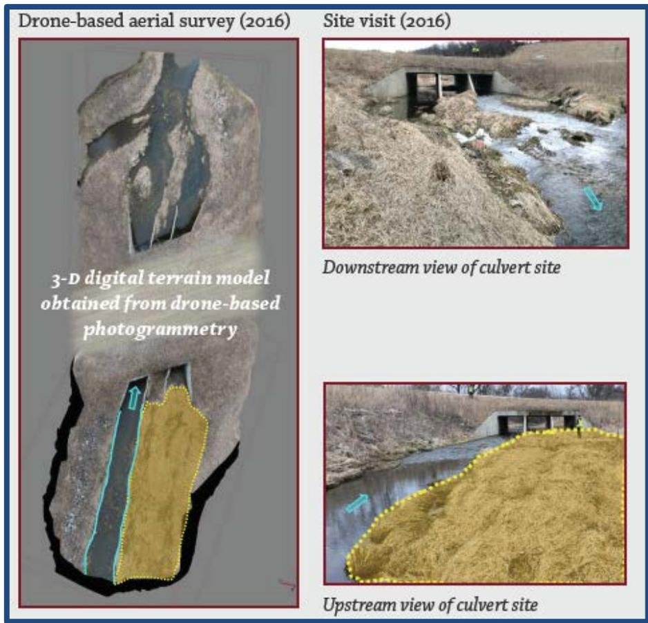
Figure 8. Drone-based culvert surveys: a) data acquisition; b) processed data and comparison between aerial- and ground-based photo-documentation.
