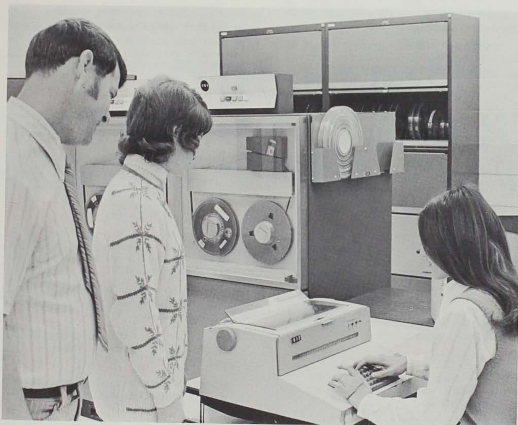
An electronic data processing systems installation with the central processing unit, the computer, and the tape and disk units for storing information.
