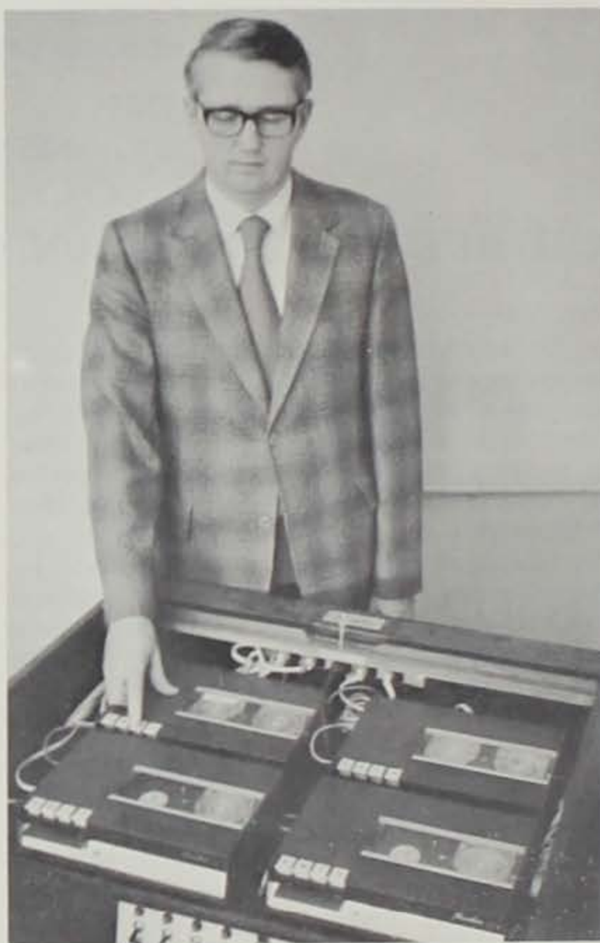
The multiple-listening console, utilizing tapes, broadcasts four different types and / or speeds of dictation simultaneously.
