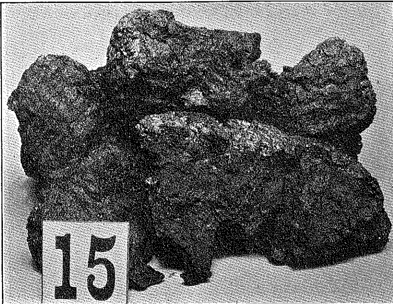
FIG. 12. Coke from Marion County coal. Pershing Coal Co.
