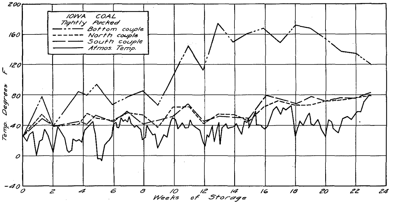
FIG. 4. Curves showing temperatures in tightly packed Iowa coal.
