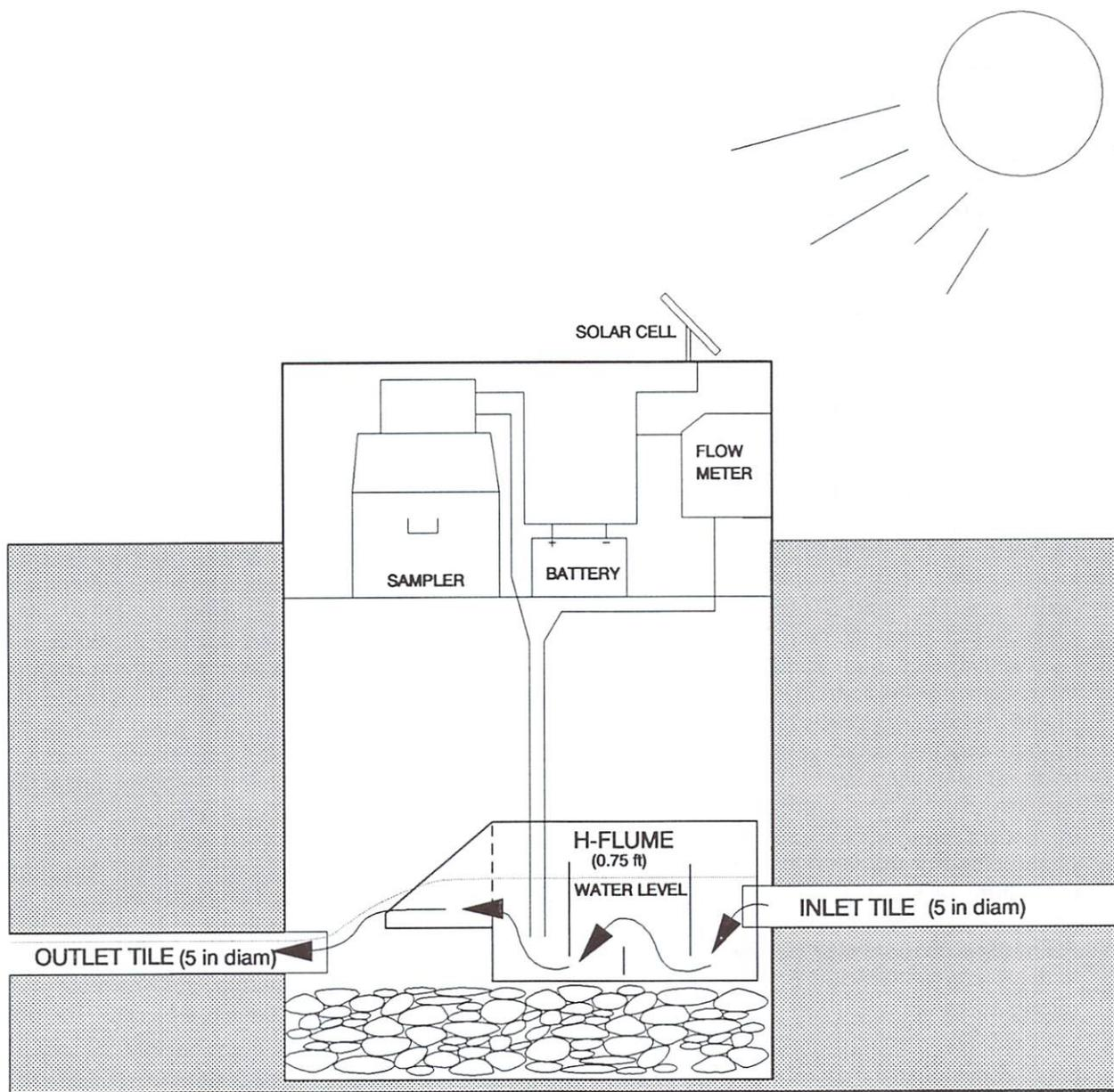
Figure 8. Diagram of monitoring sumps at L22T and BTLD.
