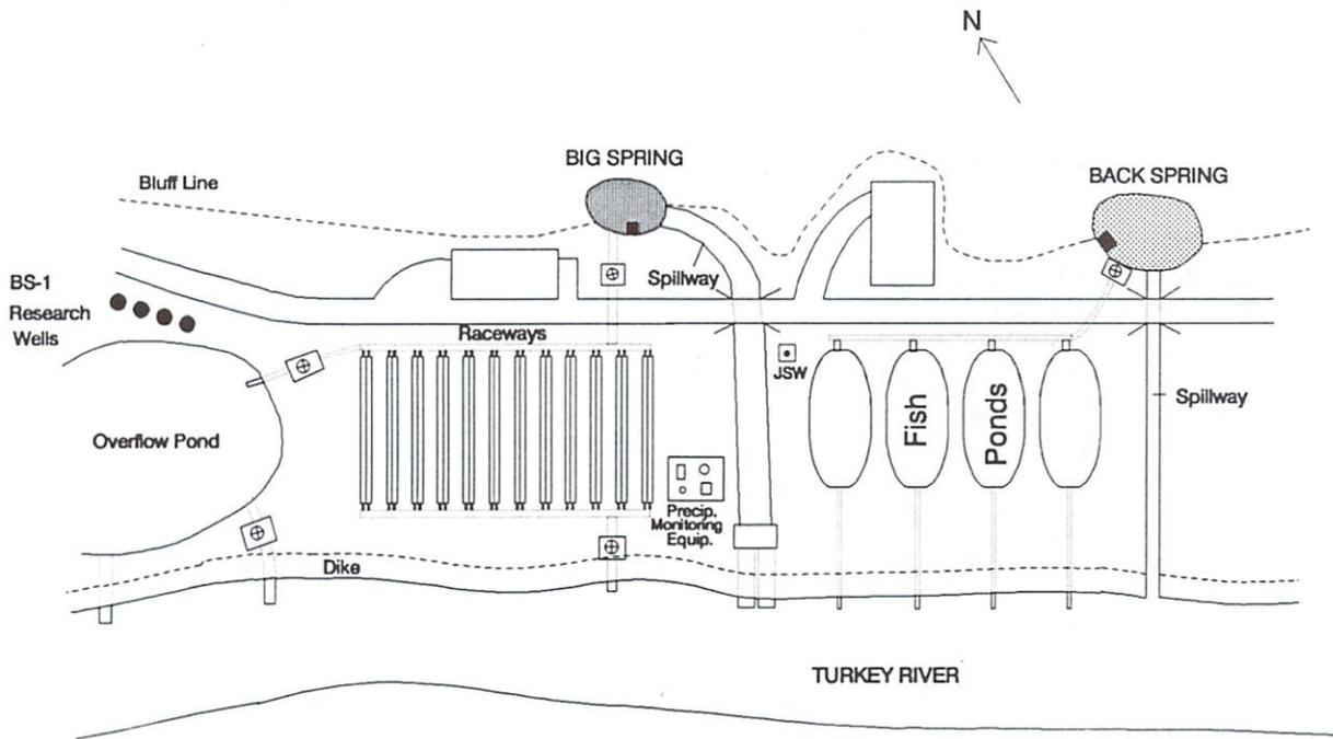
Figure 10. Diagram of Big Spring Hatchery. Dotted lines indicate structures that are underground.
