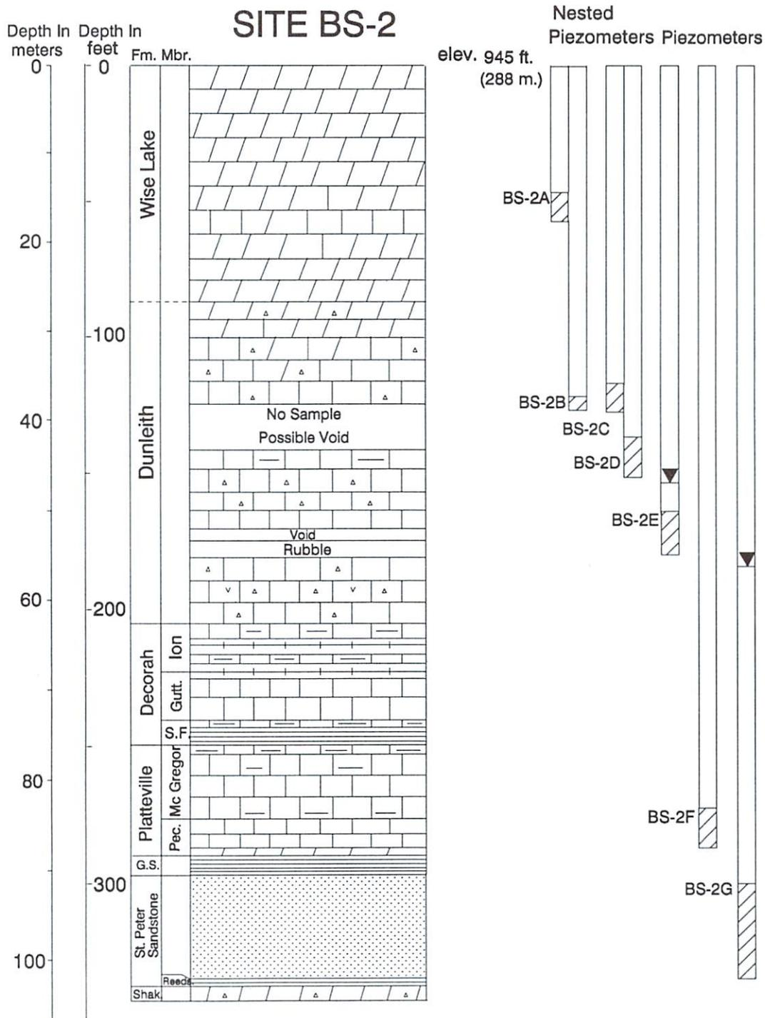
Figure 10. Stratigraphic sequence and monitoring-well installations at site BS-2 (core logged by M. J. Bounk).
