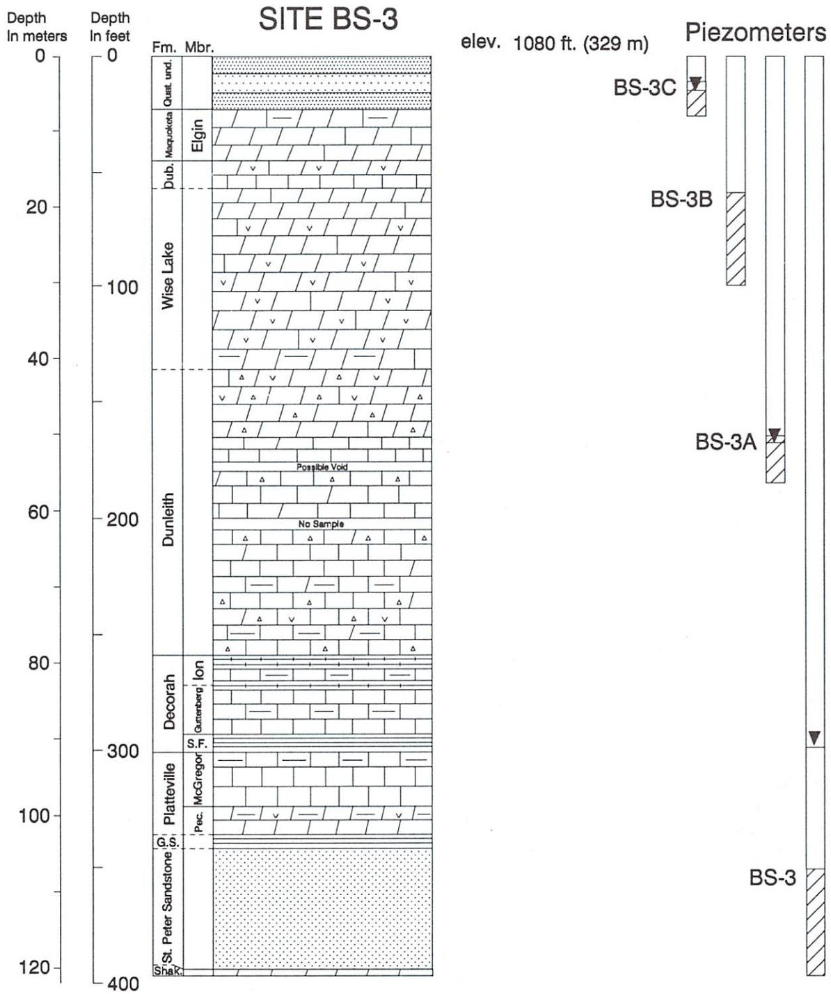
Figure 12. Stratigraphic sequence and monitoring-well installations at site BS-3 (core logged by M. J. Bounk).
