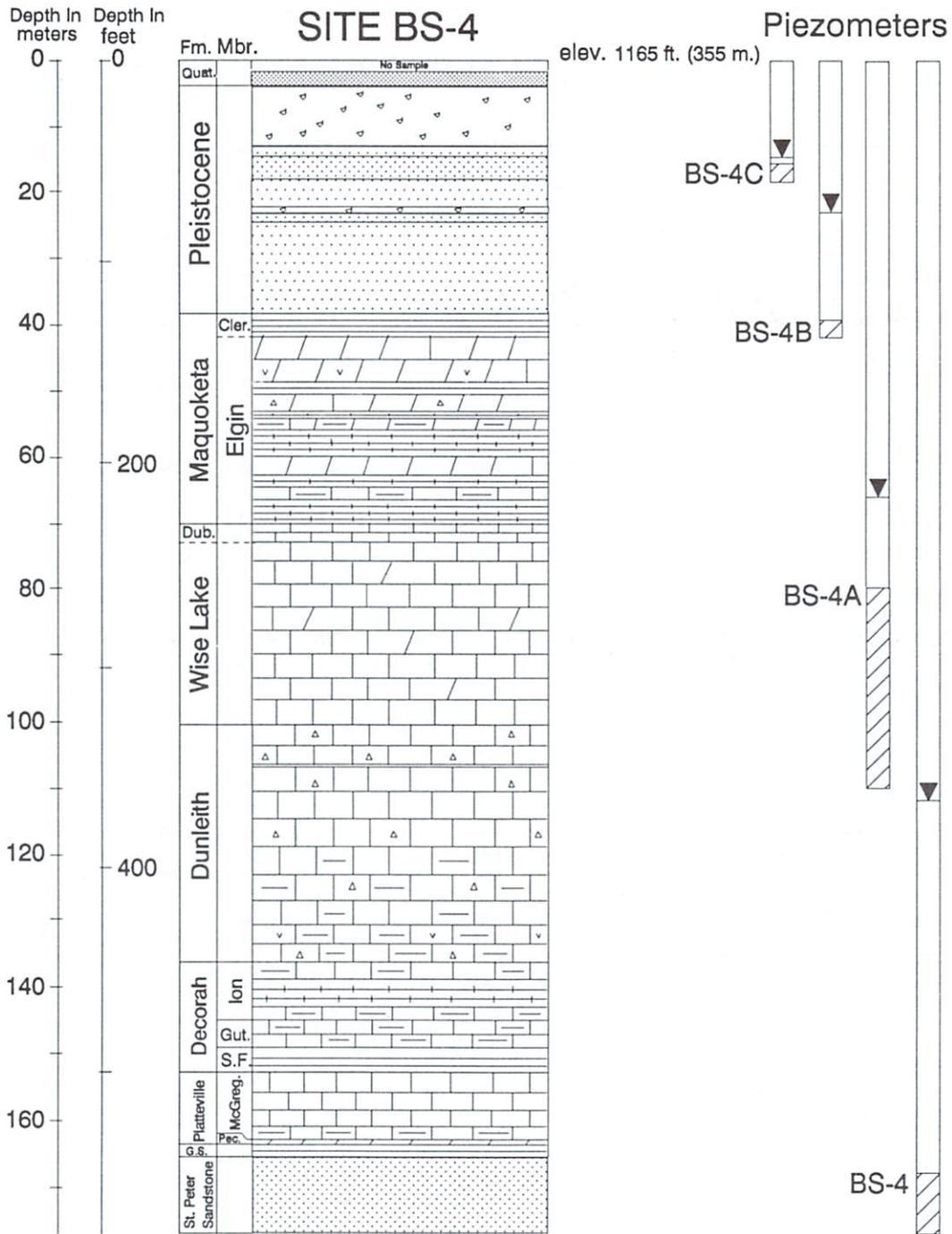
**Figure 13.** Stratigraphic sequence and monitoring-well installations at site BS-4 (core logged by M. J. Bounk).
