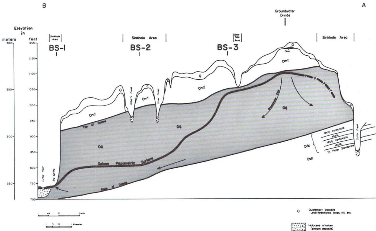
**Figure 5.** Hydrogeologic cross-section A-B; location shown on figure 3. Also shown are projected locations of monitoring-well sites (adapted from Hallberg et al., 1983). See figure 1 for legend.
