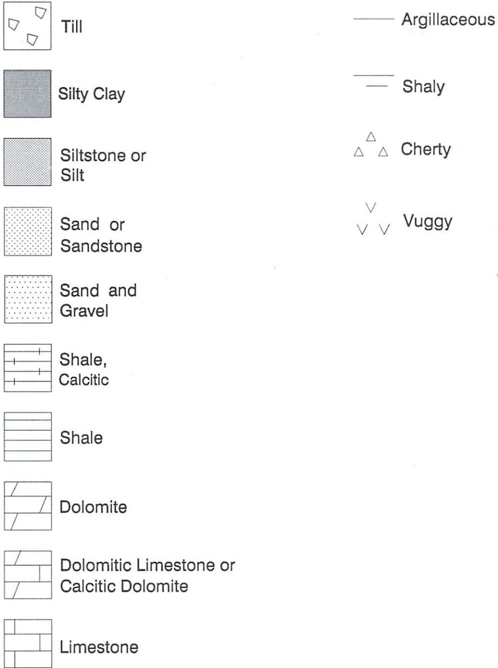
Figure 8. Lithologic key for figures 9 through 13.
