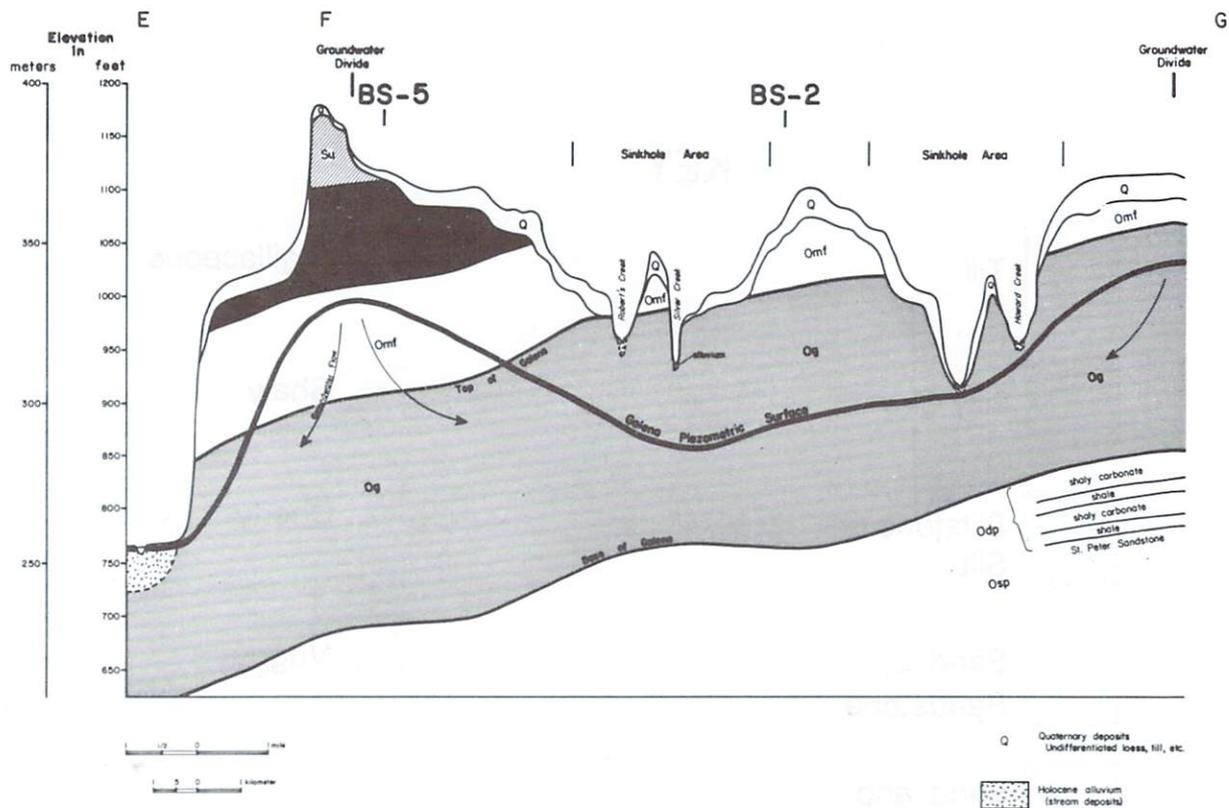
Figure 7. Hydrogeologic cross-section E-F-G; location shown on figure 3. Also shown are projected locations of monitoring-well sites (adapted from Hallberg et al., 1983). See figure 1 for legend.
