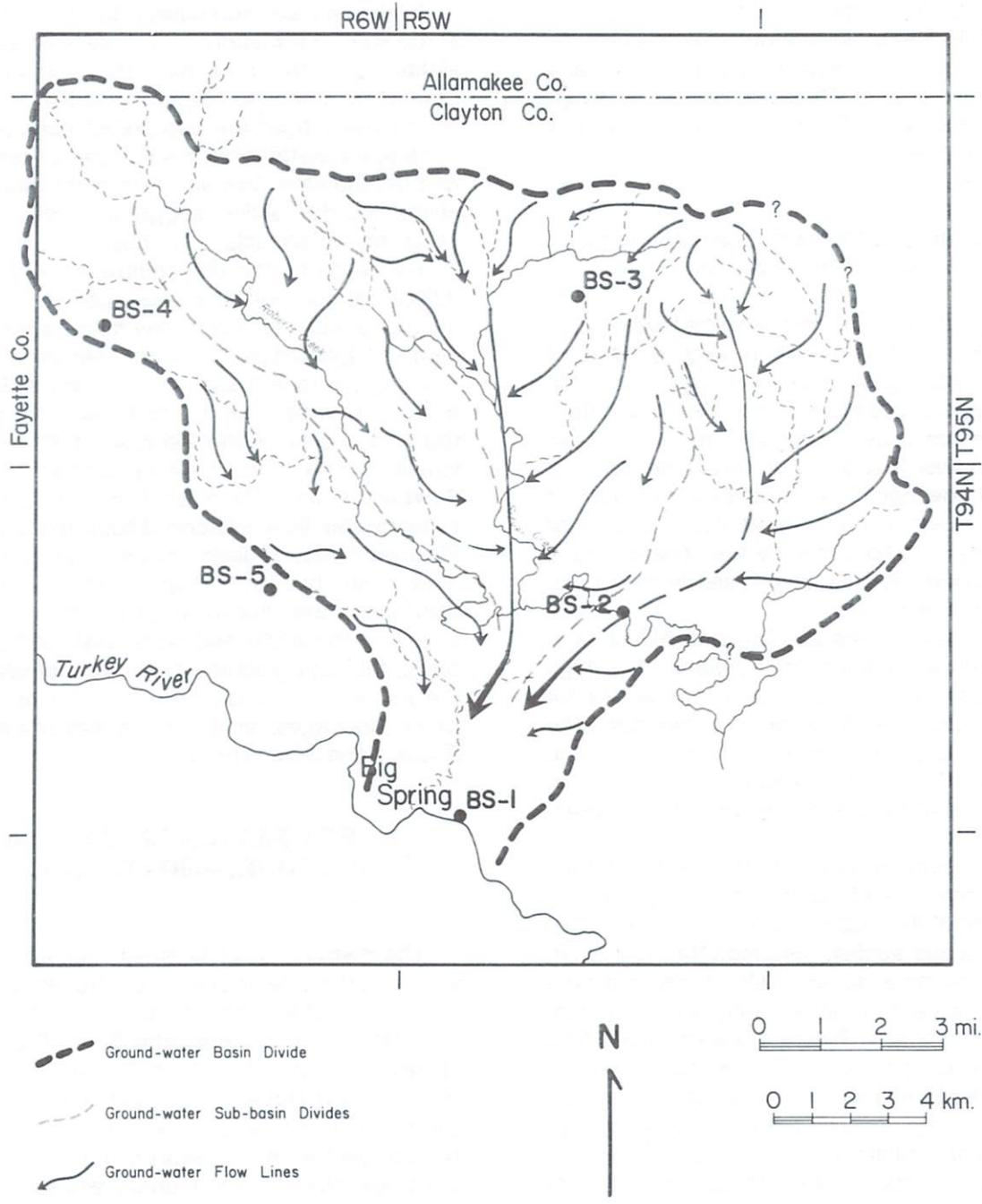
Figure 4. Groundwater basin and subbasin divides, and schematic groundwater flow lines based on the water table/potentiometric surface map (adapted from Hallberg et al., 1983).
