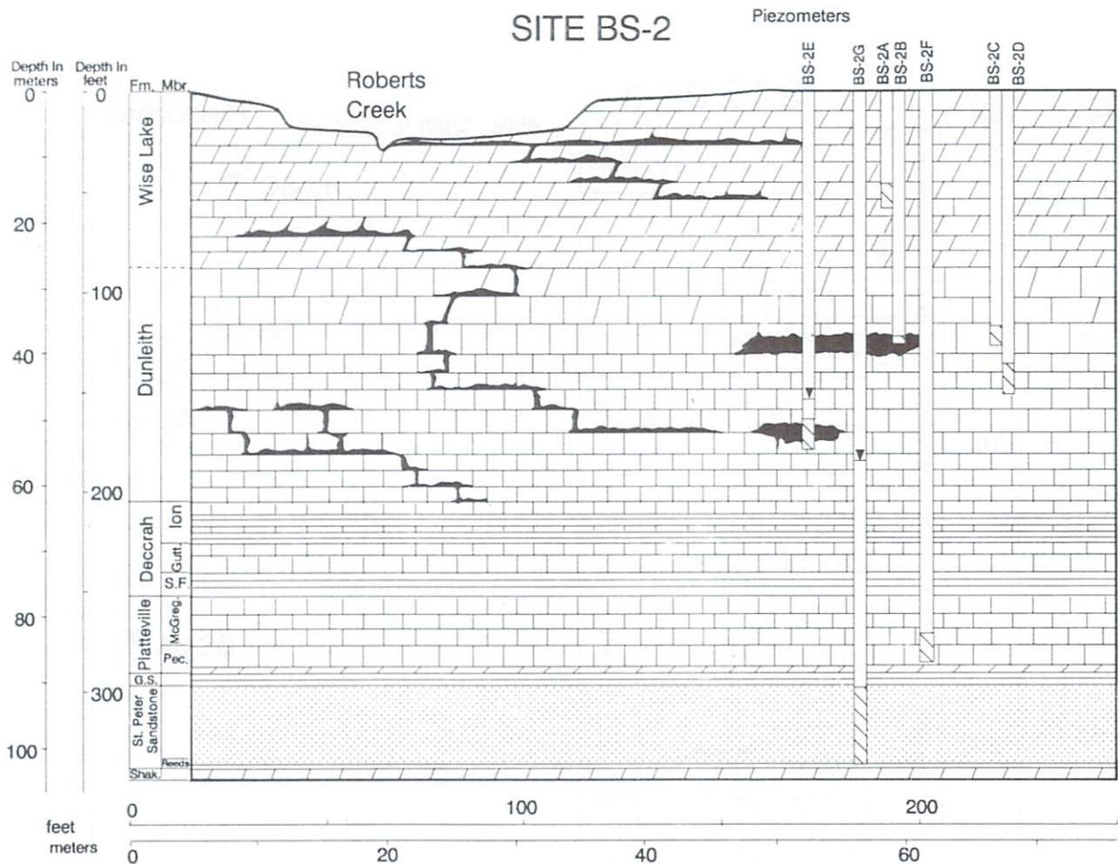
**Figure 11.** Geologic cross-section and monitoring-well installations at site BS-2. Shaded areas represent documented or inferred solution voids and solutionally enhanced fractures and bedding planes (core logged by M. J. Bounk).
