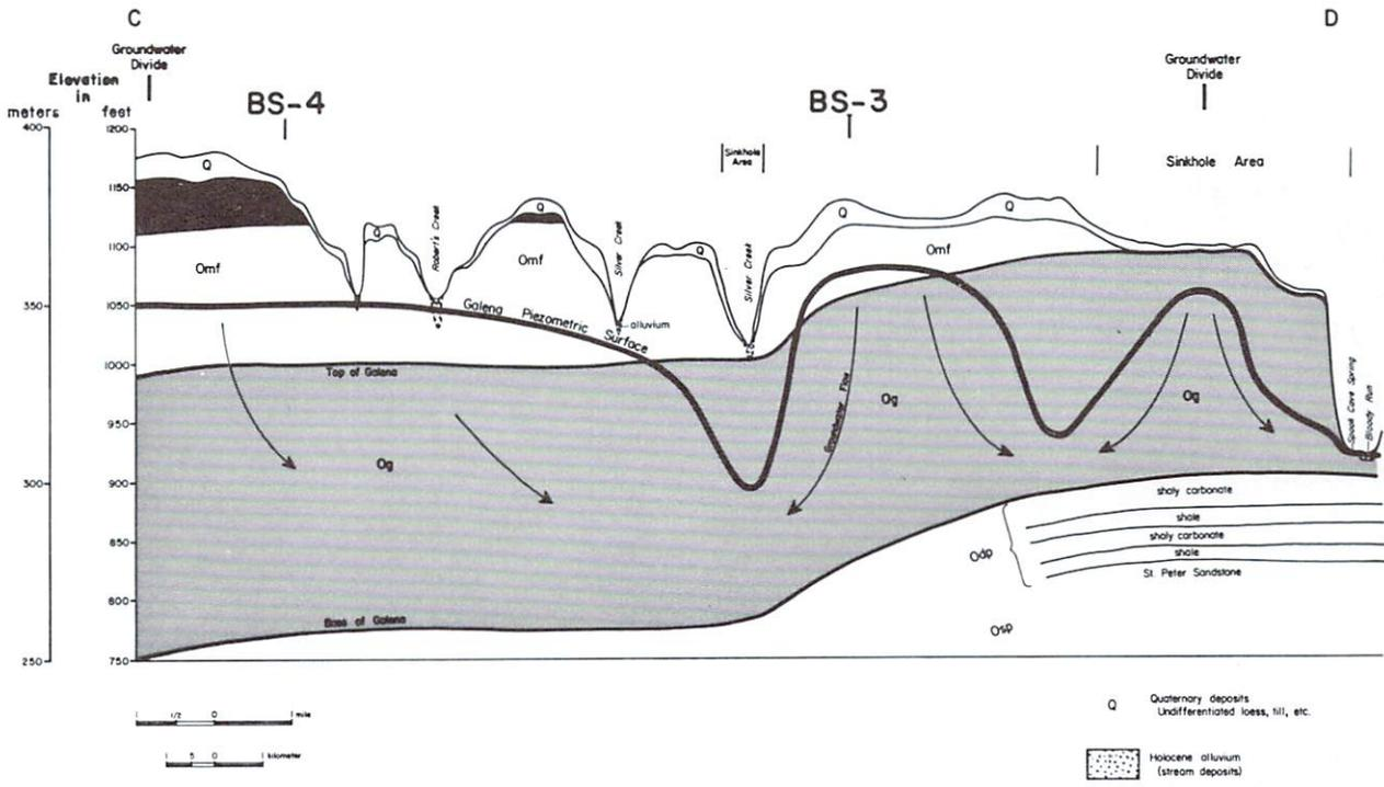
**Figure 6.** Hydrogeologic cross-section C-D; location shown on figure 3. Also shown are projected locations of monitoring-well sites (adapted from Hallberg et al., 1983). See figure 1 for legend.
