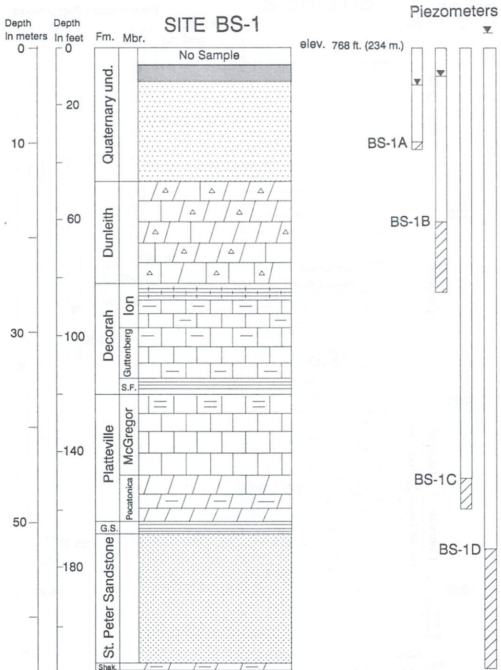
**Figure 9.** Stratigraphic sequence and monitoring-well installations at site BS-1 (cuttings logged by M. J. Bounk).
