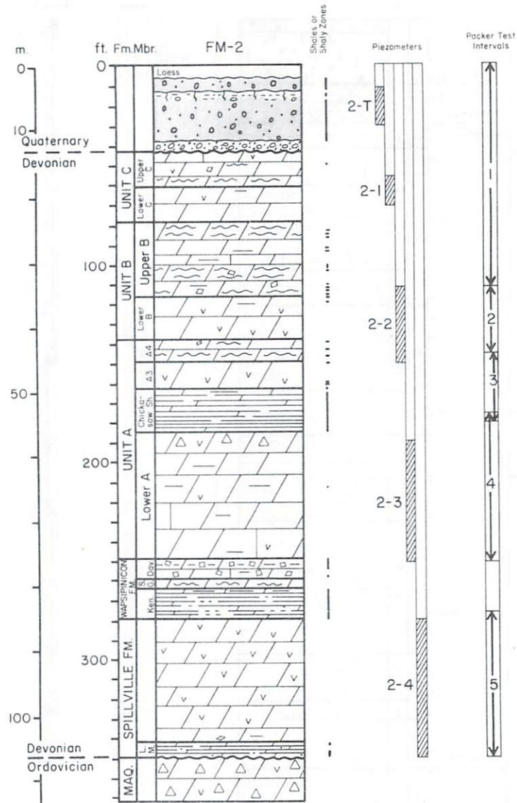
Figure 3. Geologic log, packer-test intervals, and piezometer completions, Site #2.
