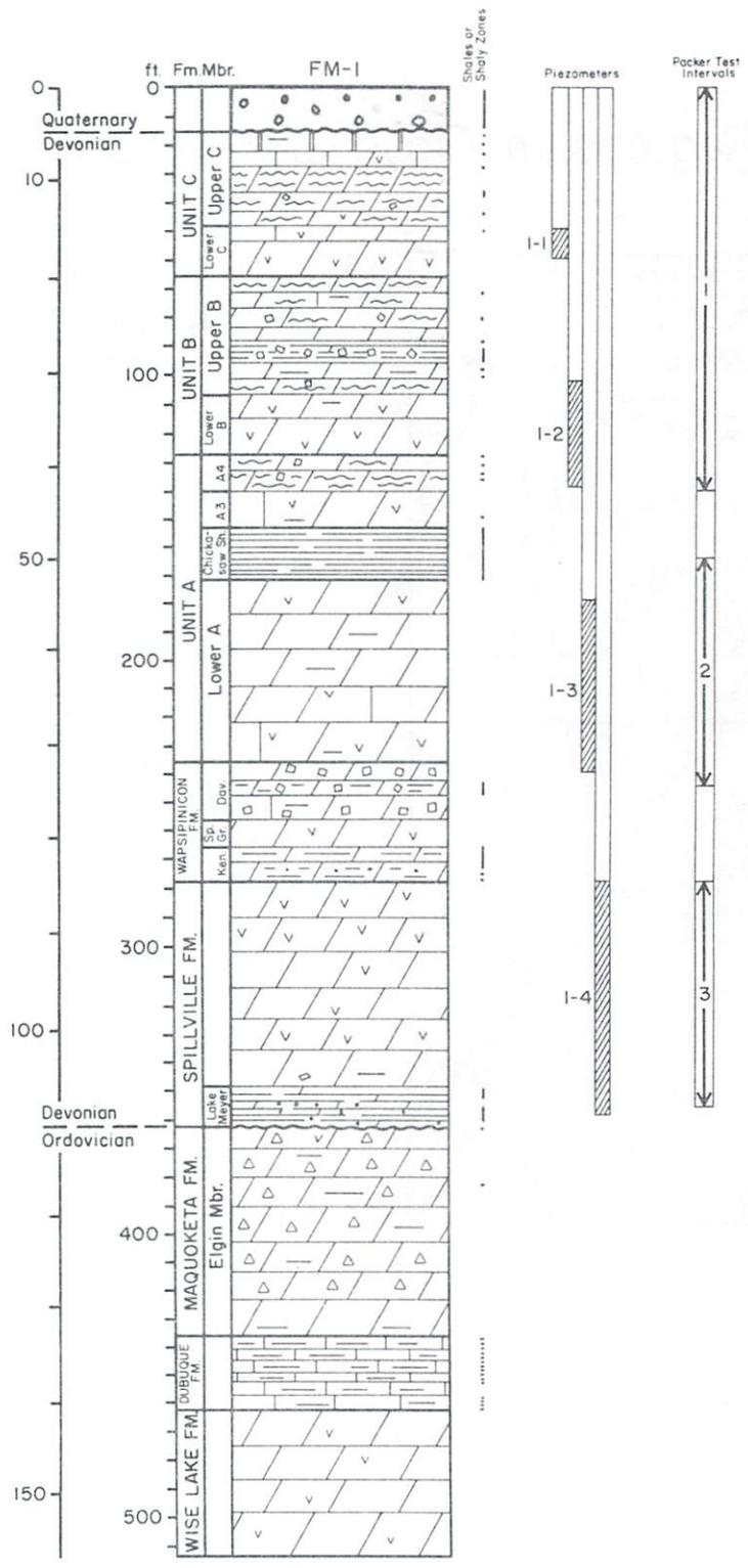
Figure 2. Geologic log, packer-test intervals, and piezometer completions, Site #1.
