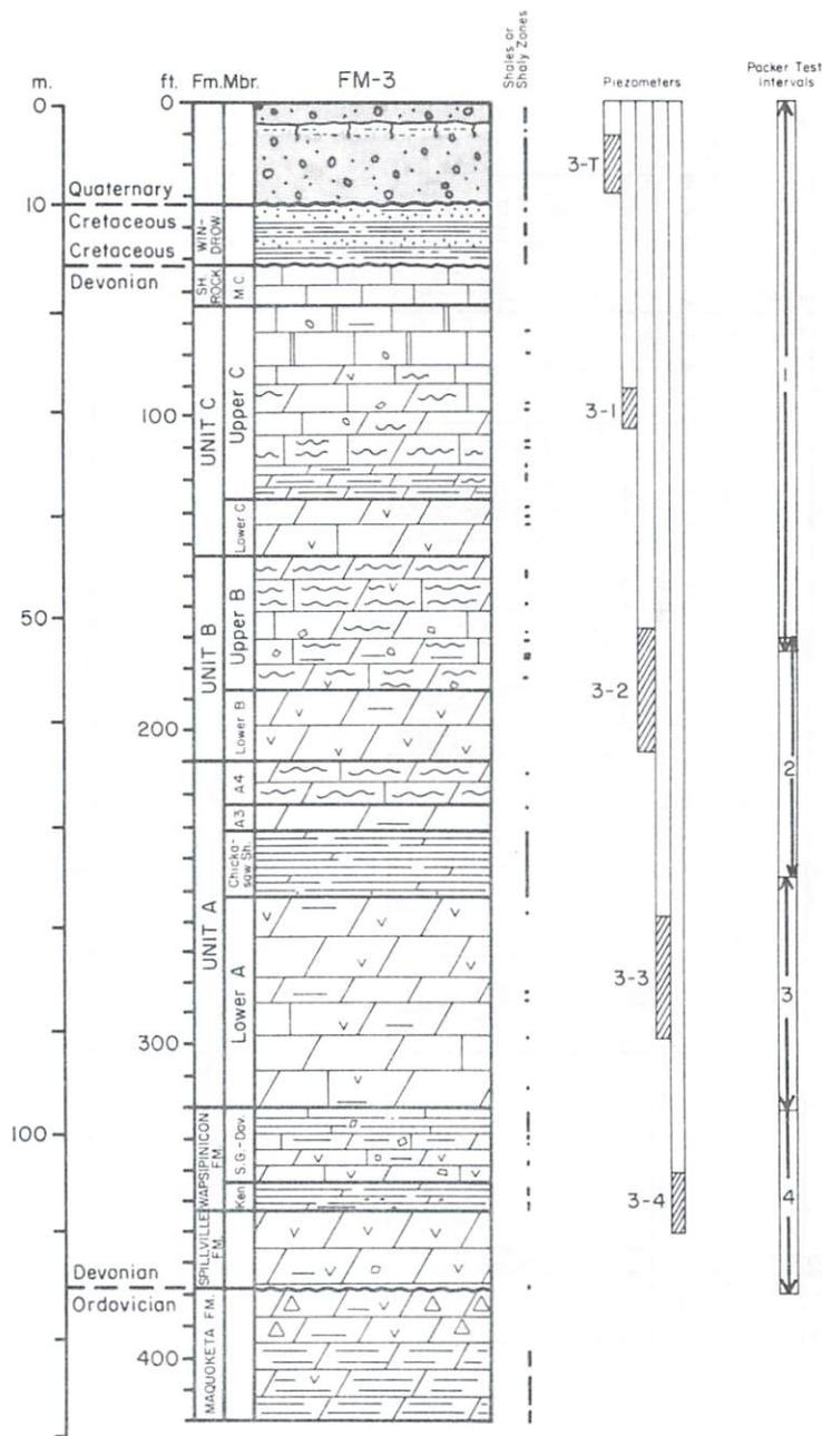
Figure 4. Geologic log, packer-test intervals, and piezometer completions, Site #3.
