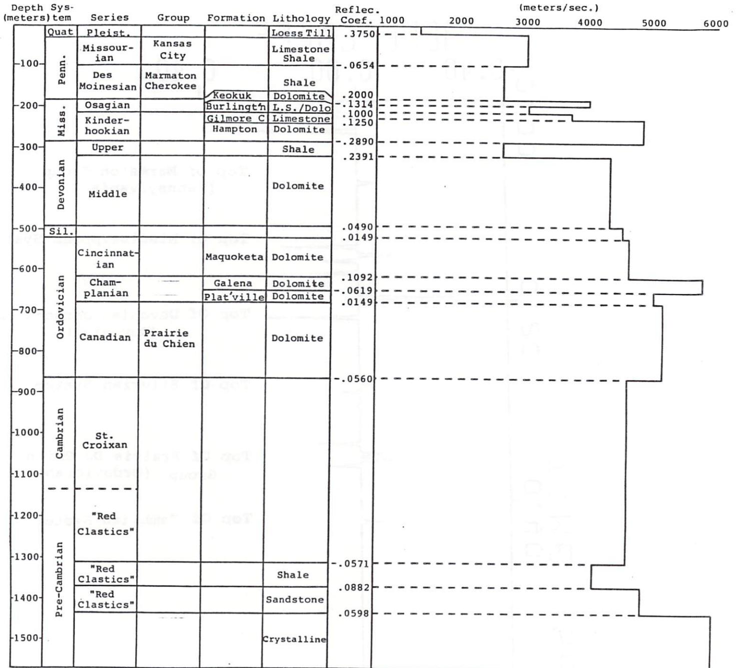
Figure 2. Hypothetical geologic section from Malvern, Iowa, with characteristic velocities, lithologies, and reflection coefficients.
