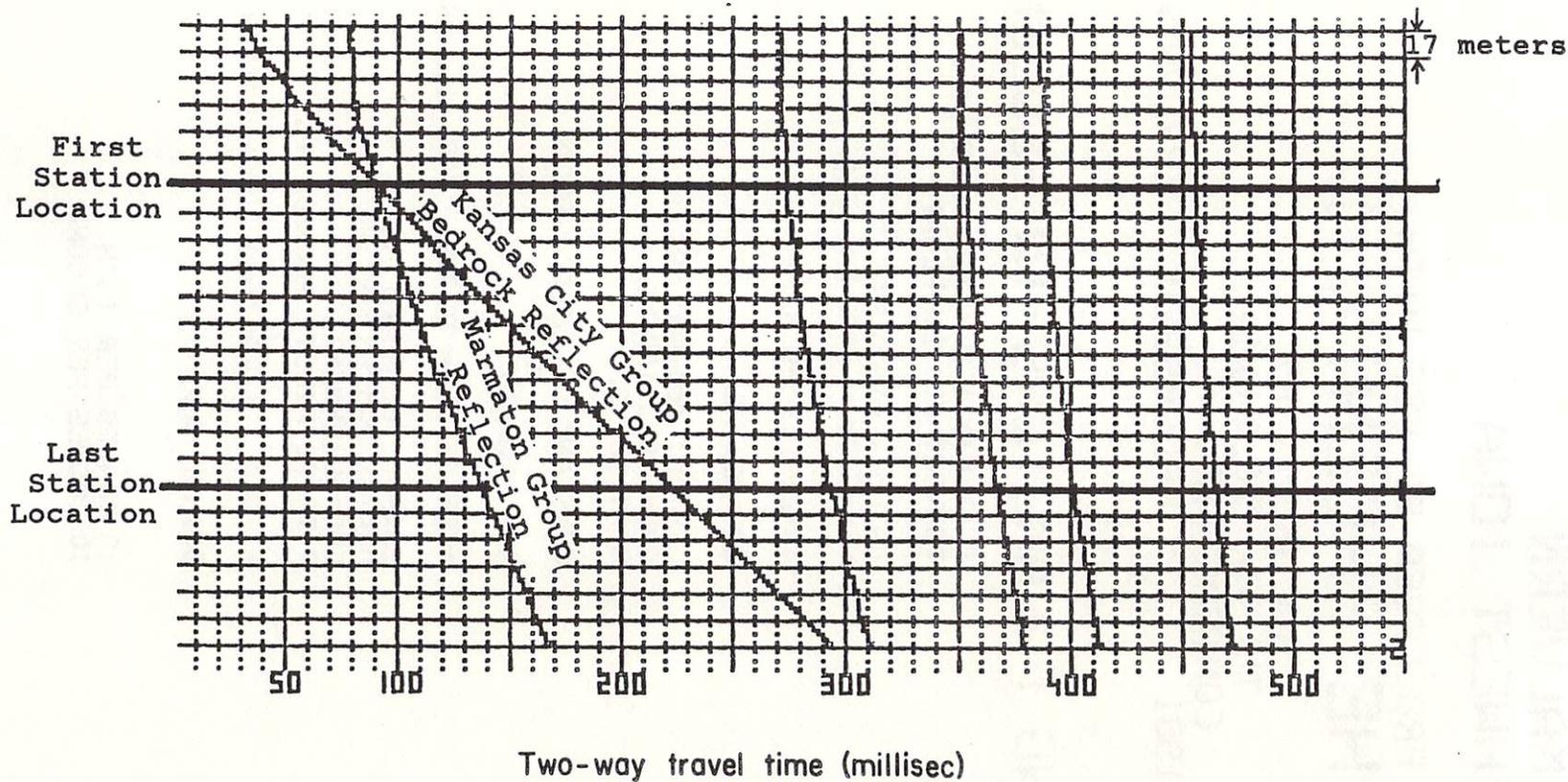
Figure 7. Synthetic field seismogram demonstrating why bedrock reflection does not appear on record sections.
