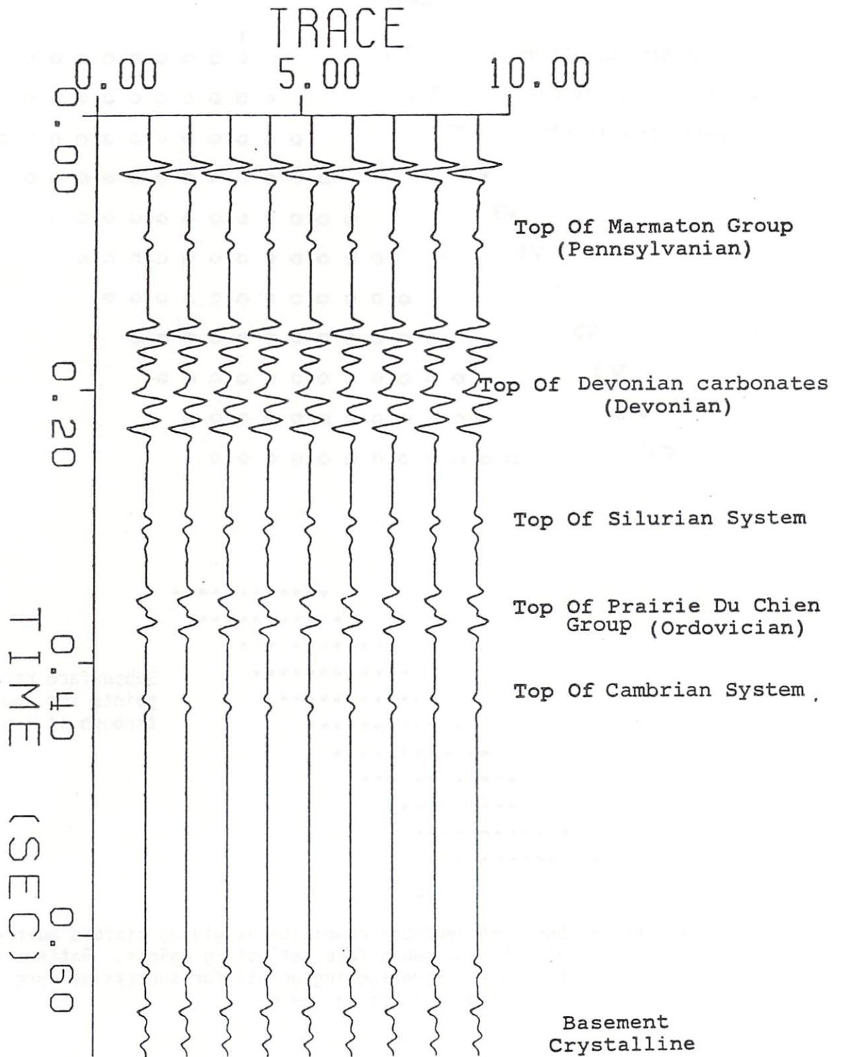
Figure 4. Synthetic seismogram for Malvern model.
