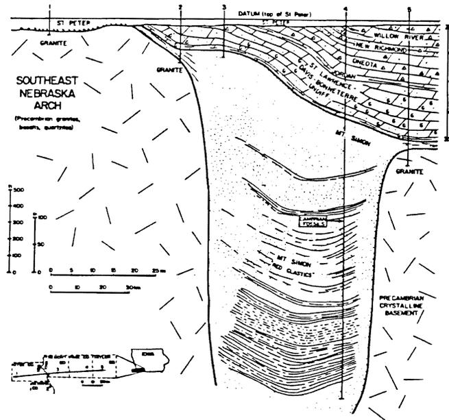
Figure IV-3. Stratigraphic cross-section across southwestern Iowa. Top of St. Peter Sandstone (Middle Ordovician) is used as the stratigraphic datum. Cross-section is used courtesy of Brian Witzke, Iowa Geological Survey.
