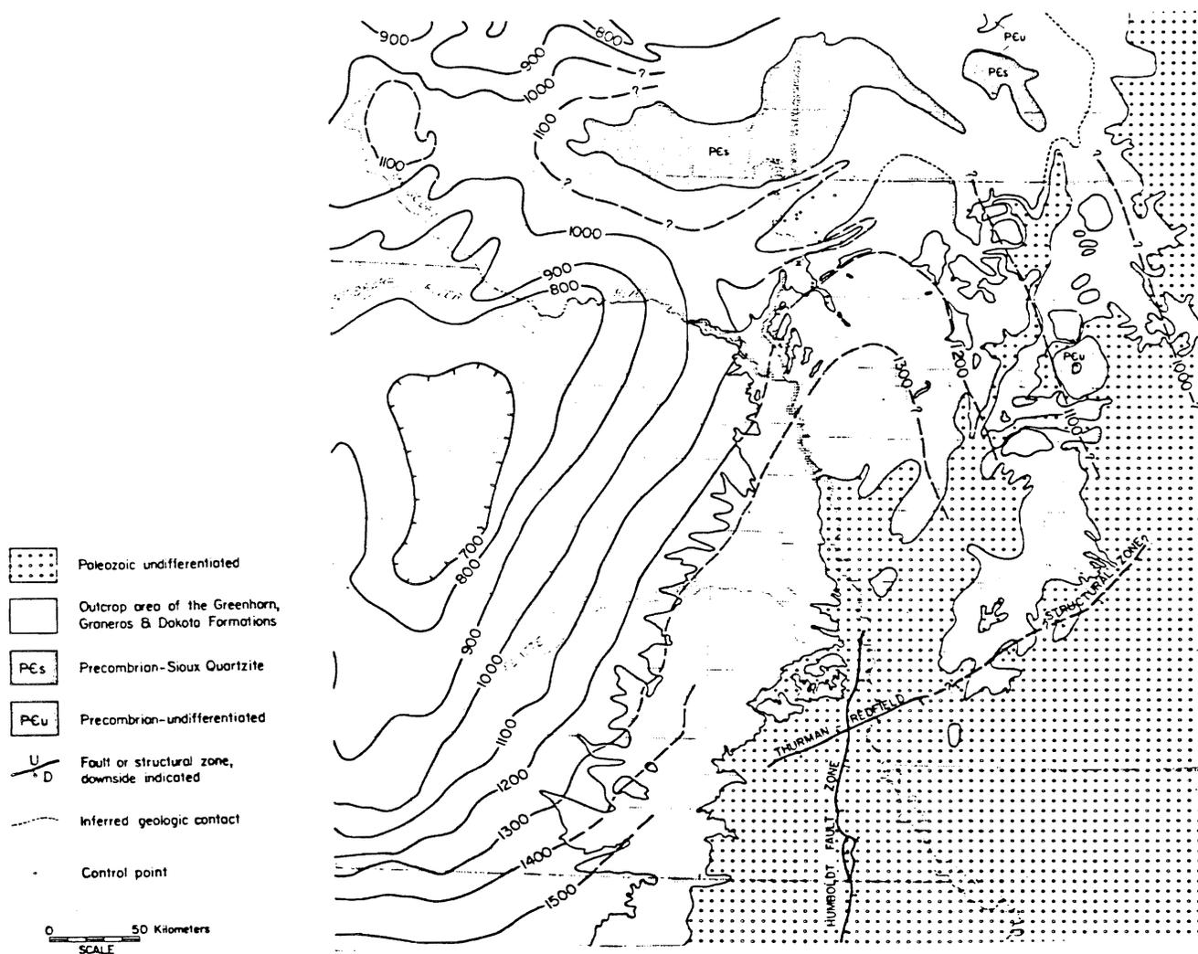
Figure IV-9. Structure contour map on top of the Greenhorn Limestone (Upper Cretaceous) (modified from Bunker, 1981b, p. 16).
