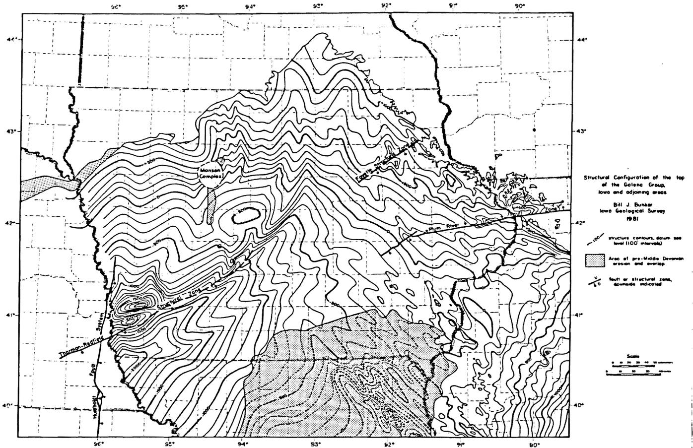
Figure IV-11. Structure contour map on top of the Galena Group (Middle Ordovician) of Iowa and parts of adjoining states (modified from McQueen et al., 1961; Bristol and Buschbach, 1973).
