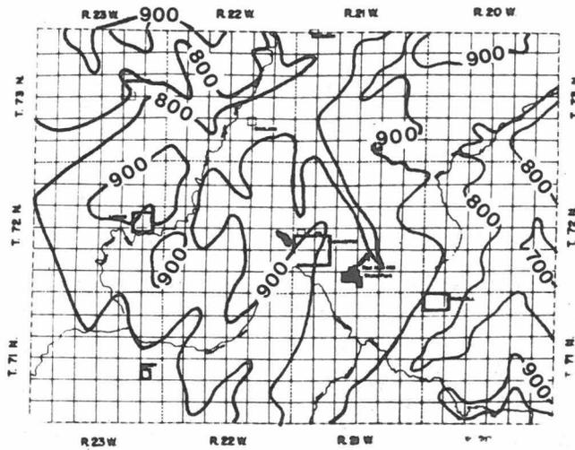
Elevation of the top of the Pennsylvanian Aquiclude in feet above mean sea level
