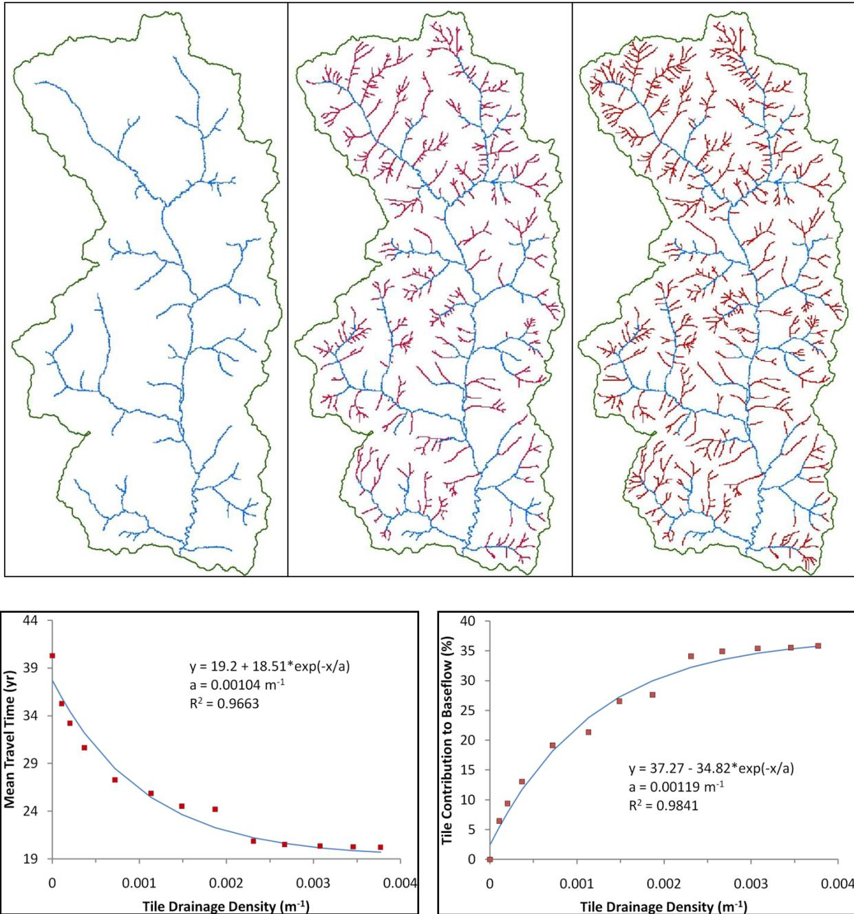
**Figure 3-4:** Hypothesized extent of tile drainage along grass waterways in Walnut Creek watershed (top middle). No drainage way tiling (top left) and maximum tile drainage extent (top right) were included as end members in modeling simulations. Increasing tile drainage density decreases mean travel time (bottom left) and increases tile flow contribution to baseflow (bottom right) (modified from Jindal, 2010 and Schilling et al., 2011).
