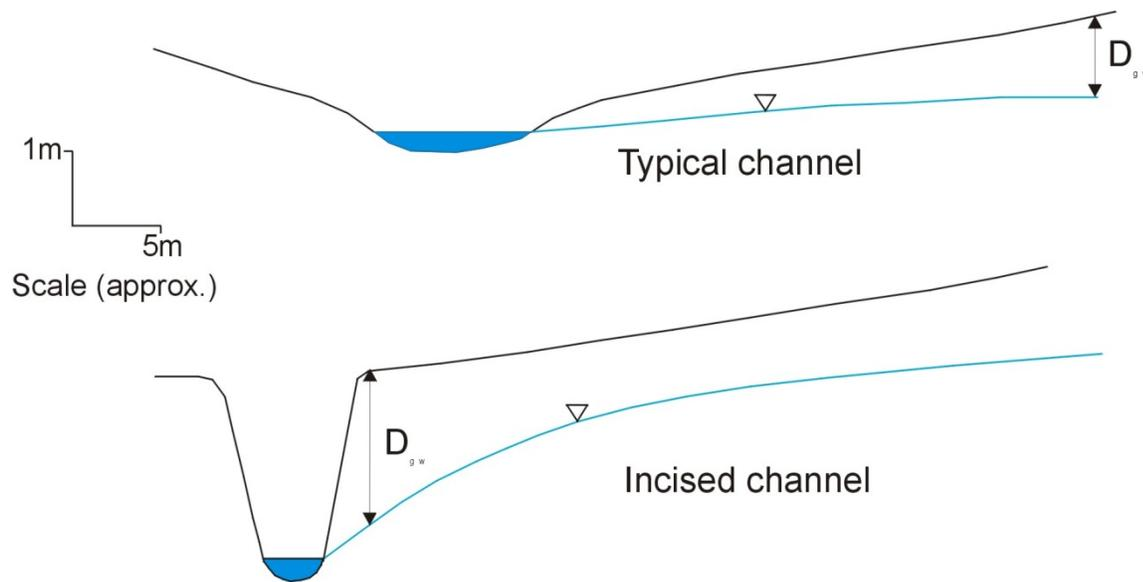
**Figure 3-11:** Comparison of riparian depth to groundwater ( $D_{gw}$ ) in a typical floodplain and near an incised channel. Note how  $D_{gw}$  is greatest near the incised channel.
