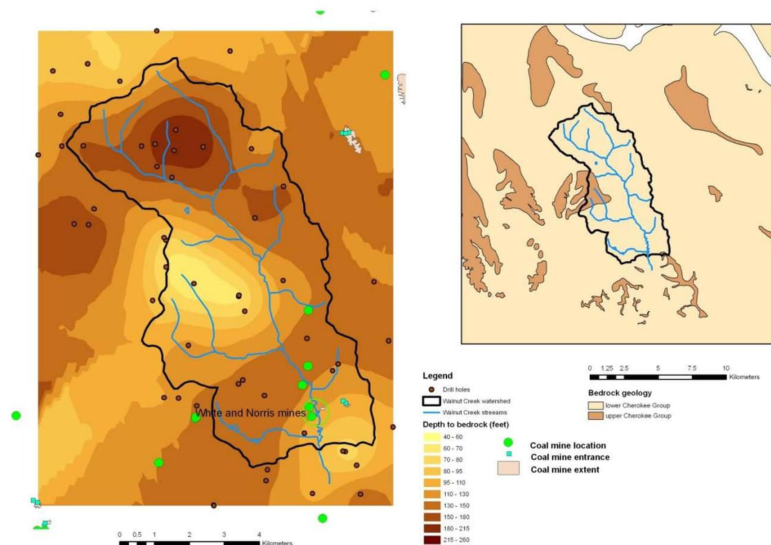
**Figure 2-1:** Bedrock geology and depth to bedrock surface in Walnut Creek watershed.
