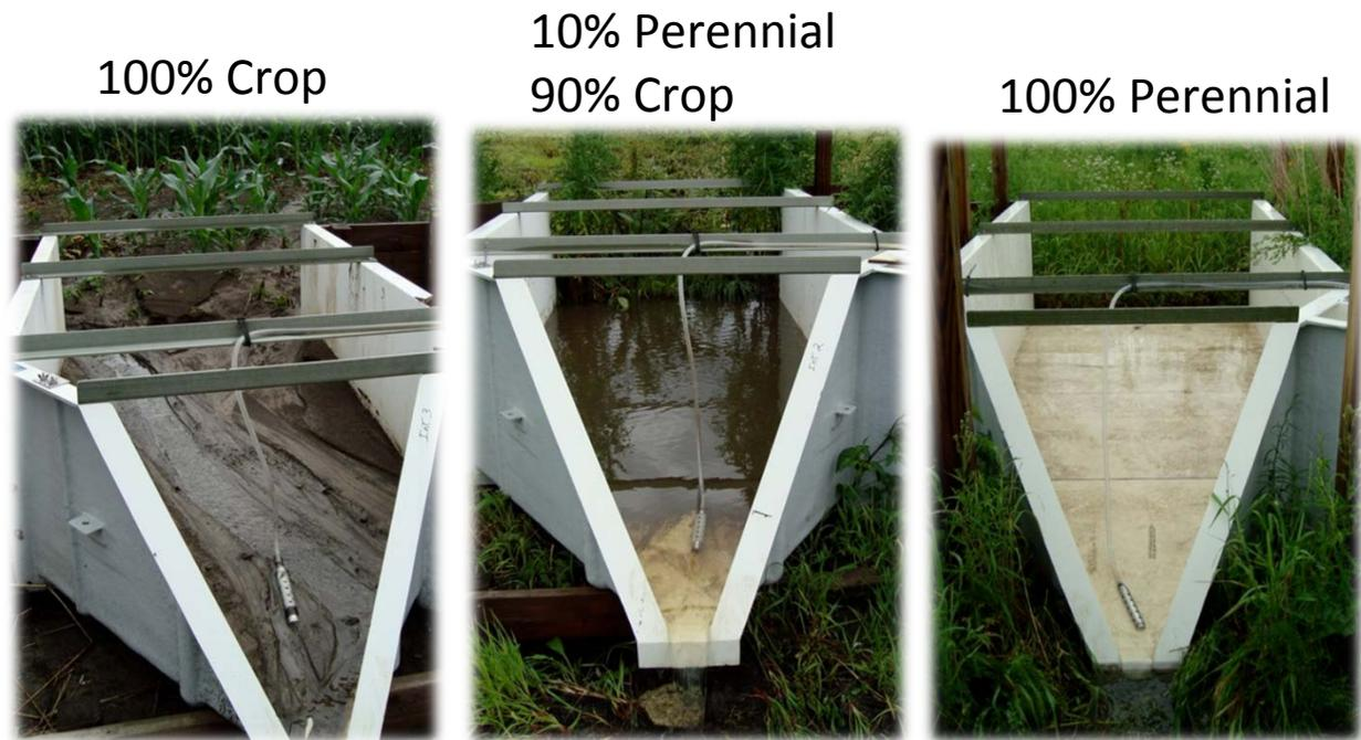
**Figure 4-4:** Visual examples of sediment loss from three small catchments in Walnut Creek watershed after a four-inch rainfall event in June 2008. The 10% perennial catchment had reconstructed prairie planted at the catchment outlet.
