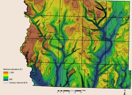
Elevation of the bedrock surface in the northwest Iowa study area. Bedrock channels appear as dark green and blue linear features.
