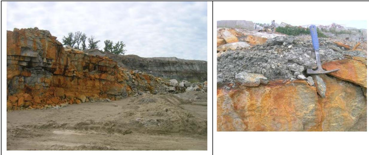
**Figure 7.** Two examples of the extensive staining from oxidation of pyrite at Klein Quarry
