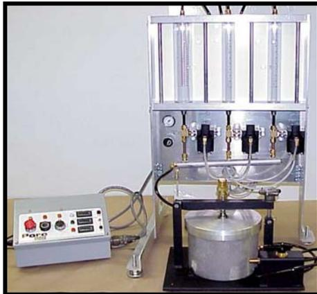
Figure 5. Iowa Pore Index Apparatus.
