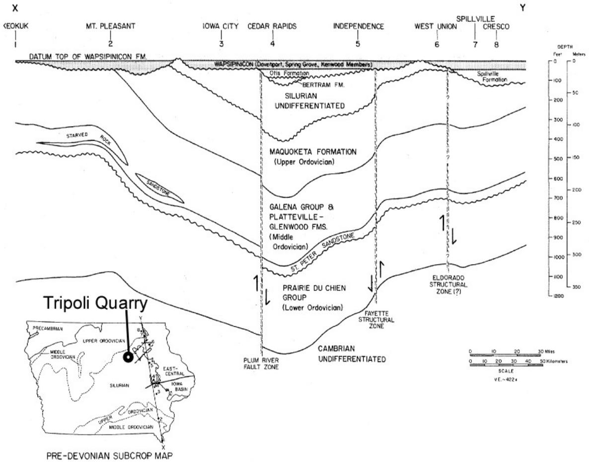
**Figure 2.** Main fault systems known in eastern Iowa shown in the north-south cross-section with the top of the Wapsipicon Group as the datum. The location of the Tripoli Quarry is shown at the western terminus of a projected fault system associated with the Fayette structural zone. After fig. 31 of Bunker and others (1984).
