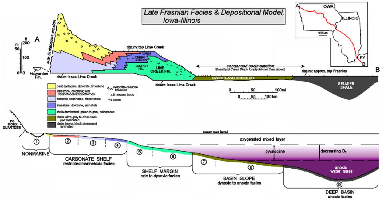
**Fig. 15.**—Regional cross-section and depositional model for Late Frasnian Lime Creek – Sweetland Creek shelf to basin system in the Iowa and deeper water setting in the Illinois Basin. Figure by Witzke.
