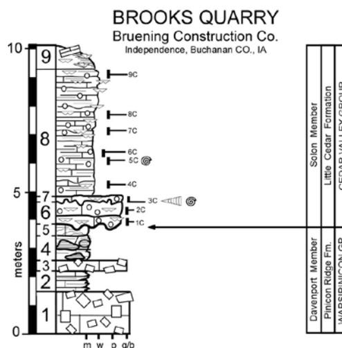
**Figure 1.** Brooks Quarry composite section measured and compiled by Dr. Jed Day. Three main facies of the Solon Member are evident. Unit 6 is a basal transgressive limestone unit, capped by the Brooks Hardground Bed (Unit 7). Unit 8 is a sparsely fossiliferous mudstone. A brachiopod and trilobite producing limestone marks the transition into the coralline limestone beds of Unit 9. See Table 1 for Faunal List from Units.
