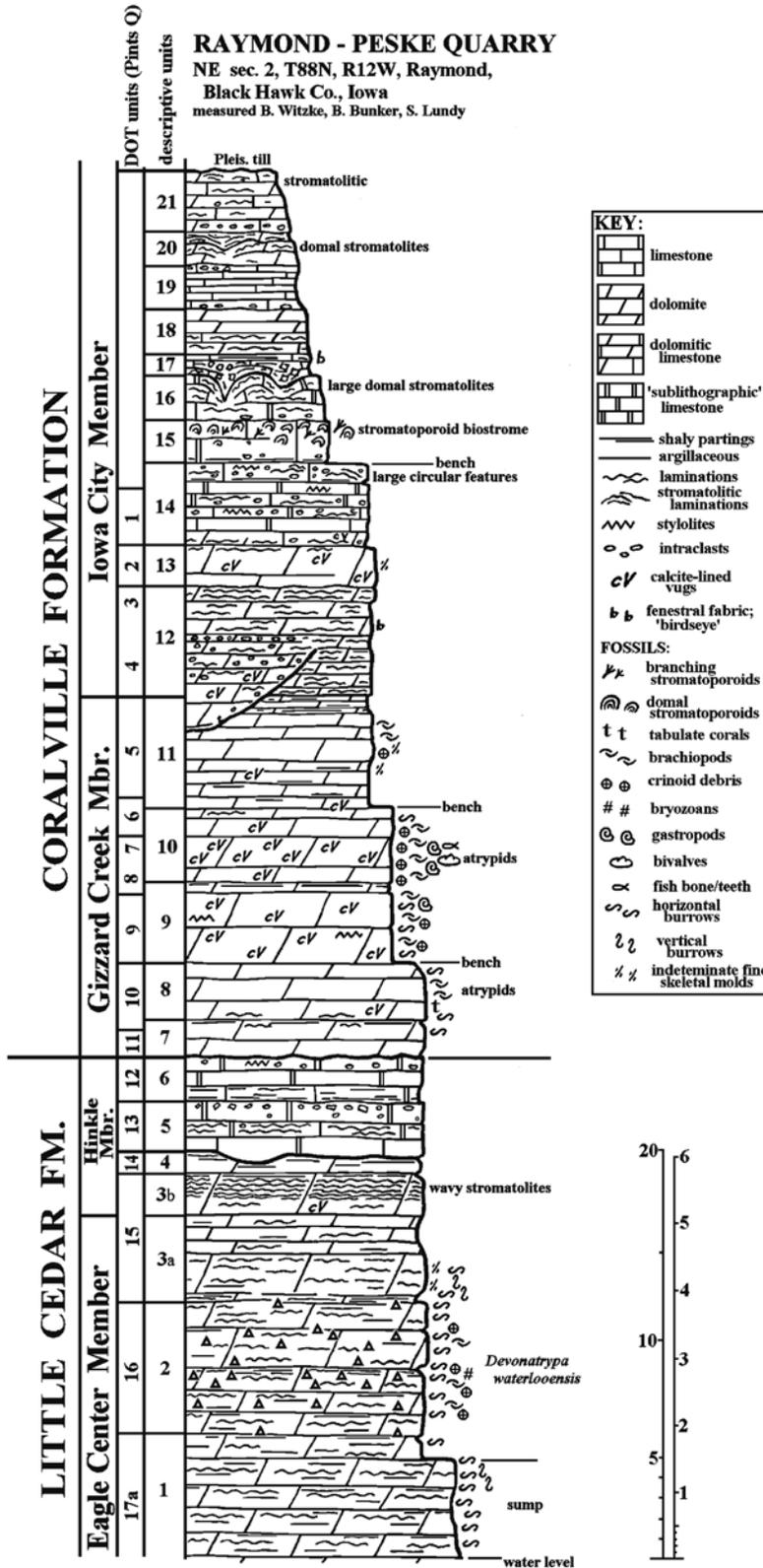
Figure 3. Stratigraphic section of Cedar Valley Group strata exposed in the Basic Materials Corporation's Raymond Quarry. Measured by B. Witzke, B. Bunker, and S. Lundy. After figure 5 of Anderson (1996).
