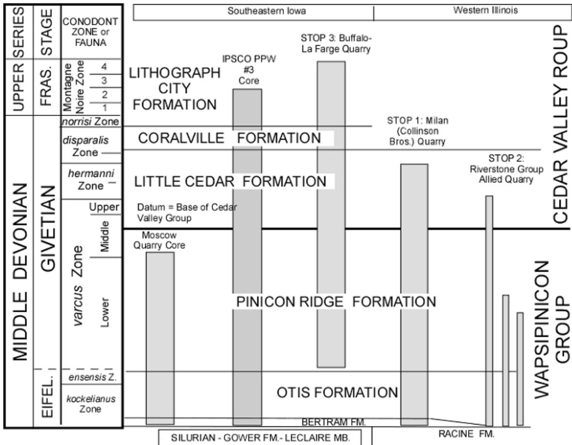
**Figure 1.** Chart showing Silurian and Devonian Wapsipinicon and Cedar Valley Group stratigraphic units exposed in quarries and present in cores shown in Stop Descriptions. At the Allied Quarry (Stop 2) the longest column is the generalized stratigraphic section and the two shorter columns are the 671 and 67-2 core sections. The IPSCO PPW # 3 and 67-1 and 67-2 cores will be on display for inspection in the Field Conference banquet hall.
