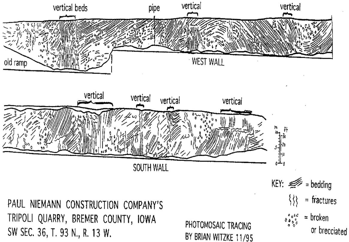
**Figure 6.** Diagram showing the structural relationships of Silurian Hopkinton Formation strata exposed in the south and west walls of the Tripoli Quarry in 1995. After fig. 5 of Anderson (1996).
