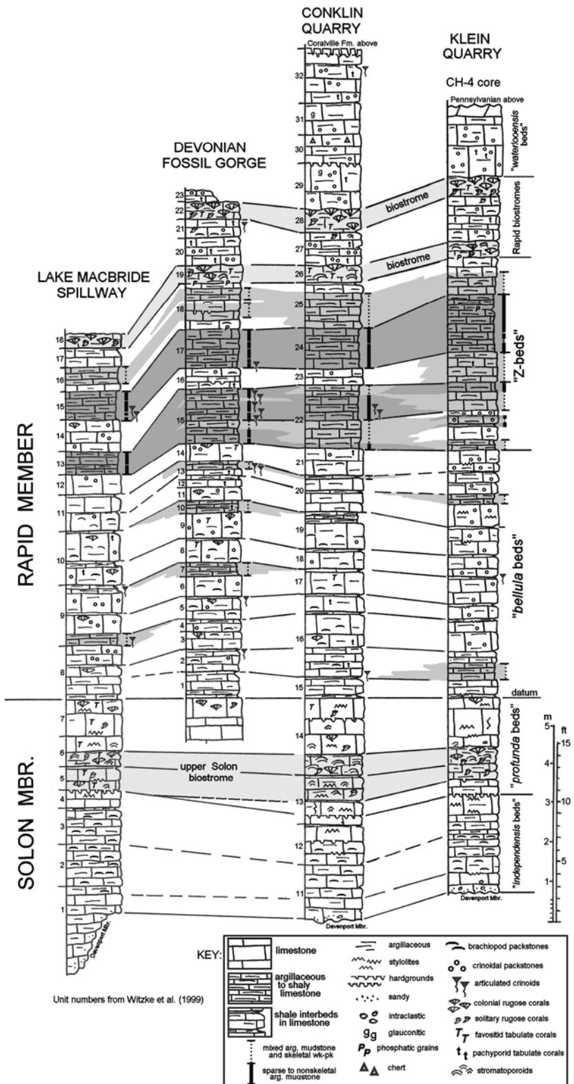
**Figure 4.** Representative graphic stratigraphic sections of Little Cedar Formation in Johnson County, Iowa. Darker shading corresponds to intervals of sparse skeletal to nonskeletal argillaceous mudstone and mixed mudstone with wackestone-packstone. Positions of Solon and Rapid biostromes shown in lighter shading.
