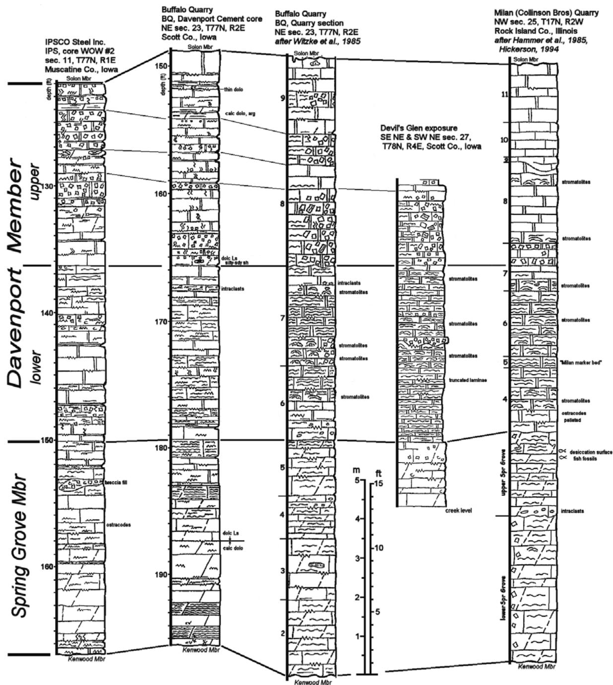
**Figure 4.** Representative graphic sections of upper Wapsipinicon Group strata in the Quad Cities area, Iowa and Illinois. Symbols as in Figures 1 and 2. IPSCO and Buffalo Quarry cores are stored at the Iowa Geological Survey. Milan Quarry section adapted from Hammer and others (1985) and Hickerson (1994). The natural exposure at Devil's Glen is here designated the type locality of the Davenport Member. Symbols as noted for Figures 1 and 2. Cores are archived at the Iowa Geological Survey.
