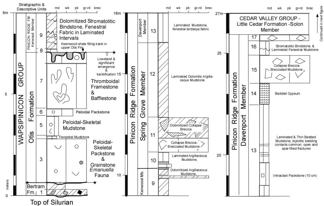
**Figure 6.** Stratigraphy of the Wapsipinicon Group in the IPSCO PPW # 3 core from Muscatine County, Iowa. Arrows at major discontinuities denote positions of major marine flooding surfaces and define T-R cycle boundaries. Arrow within the Otis Formation shows the position of the minor flooding event of Otis Formation 4<sup>th</sup> Order T-R cycle 2. Location: SW NE SW Sec. 15, T. 77 N., R. 1 E.
