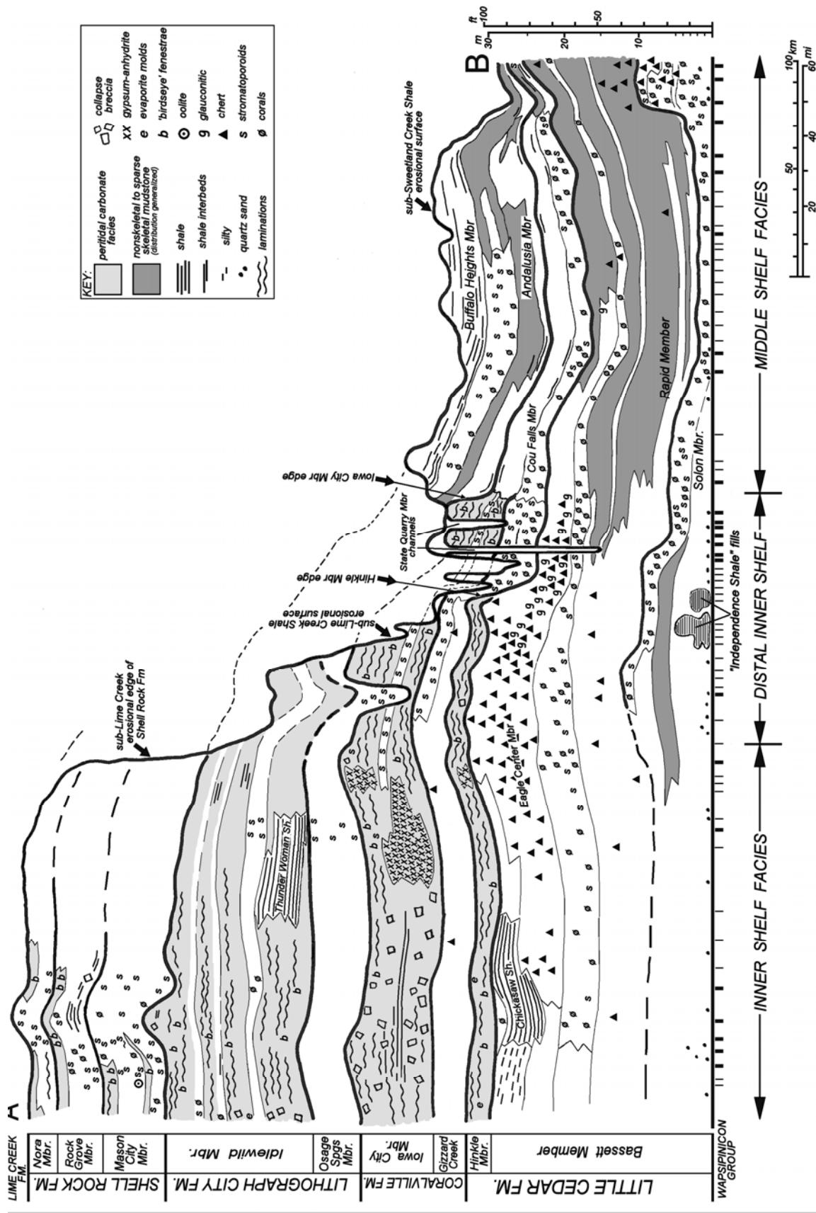
**Figure 2.** Northwest-southeast stratigraphic cross section of the Cedar Valley Group in eastern Iowa. Significant sub-Lime Creek/Sweetland Creek erosion has truncated Cedar Valley strata, especially in the distal inner-shelf area. "Independence Shale" fills represent stratigraphic leaks of Lime Creek Shale within Cedar Valley karst networks and openings. See Figure 1 for location of cross-section line (AB) and data points used in the construction.
