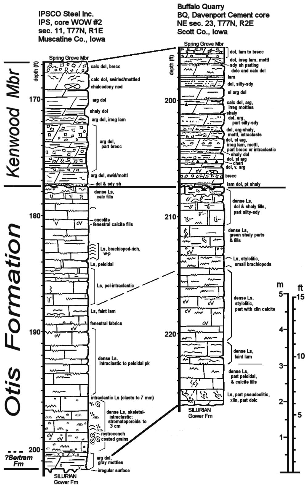
**Figure 3.** Graphic sections of lower Wapsipinicon Group strata from two cores in southeastern Iowa. Symbols as noted for Figures 1 and 2. See Figure 5 in the accompanying Cedar Valley Group article for explanation of abbreviations. Cores are archived at the Iowa Geological Survey.
