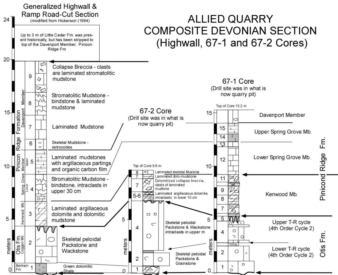
**Figure 5.** Stratigraphy and Devonian T-R cycles developed in the Wapsipinicon Group in the highwall section and cores 67-1 and 67-2 from the Allied Quarry, Rock Island County, Illinois. Locations given in Stop 2 discussion.
