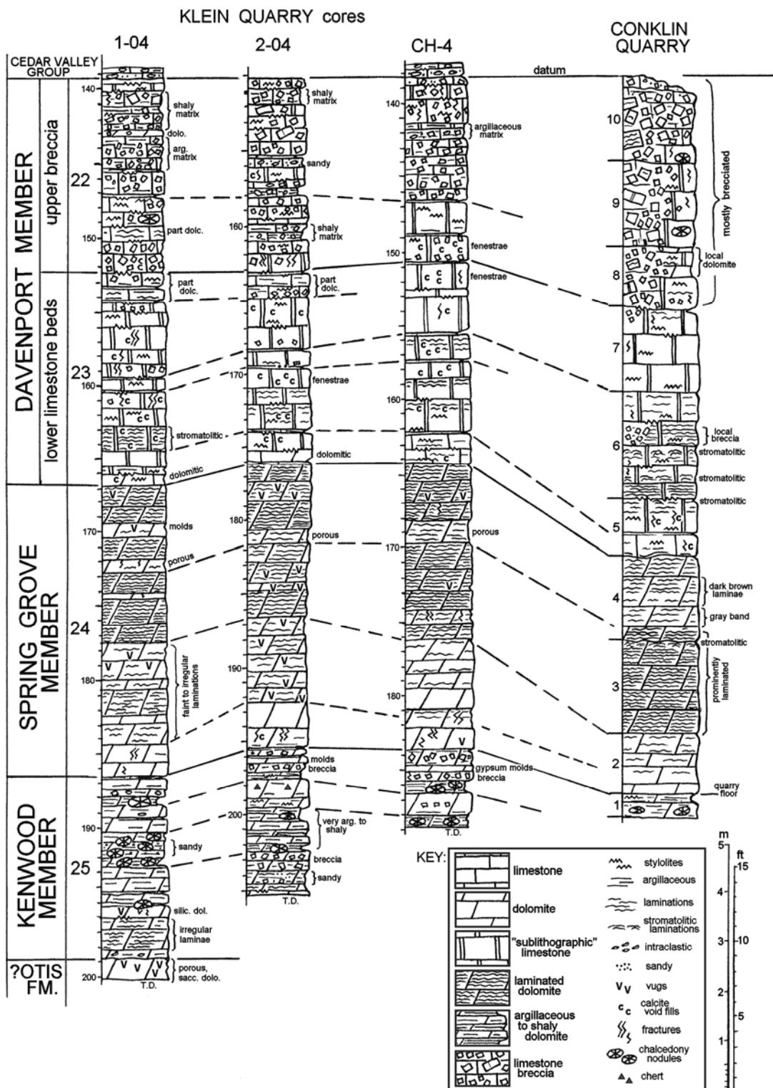
**Figure 1.** Graphic stratigraphic sections, Wapsipinicon Group, Johnson County, Iowa. Closely spaced core sections from the Klein Quarry are shown to illustrate lithologic variations within the constituent members over short lateral distances (<1 km). Conklin Quarry section adapted from Witzke and others (1999). Cores stored at the Iowa Geological Survey; core depths in feet.
