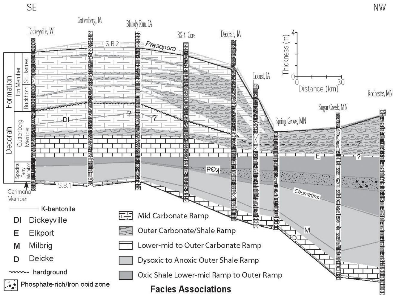
**Figure 10.** Facies associations distributions and correlation of measured sections along the line shown in Figure 3. Datum is the Elkport K-bentonite. See Figure 3 caption for specific locations of measured sections. See Emerson (2002, appendix-II) for stratigraphic details of the measured sections. See Table 1 for facies association details. S.B.1 and S.B. 2 = sequence boundaries 1 and 2.
