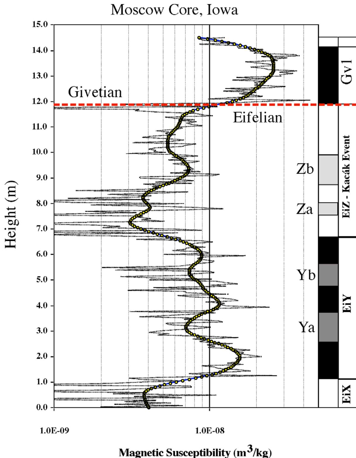
**Figure 10.** MS data for the latest Eifelian Stage from a Moscow Quarry core (Fig. 1, locality MQC). MS data reported as in Fig. 6. MS chronos notation from Fig. 8. Za, Zb, Ya, and Yb are MS subchrons. The Eifelian-Givetian boundary is represented by an unconformity (dashed horizontal line).
