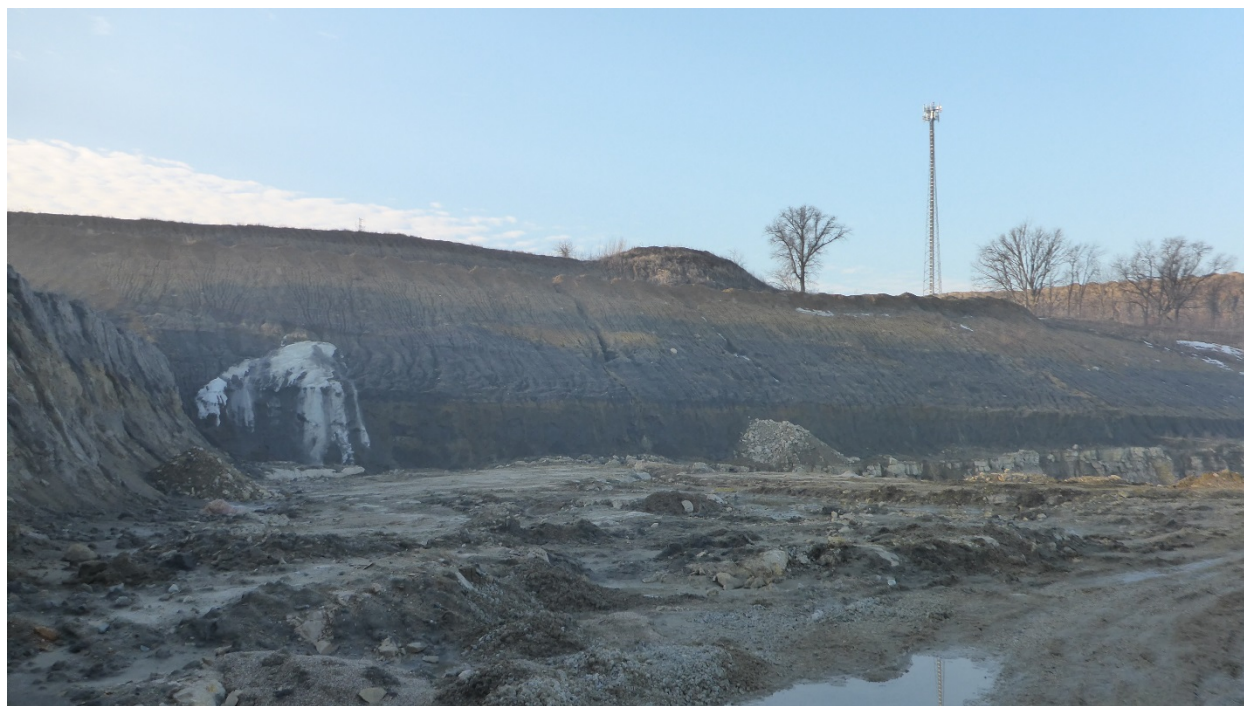
Figure 4. South quarry wall. Note the presence of the till-till contact (dark gray unit overlying brown oxidized unit) and deformed sand body within the till.
