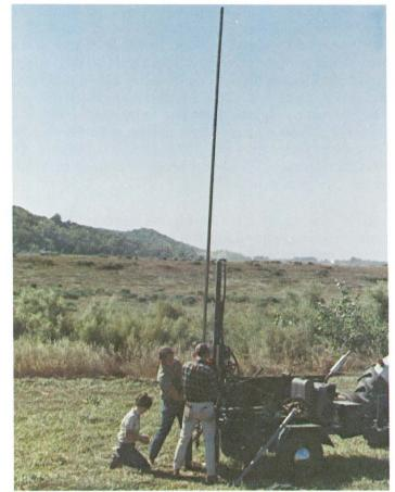
Figure 9. Drilling projects provide information on types of sediments that lie beneath the land surface. Here, along Waubonsie Creek in Fremont County, samples are taken to determine whether the sediments were deposited by the Missouri River, out of the picture to the right, or whether they originated from the loess hills in the background. Photo by James C. Davis.
