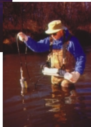
Right: This device measures such water characteristics as pH, dissolved oxygen, and turbidity.
