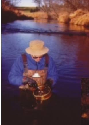
Right: This device measures such water characteristics as pH, dissolved oxygen, and turbidity.
