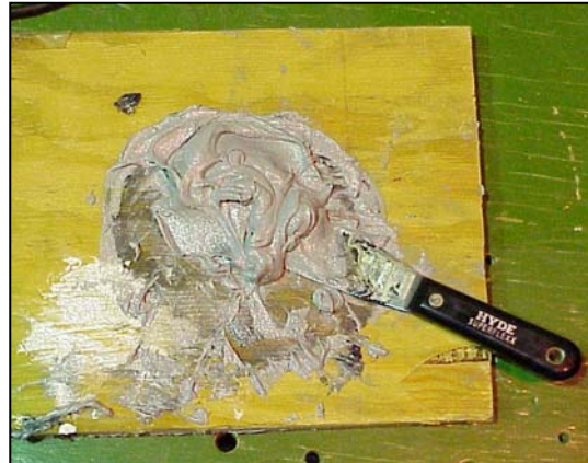
Figure A.16 Blend until an even gray color appears.
