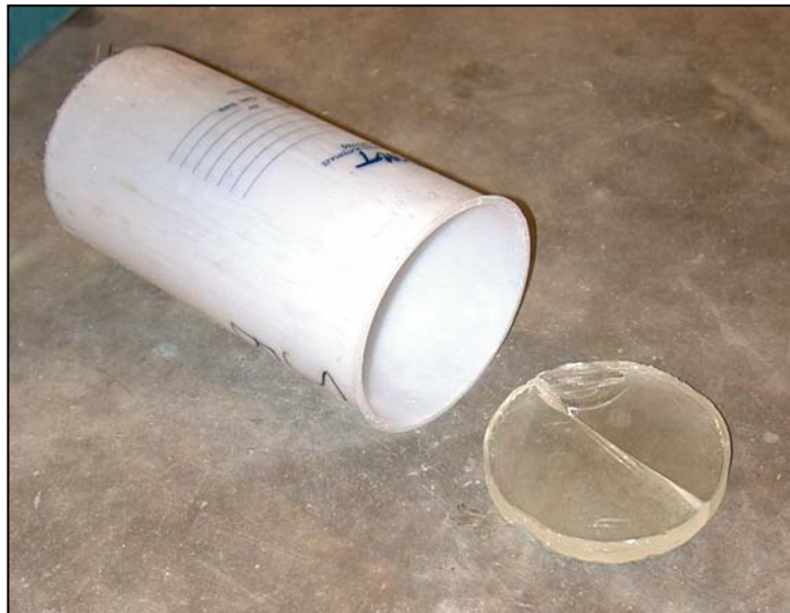
Figure A.32 Let the epoxy set-up overnight and the hardened substance can be removed, allowing the containers to be used again.
