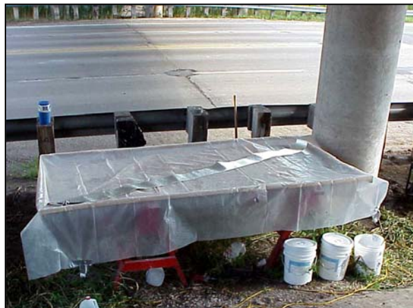
Figure A.20 Create a temporary saturation trough.
