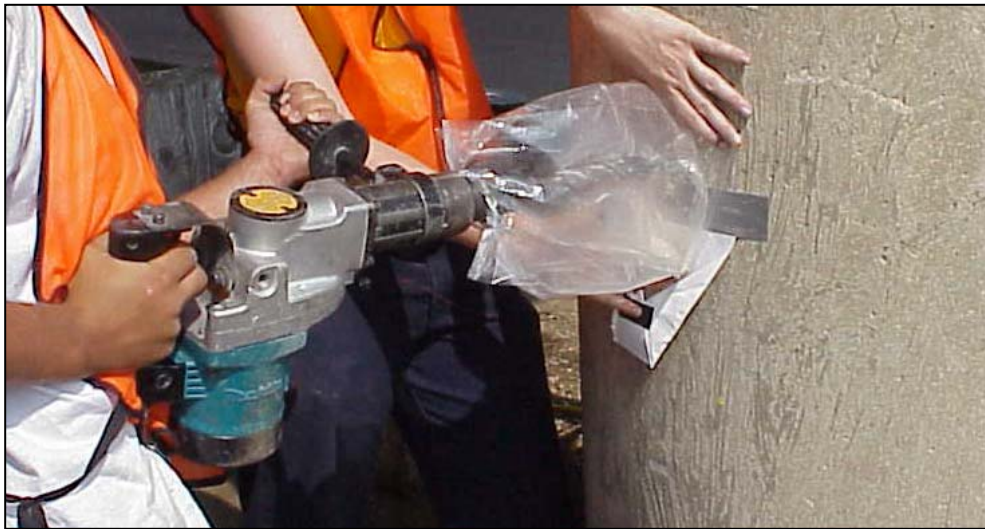
Figure 3.19 Hammer drill and plastic bag utilized in powder collection.
