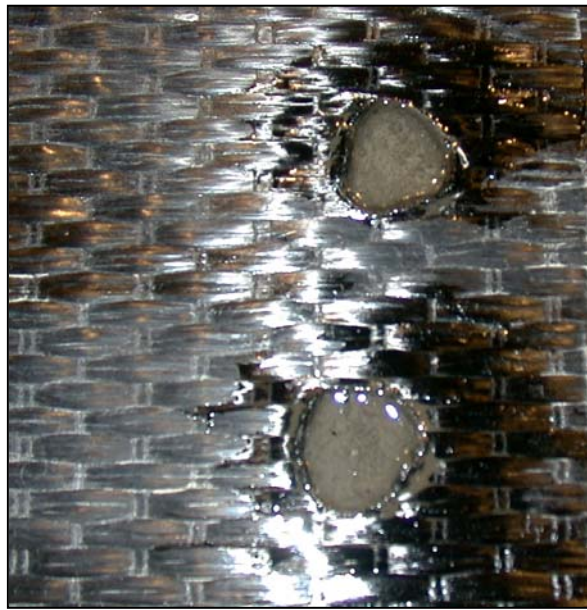
Figure 4.7 Epoxy patched sample stations from the first cycle.
