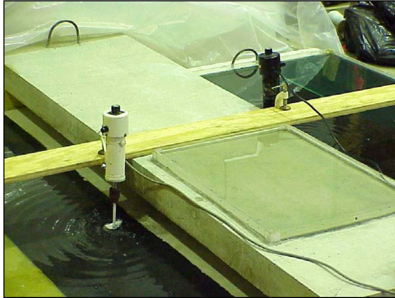
Figure 3.24 Position of the two electric mixers on the stacked slabs.
