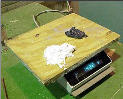
Figure A.15 The putty's main agent and hardener are measured by weight.
