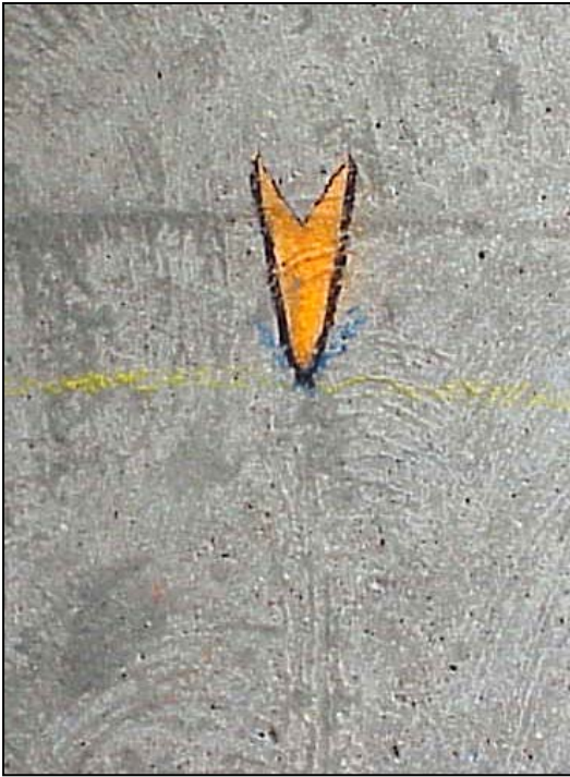
Figure 3.16 One of four locator arrows used to establish the perimeter positions.
