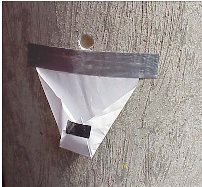
Figure 3.18 Powder collector in place at a sample station.
