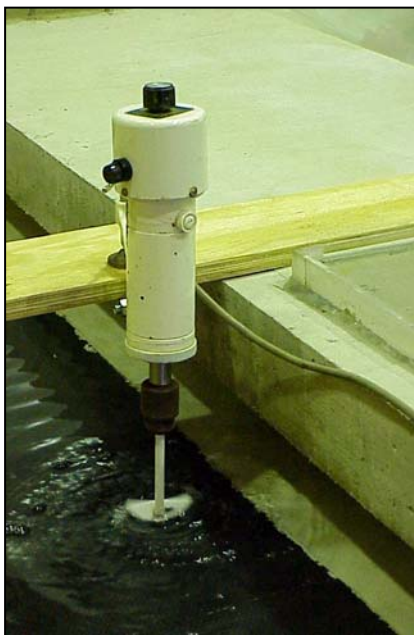
Figure 3.23 Electric mixer with a plastic paddle blade to prevent corrosion.
