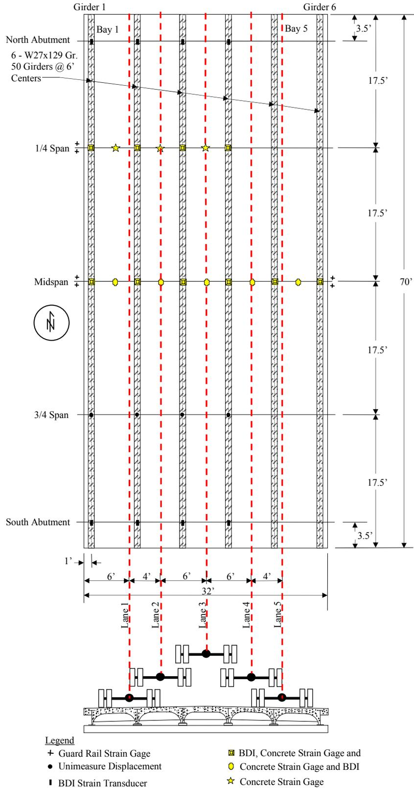
Figure 3.9. Layout of main flexural instrumentation and test vehicle placement for MBISB 2.
