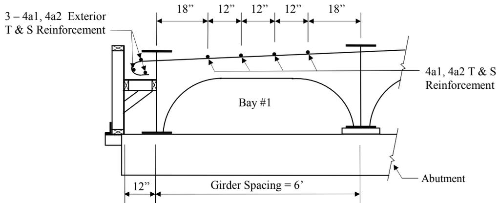
Figure 5.7. Typical layout of the longitudinal T & S reinforcement.
