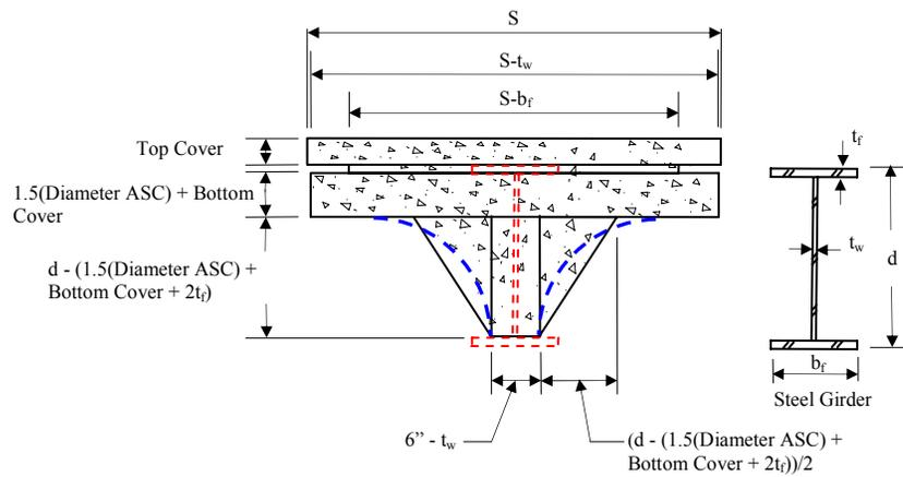
b. Detail A: Approximated interior cross section
