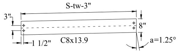
d. Typical layout of C8x13.9 diaphragm section
