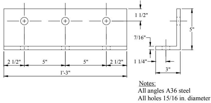
a. Diaphragm connector for C15x33.9 section
