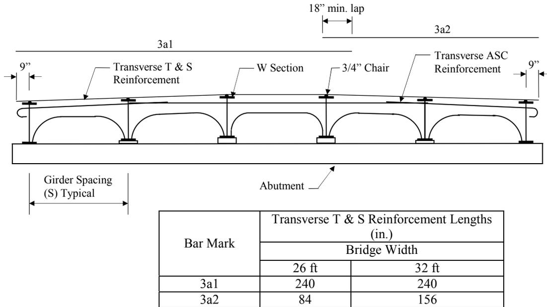
Figure 5.9. Layout of transverse T & S reinforcement.
