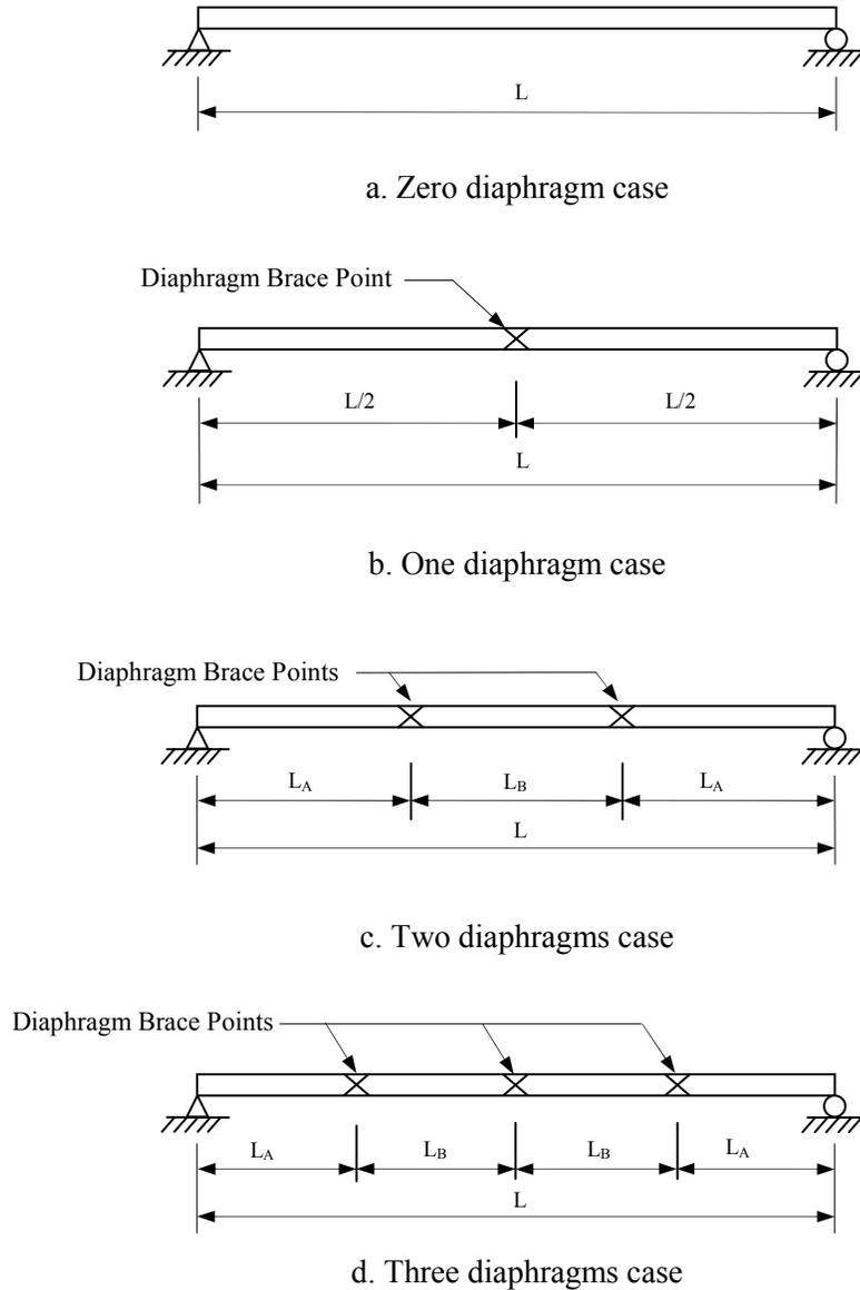
Figure 4.3. Possible diaphragm layouts for the MBISB.
