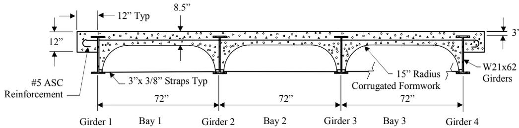
a. Typical transverse cross section of the model bridge
