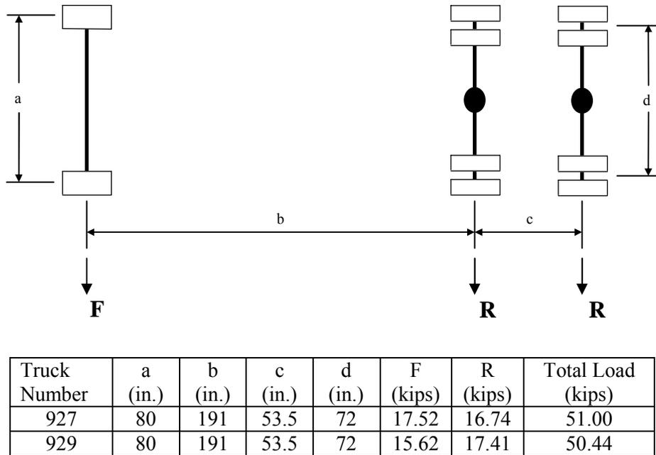
Figure 3.2. Wheel and load configurations for the MBISB 1 test vehicles.
