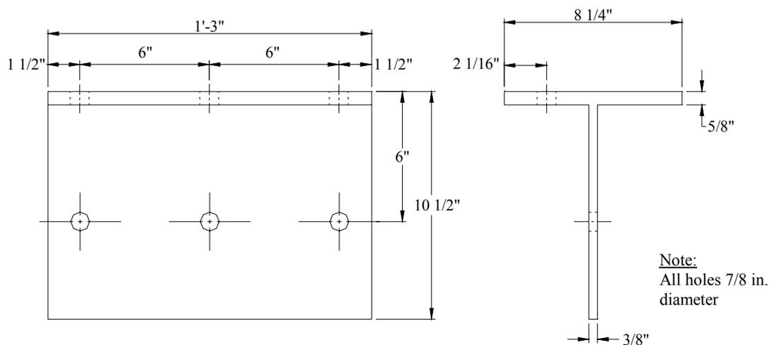
Figure 5.1. Diaphragm connection used in the construction of MBISB 2.
