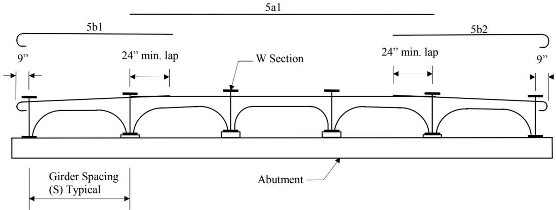
Figure 5.6. Transverse reinforcement for the MBISB design.
