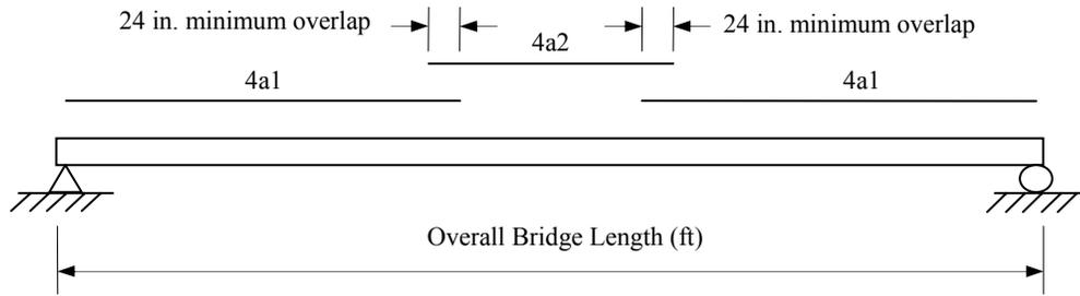
Figure 5.8. Typical longitudinal layout of T & S reinforcement.
