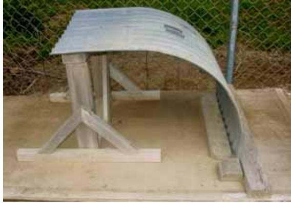
d. Jig with first component in position
