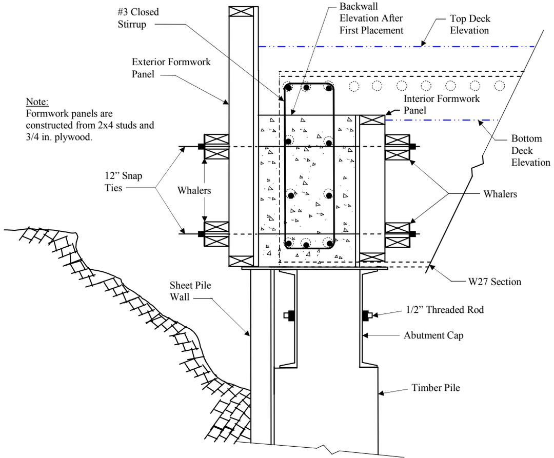
a. Cross section of backwall formwork
