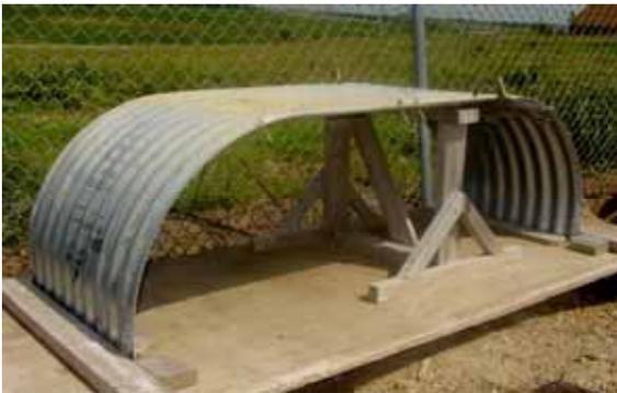
e. Individual components clamped in preparation of drilling the bolt holes
