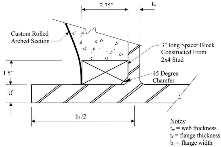
a. Installed spacer block
