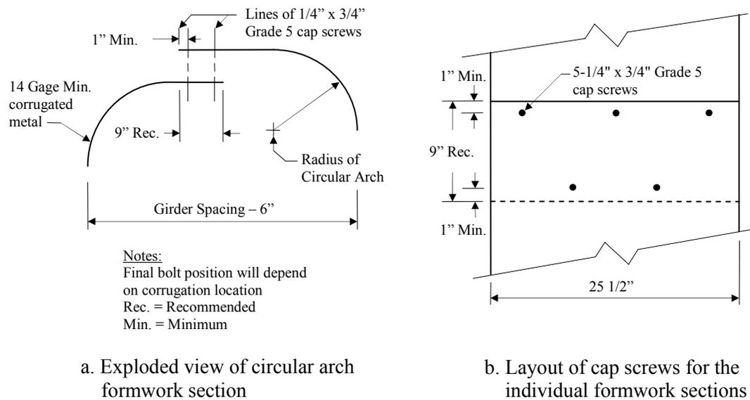
Figure 4.9. Assembly of the individual arched sections.
