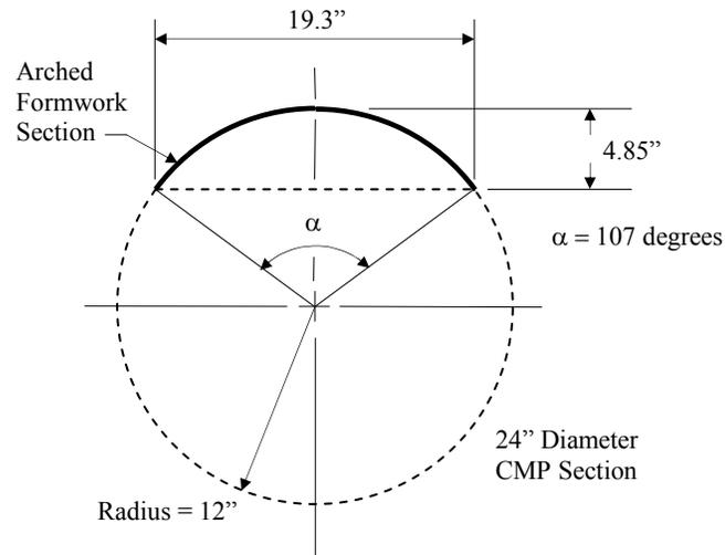
Figure 4.8. Stay-in-place formwork section cut from the 24 in. diameter CMP used in MBISB 1.
