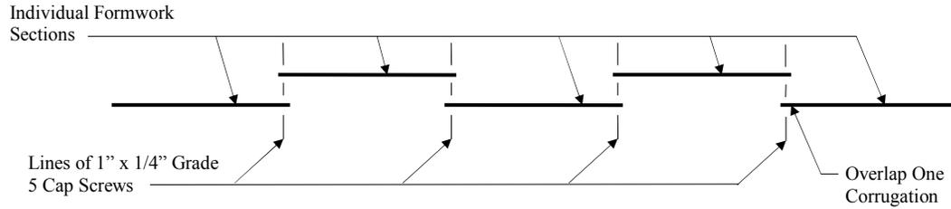
a. Typical 'over/under' battery layout configuration
