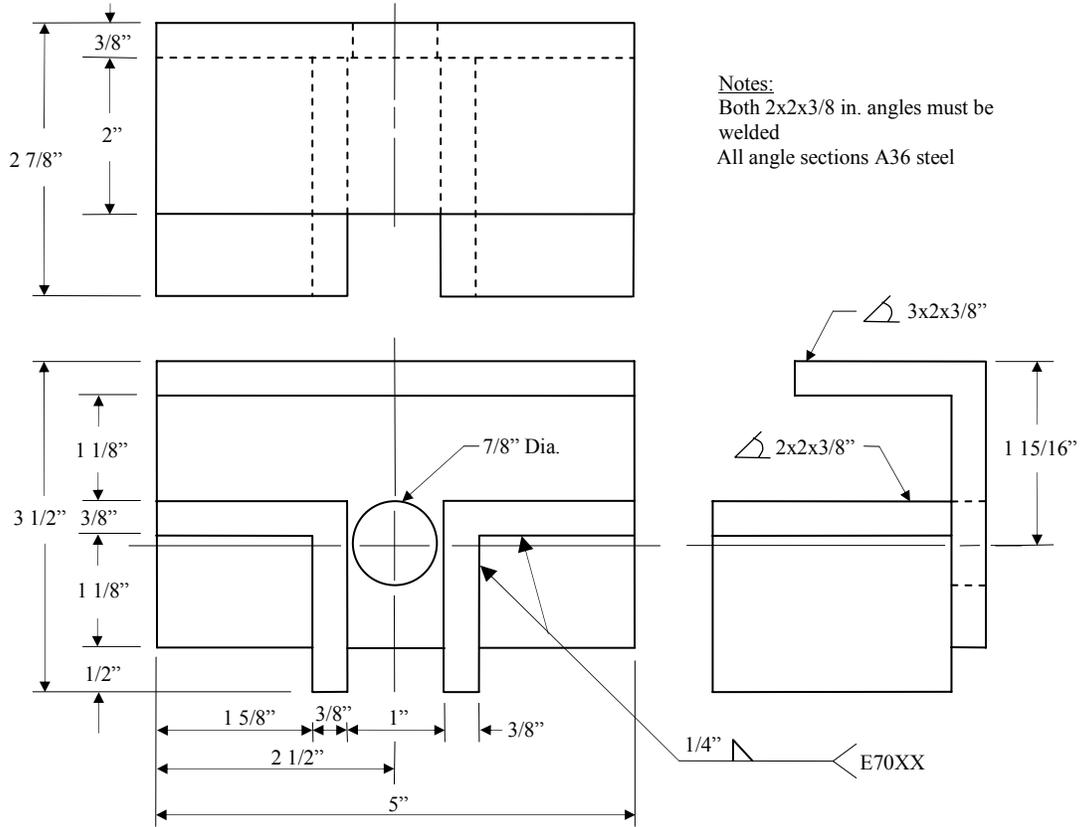
a. Schematic of tension clip
