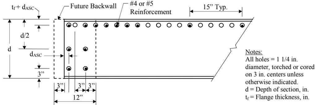
Figure 4.12. Layout of deck reinforcement.
