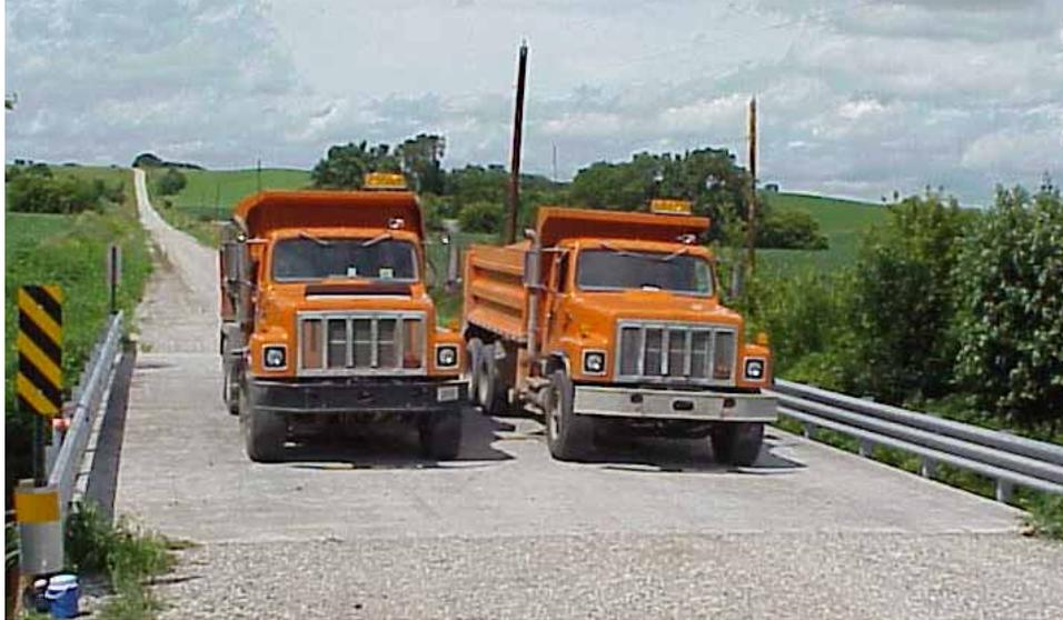
a. Static test 1, test vehicles in Lanes 2 and 4
