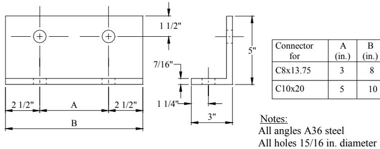
b. Diaphragm connector for C10x20 and C8x13.75 sections
