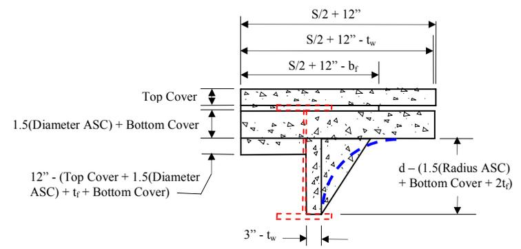
c. Detail B: Approximated exterior cross section
