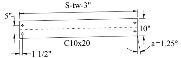
c. Typical layout of C10x20 diaphragm section
