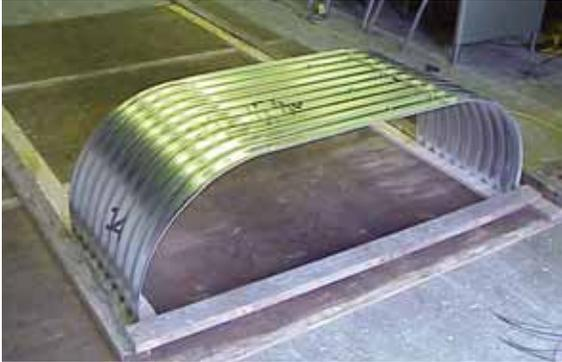
b. Individual arch section fitted in the jig
