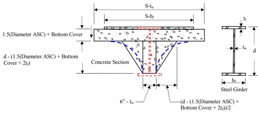
(b) Detail A: Approximated interior cross section
