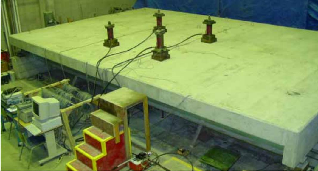
c. Over view of the model bridge during the ultimate flexural loading
