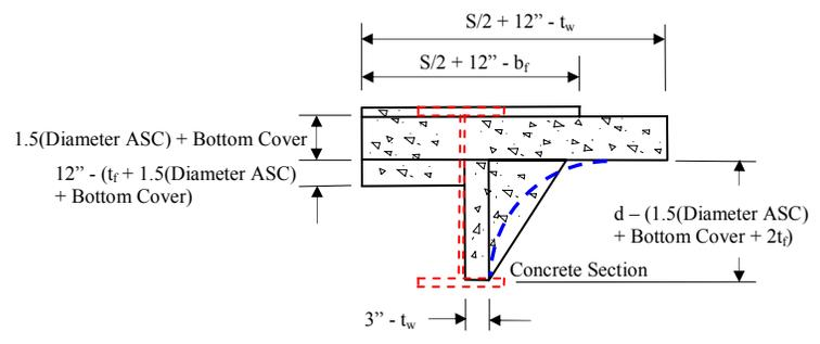
(c) Detail B: Approximated exterior cross section
