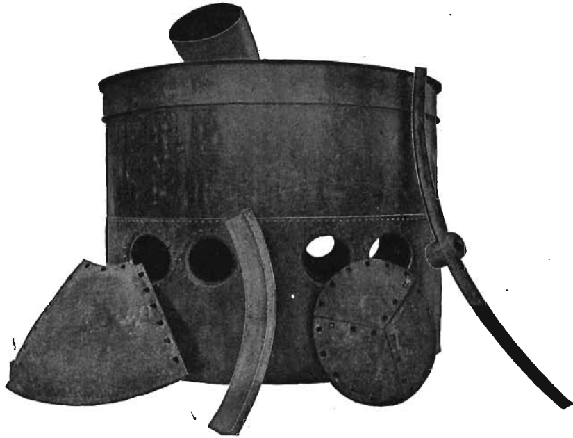
FIG. 39.—Calcining kettle with stirrer, and portions of sectional bottom and lip ring. Courtesy New York Geological Survey.
