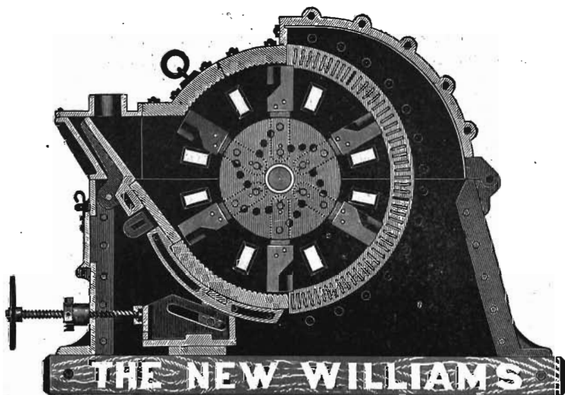
FIG. 36.—A hammer mill. Several mills of this type are on the market and they are sometimes used in gypsum mills for initial crushing and grinding. Courtesy New York Geological Survey.
