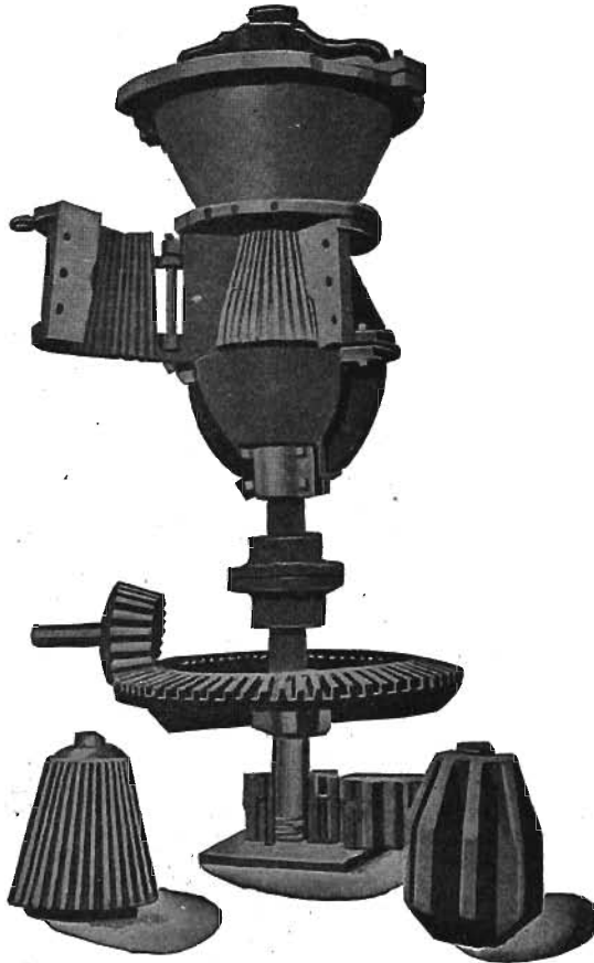
FIG. 33.—Cone crusher or cracker which is commonly used in gypsum mills to further reduce the product coming from the jaw crusher. Courtesy of New York Geological Survey.
