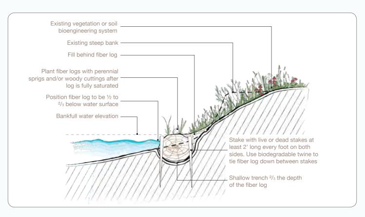
**Figure 4B-6.** Stream Edge Protection with Coconut Logs
