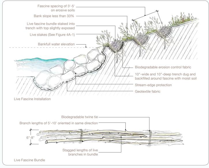
Figure 4B-5. Stream Edge Protection with Live Fascine
