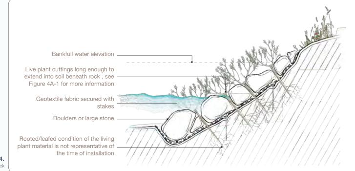
Figure 4B-4. Stream Edge Protection Using Rock
