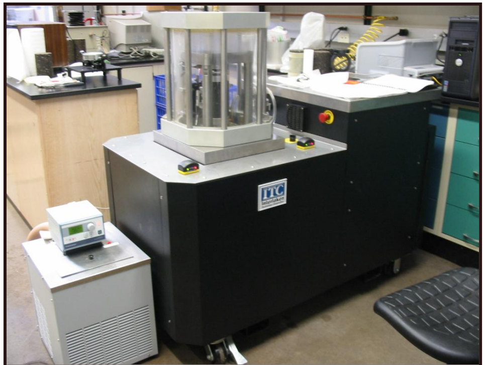
CIR-emulsion mixtures tested using an Interlaken Gyratory Compactor Photo: Dr. Hosin "David" Lee, The University of Iowa/IIHR
