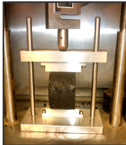
Indirect tensile strength test setup
