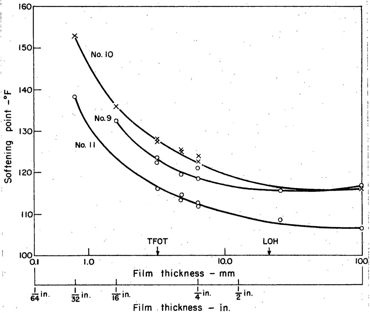
Fig. 10. Softening point vs film thickness.
