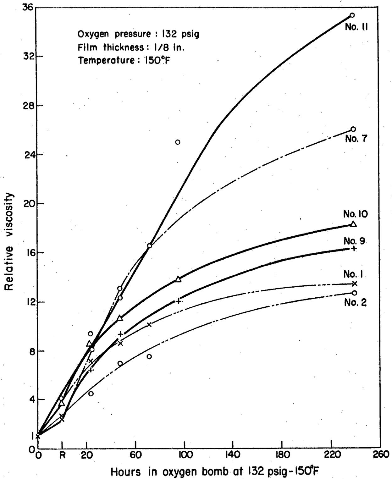
Fig. 5. Relative viscosity vs time of aging.
