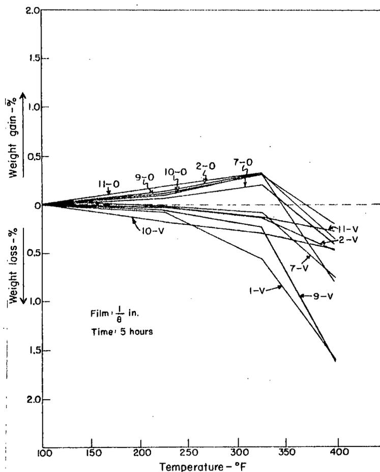
Fig. 25. Weight change vs temperature.
