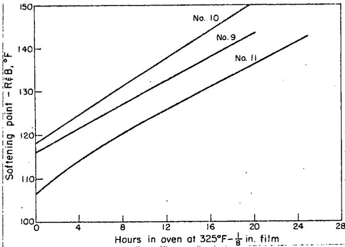
Fig. 16. Softening point vs heating time.
