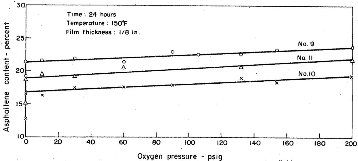
Fig. 9. Effect of oxygen pressure on asphaltene content.
