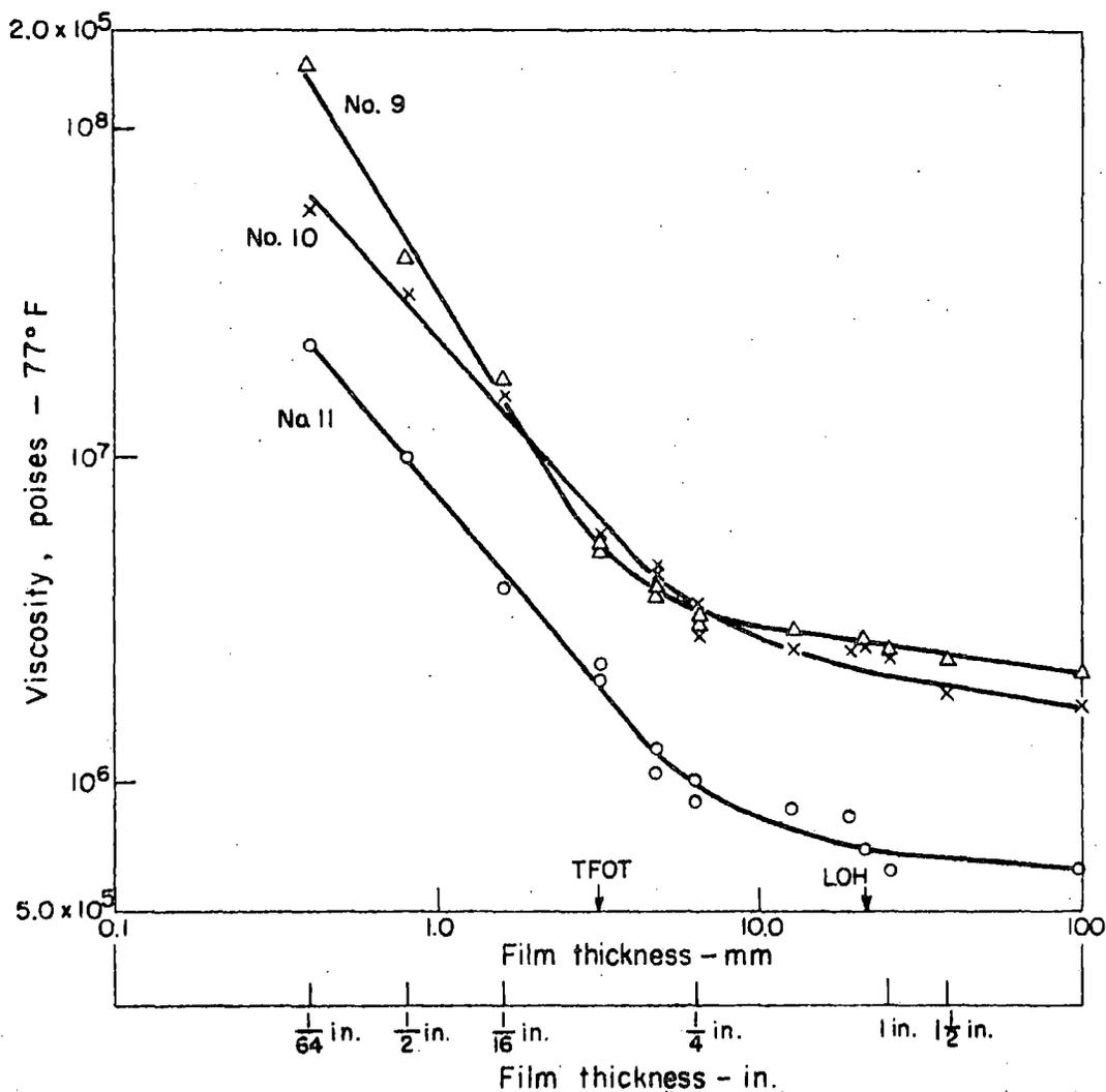
Fig. 9. Viscosity vs film thickness, TFOT.
