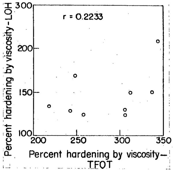
Fig. 23. Hardening LOH vs hardening TFOT, by viscosity.
