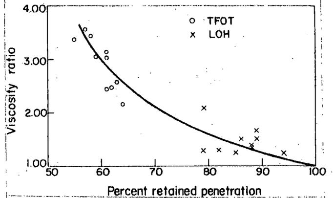
Fig. 24. Hardening by viscosity ratio vs hardening by retained penetration.
