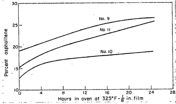
Fig. 17. Asphaltene content heating time.
