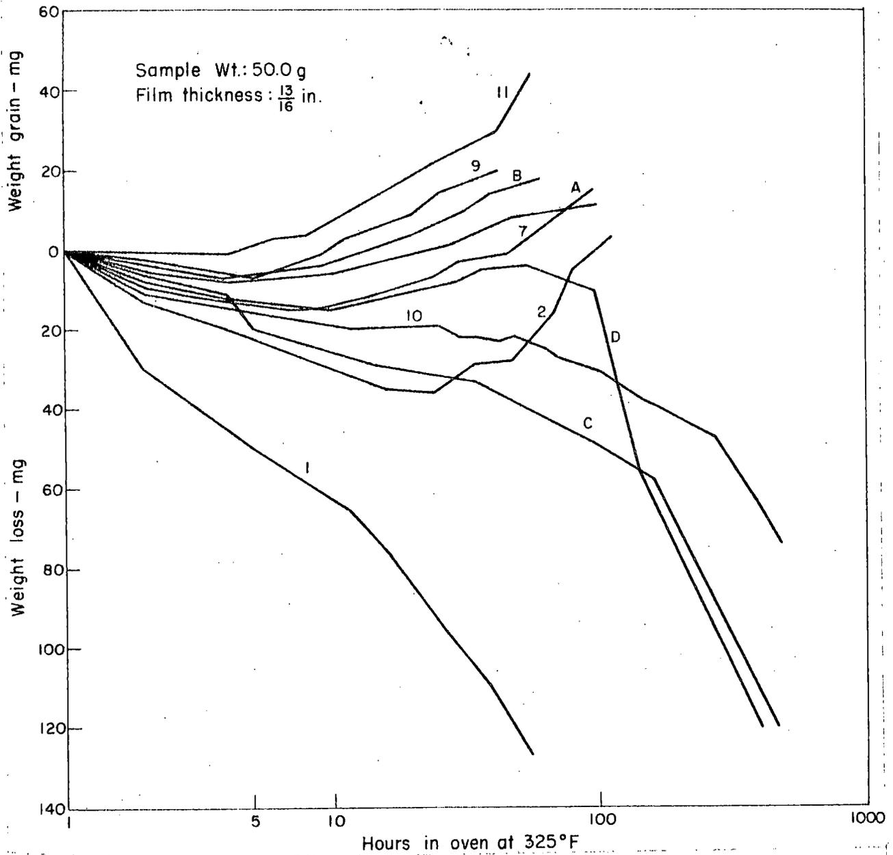
Fig. 20. Weight change during loss on heating tests (LOH).
