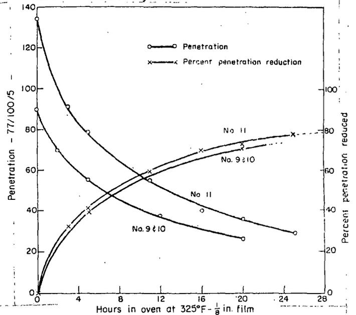
Fig. 13. Effect of heating vs time on penetration.
