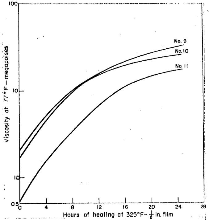
Fig. 15. Viscosity vs heating time.
