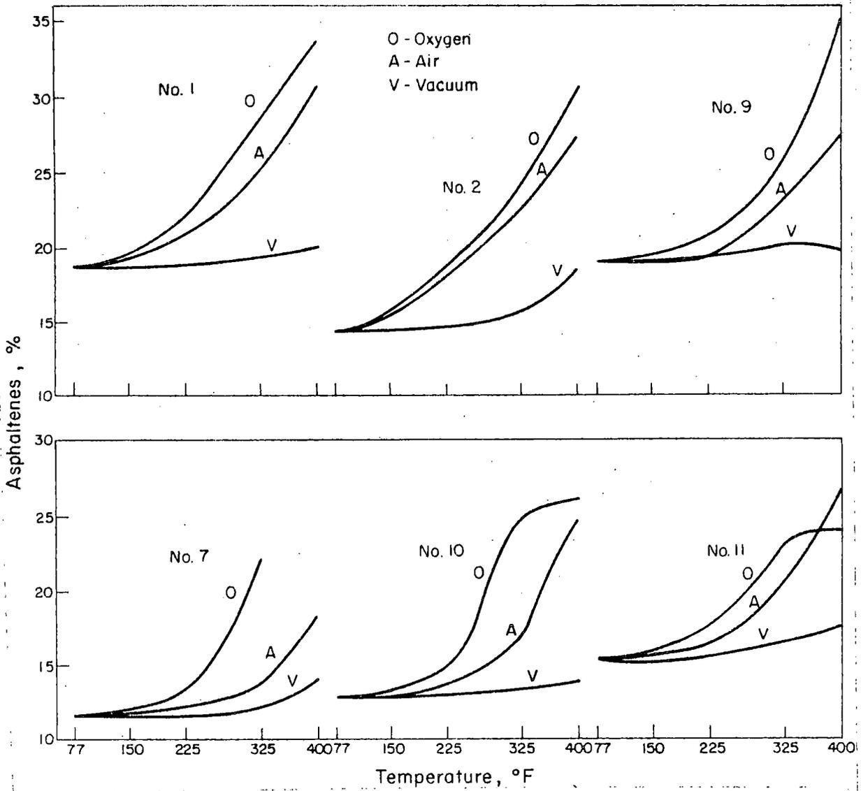
Fig. 7. Percent asphaltene vs temperature.
