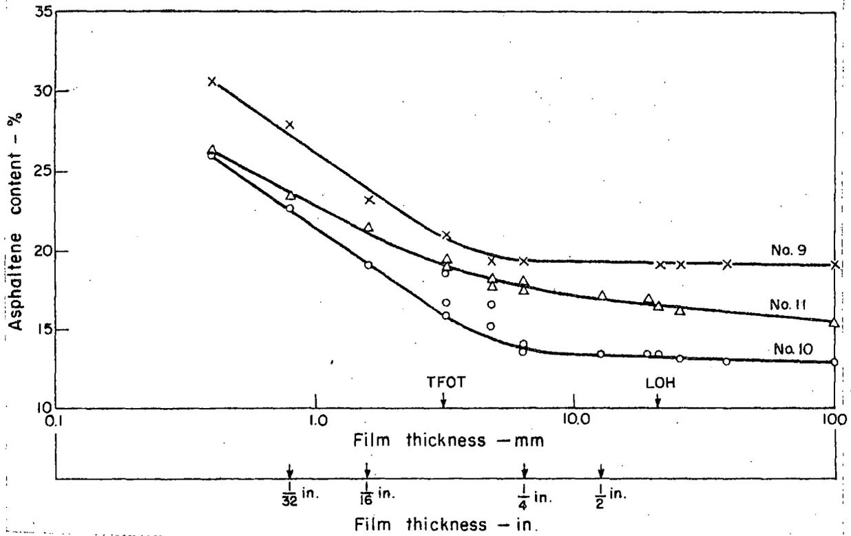
Fig. 11. Asphaltene content vs film thickness, TFOT.
