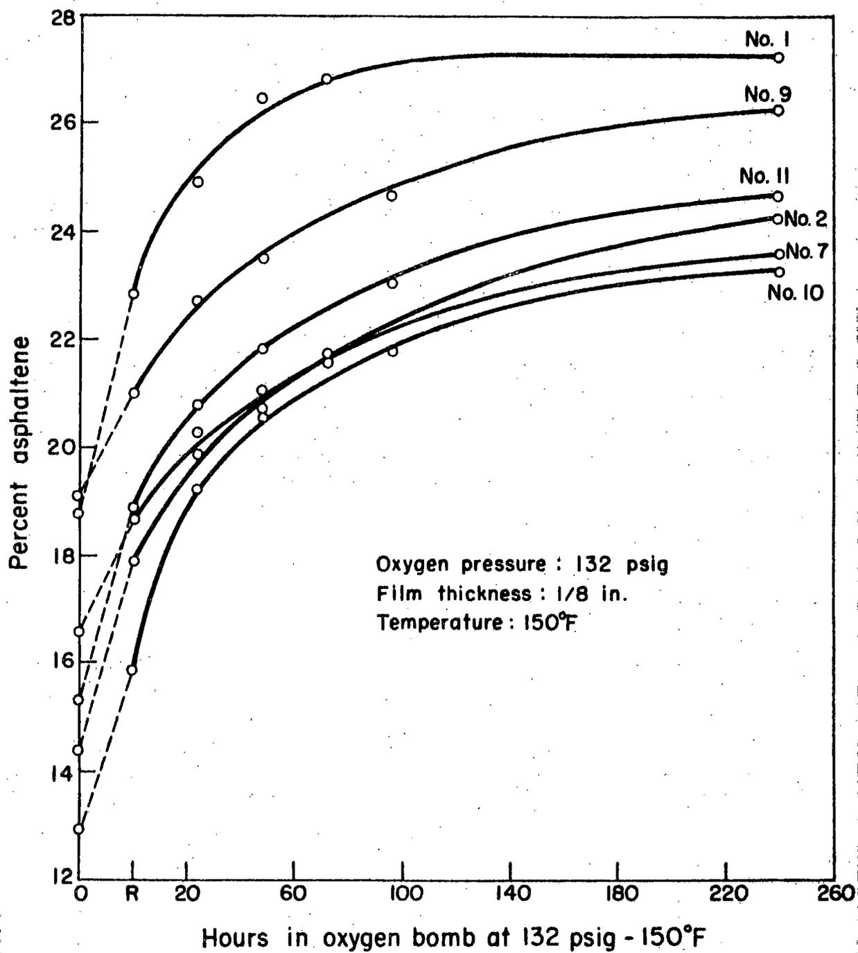
Fig. 7. Asphaltene content vs time of aging.
