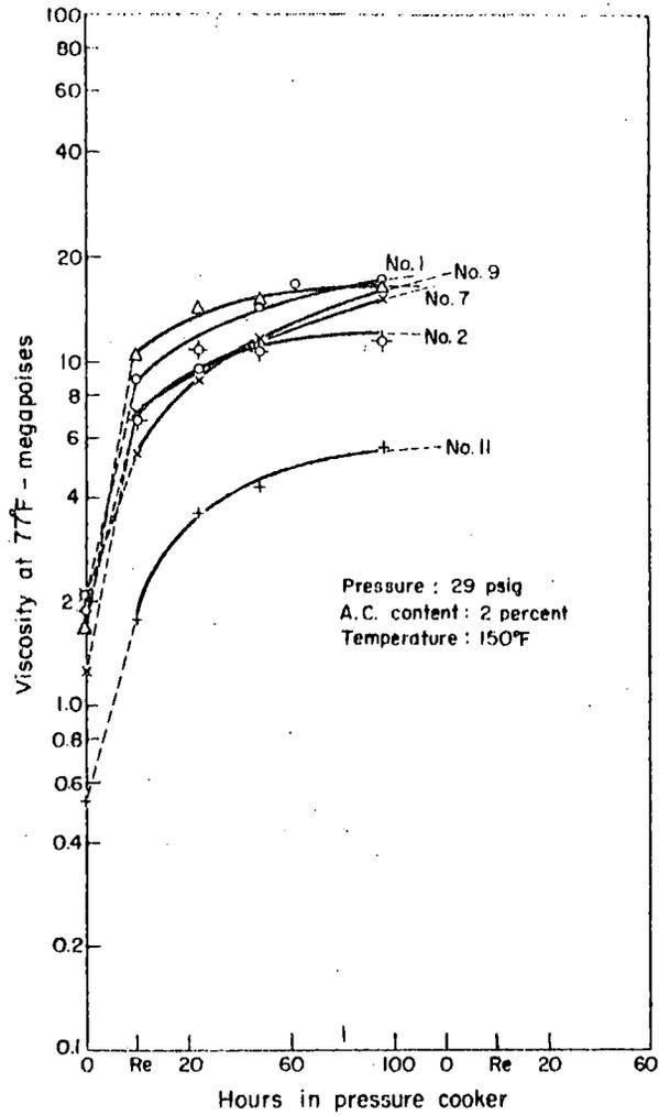
Fig. 10. Viscosity of recovered asphalt vs time of aging.
