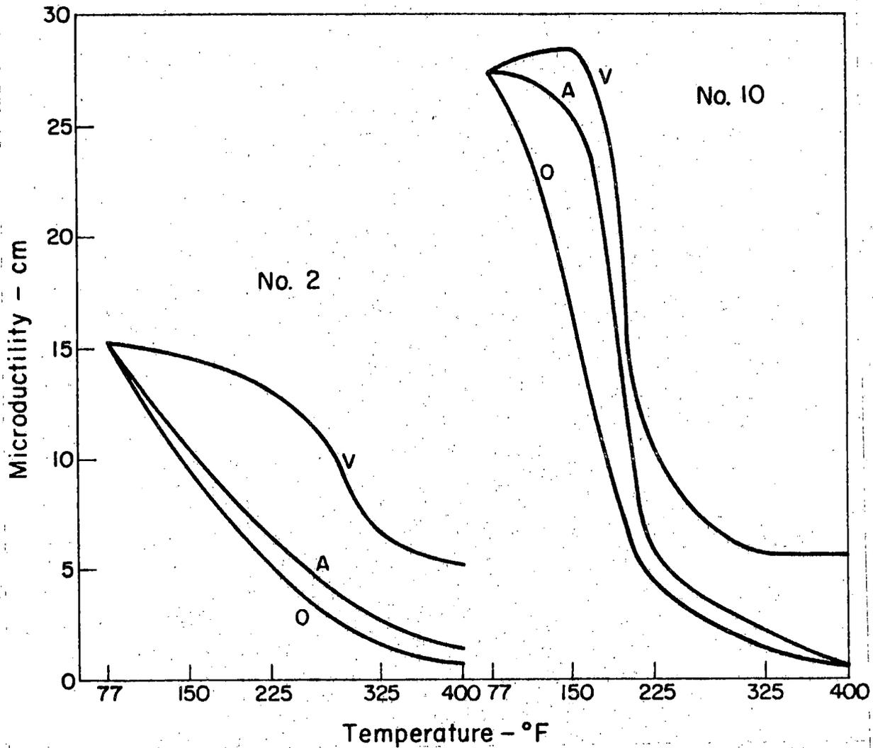
Fig. 26. Microductility at 60°F vs temperature and medium.
