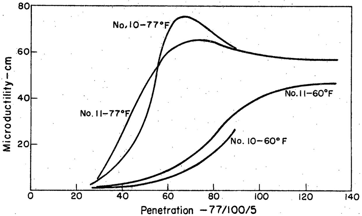
Fig. 28. Microductility vs penetration.
