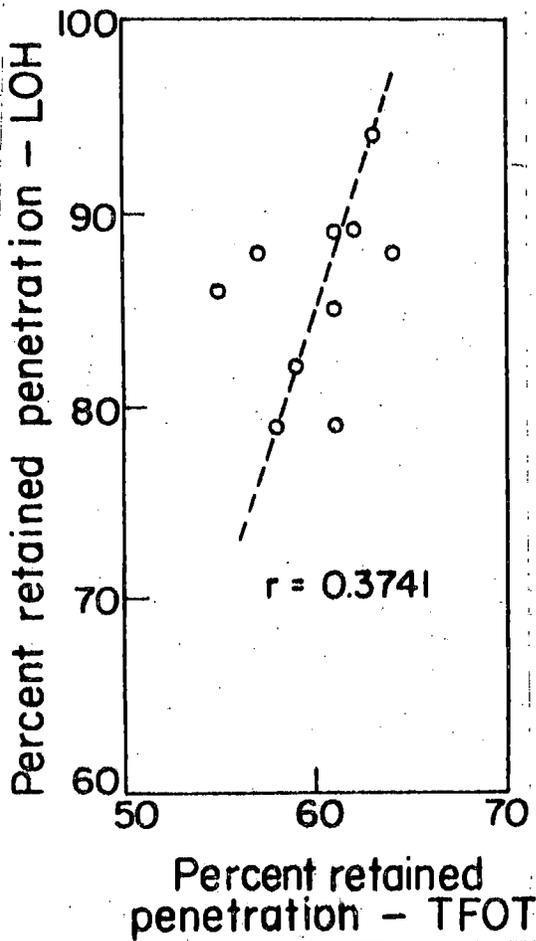
Fig. 22. Hardening LOH vs hardening TFOT, by retained penetration.
