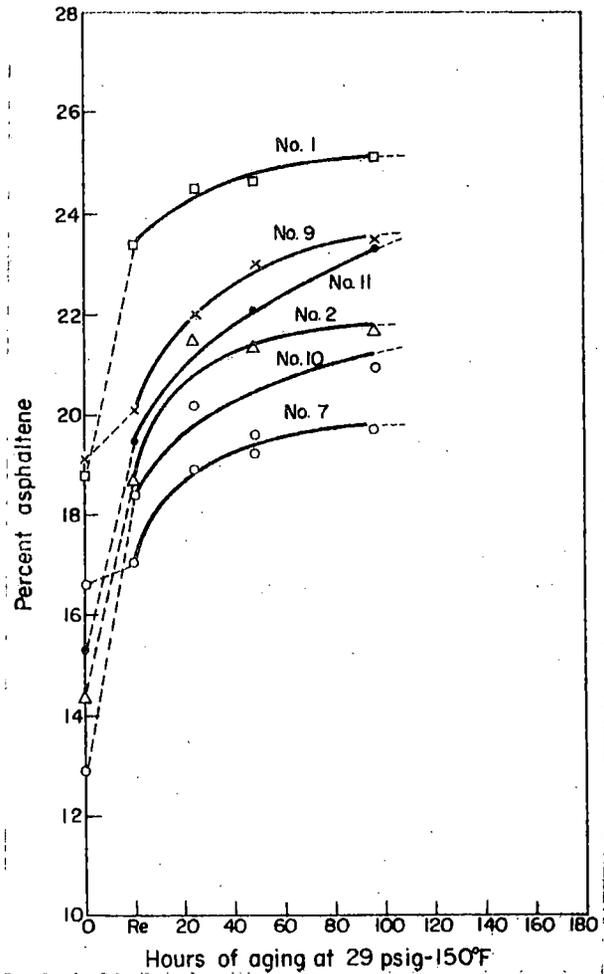
Fig. 11. Percent asphaltene of recovered asphalts vs time of aging.
