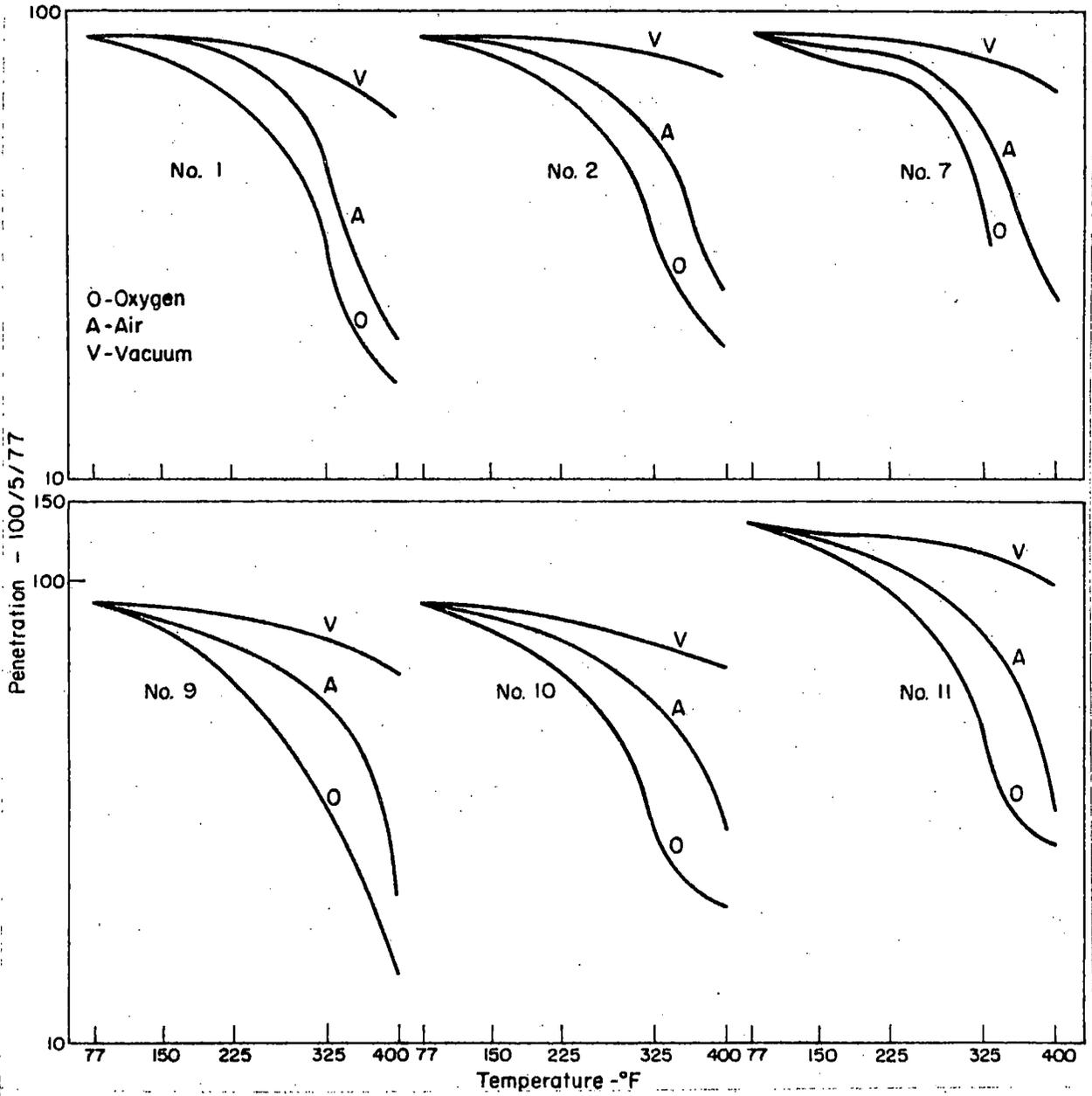
Fig. 2. Log penetration vs temperature.
