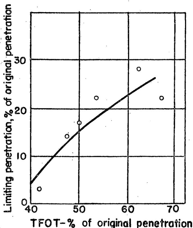
Fig. 29. Limiting penetration vs thin film oven test, after Way et al.
