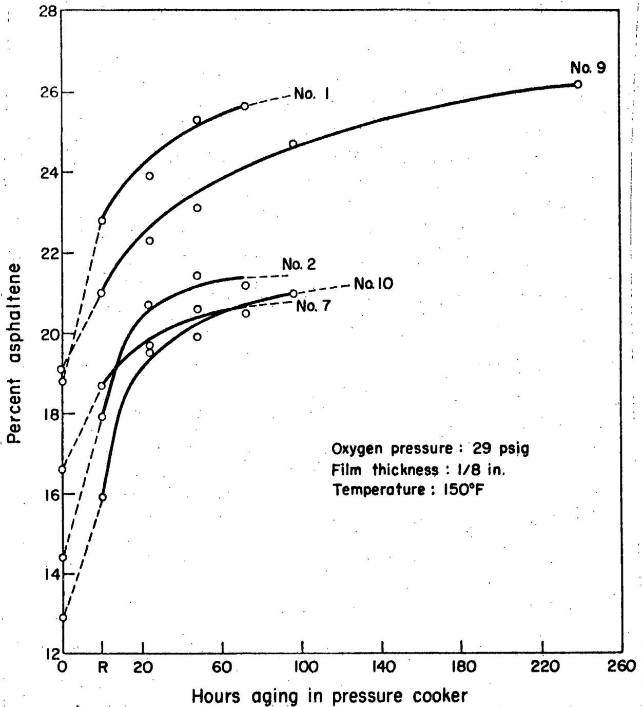
Fig. 6. Asphaltene vs time of aging.
