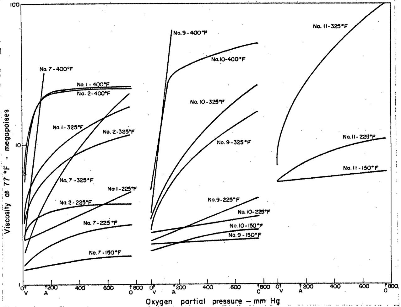
Fig. 5. Log viscosity vs oxygen partial pressure.
