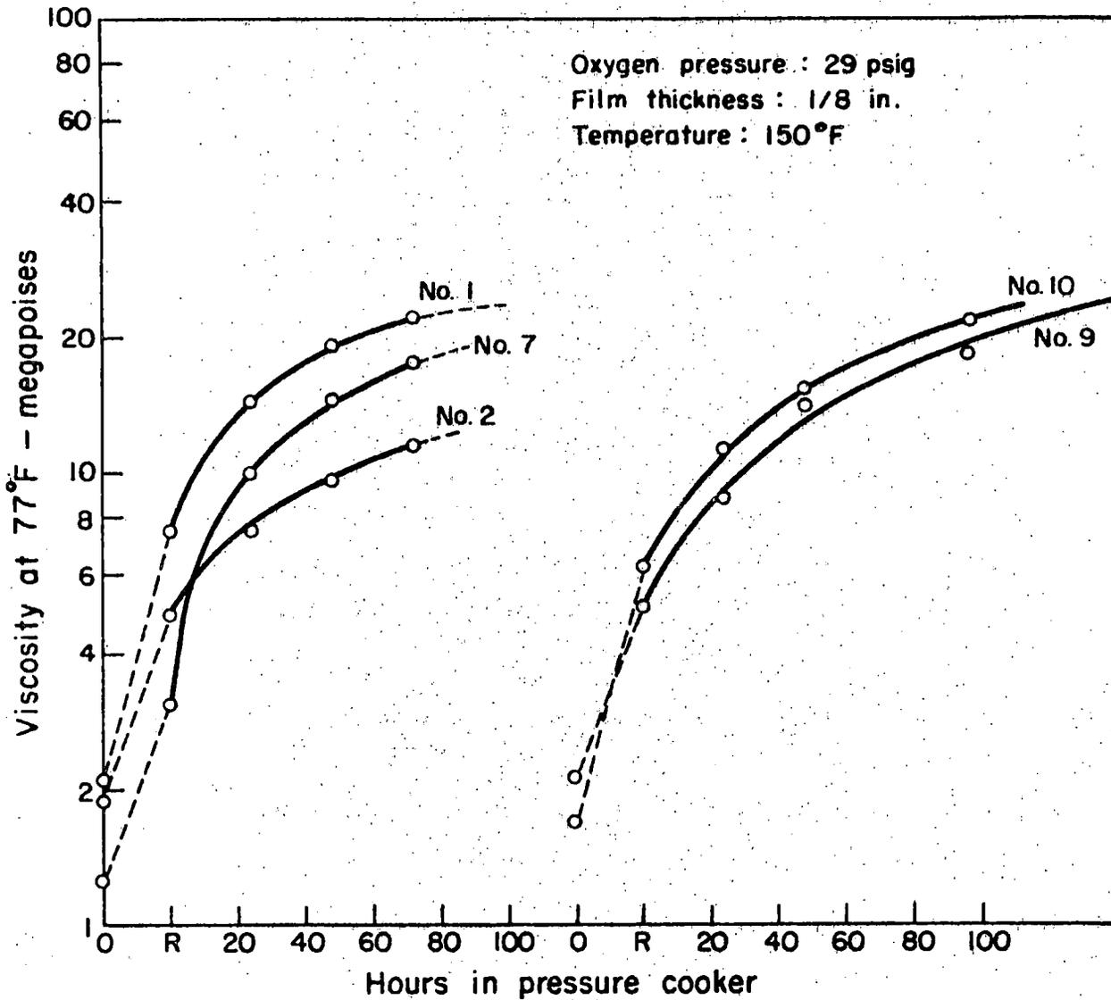
Fig. 1. Viscosity vs time of aging in pressure cooker.
