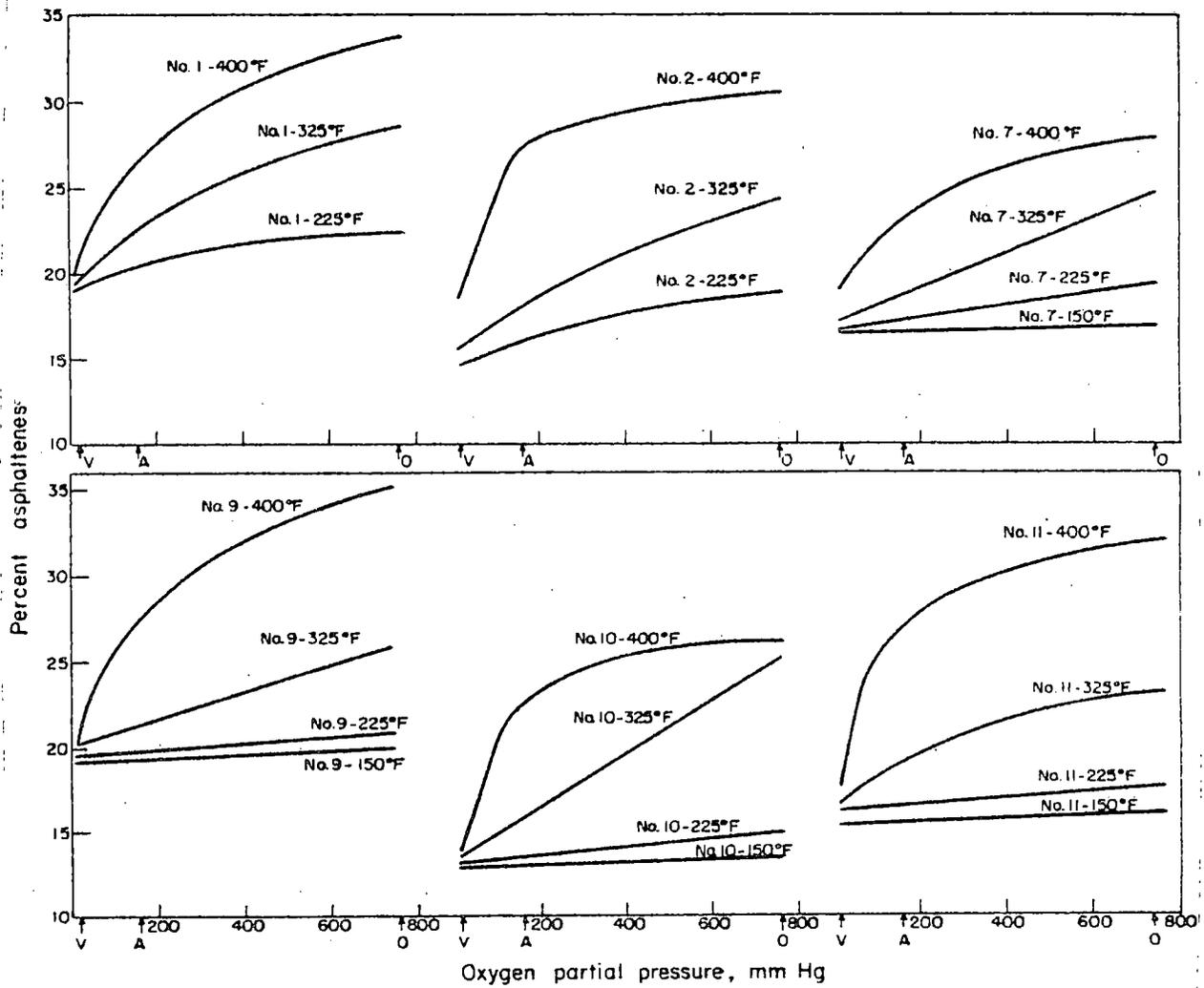
Fig. 6. Percent asphaltenes vs oxygen partial pressure.
