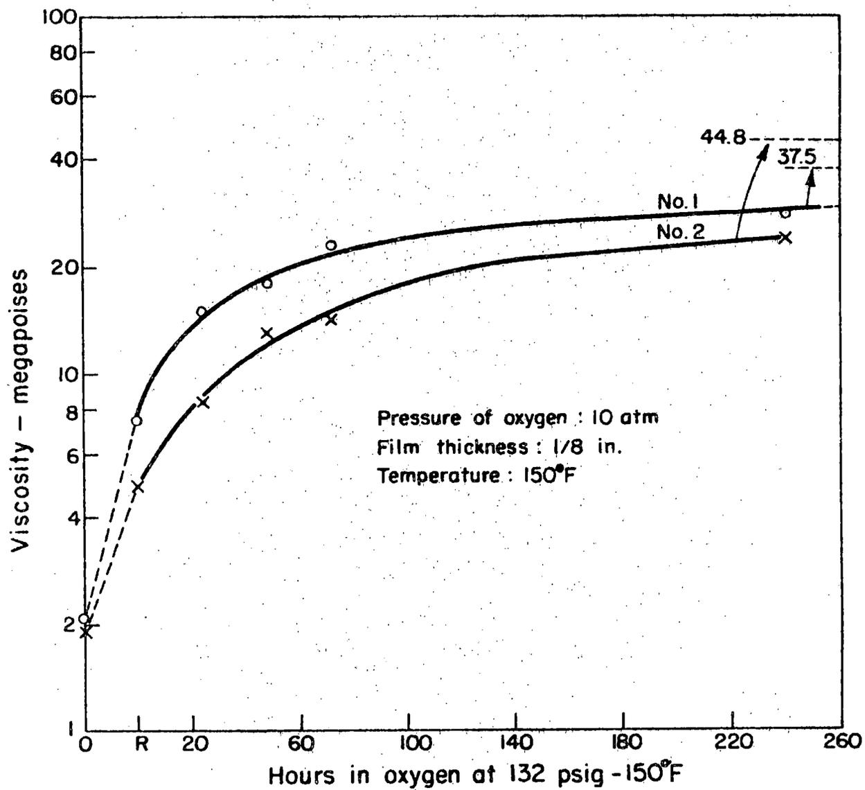
Fig. 2. Viscosity vs time of aging in pressure bomb.
