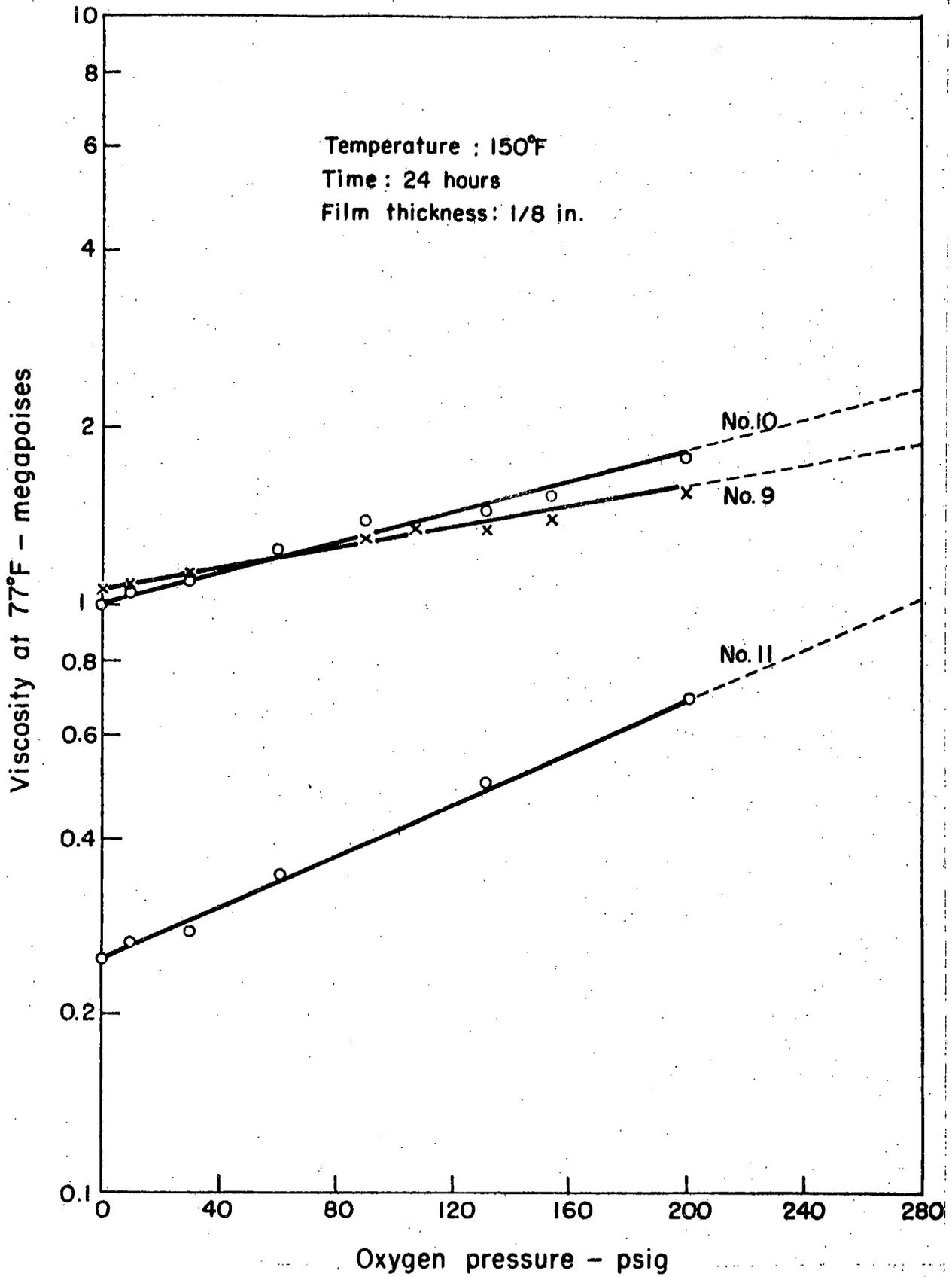
Fig. 8. Effect of oxygen pressure on viscosity.
