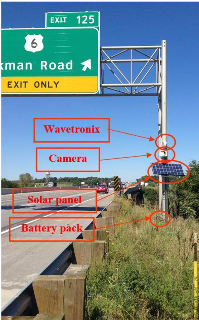
*Wavetronix SmartSensor HD detector and camera setup for measuring headway/time gap*
