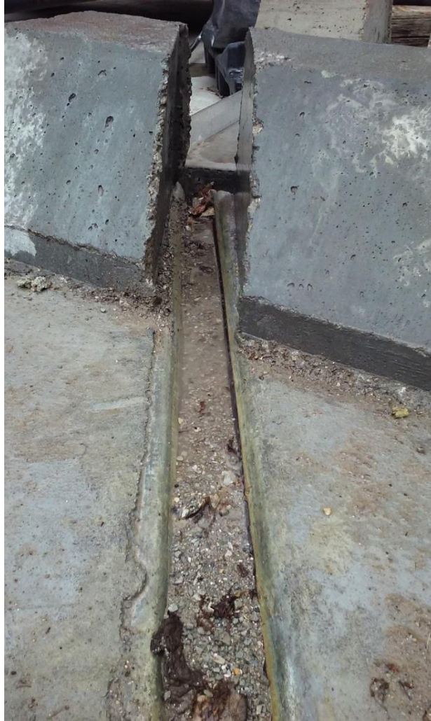
Figure 58. Mixture of debris on top of strip seal specimen after simulating water flowing heavily off the bridge
