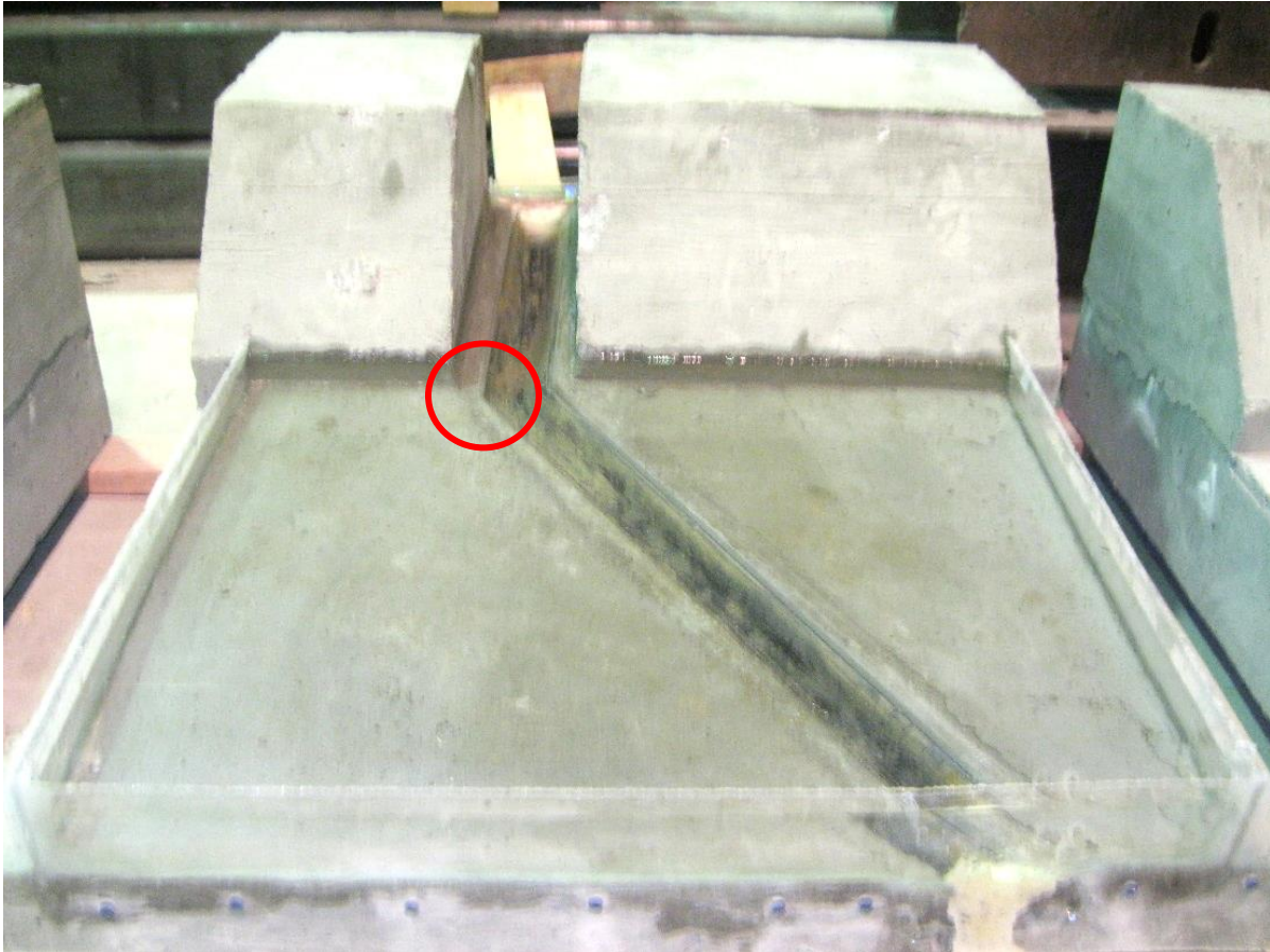
Figure 54. Watson Bowman Acme dogleg specimen with leaking gland
