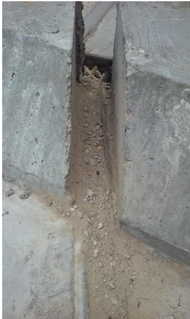
Figure 57. Mixture of dry debris placed on top of strip seal specimen
