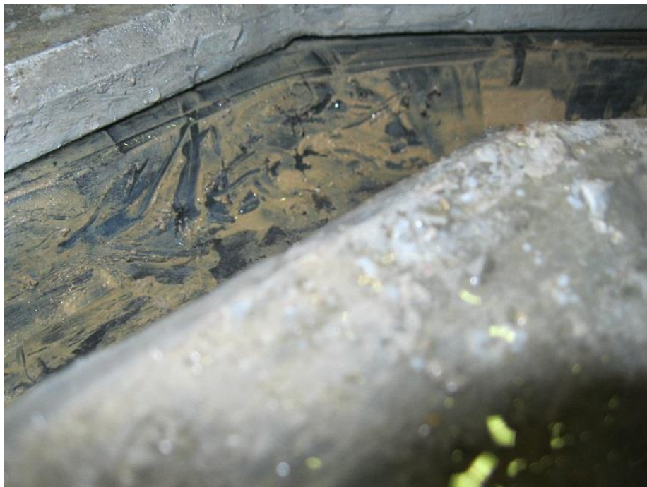
Figure 56. Second attempt to properly install gland in Watson Bowman Acme dogleg specimen
