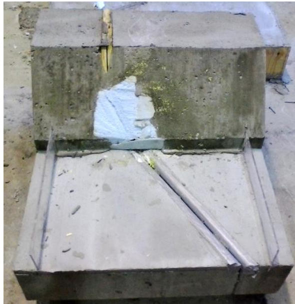
Figure 32. Completed blackout area using insulation board
