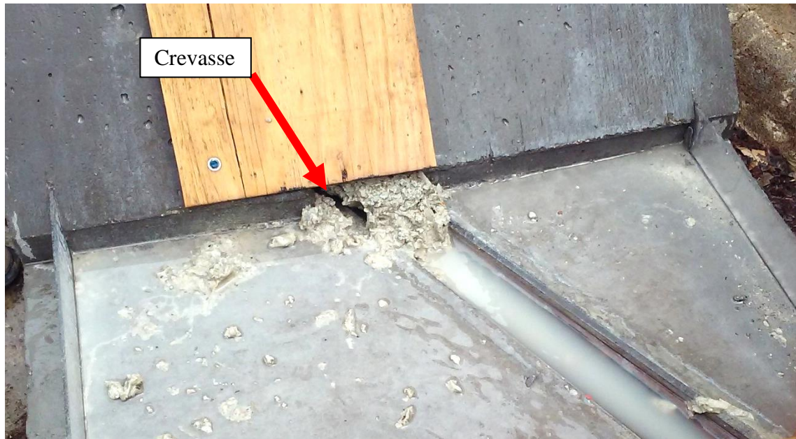
Figure 62. Crevasse that had formed in saturated bentonite causing ponding test failure
