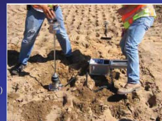
Light Weight Deflectometer (Model: Zorn ZFG2000)
