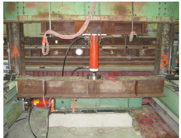
*Coefficient of friction test setup, showing stainless steel sole plate and PTFE-topped neoprene bearing pads*
