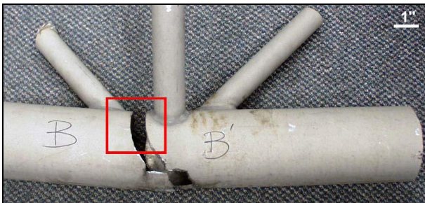
Picture showing a crack developing at the welding heat zone
