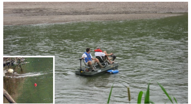
Figure 4. Detection of the particles in the Raccoon River via an antenna towed by a boat. On the left corner, a scour ball found floating in the river.
