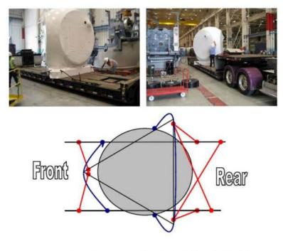
This is a top view of the Hub on a trailer. The red colored line refers to chains coming off the attachment points. The blue lines refer to chains wrapping in front or behind the shipping frame to prevent forward or backward movement.
