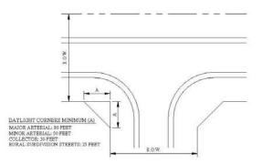
Figure 1: Minimum Daylight Corners
