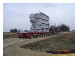
Figure 3.12. Electrical transformer en route to power station (photo courtesy of Mitchell County)
