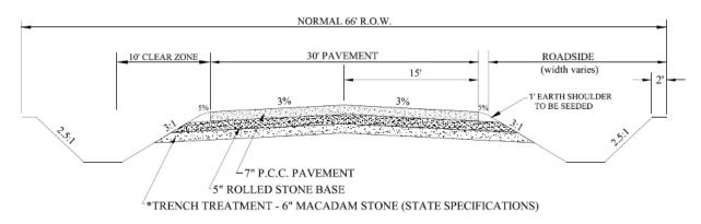
Figure 5.10. Typical minimum PCC pavement—open ditch section
