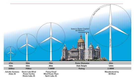
Figure 2.19. Wind turbine heights in Iowa (Iowa Energy Center)
