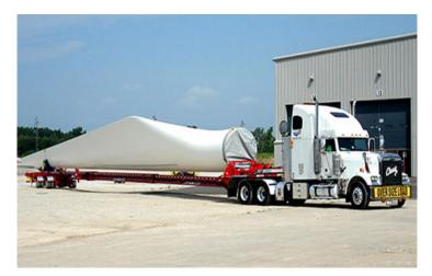
Figure 2.20. Transporting large wind turbines (Treehugger 2008)
