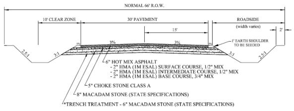
Figure 5.11. Typical minimum HMA pavement, macadam stone base—open ditch section
