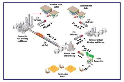
Figure 4.2. Typical transport system for biofuels production (National Bioenergy Center, National Renewable Energy Laboratory)
