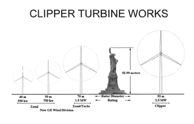
**Figure 6.1. Clipper turbine evolution**
