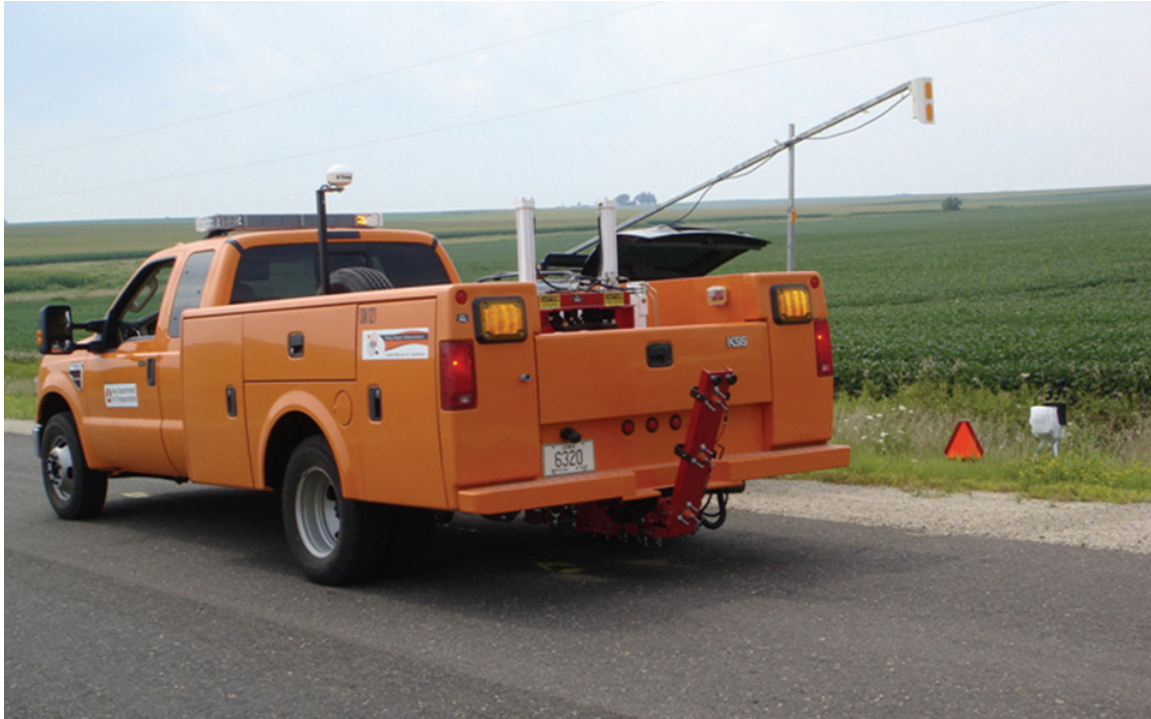
Figure 7-18. Measuring modulus of the CIR-foam layer using FWD
