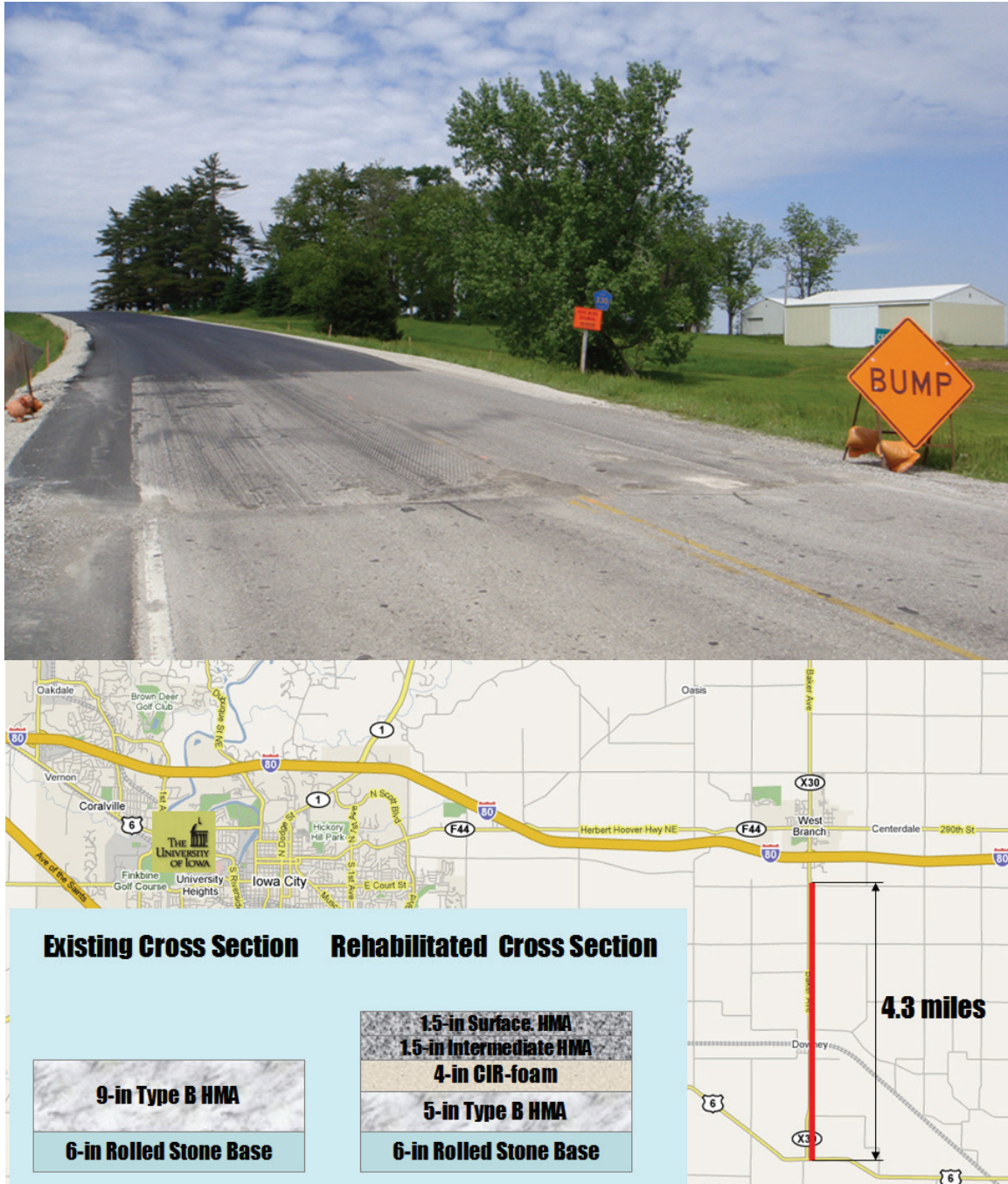
Figure 5-3. Comparison of pavement cross section of CIR-foam project site in Cedar County
