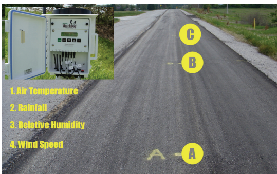
Figure 6-7. Pictures of installation process for embedded moisture and temperature sensors at the bottom of the CIR-CSS-1-emulsion layer
