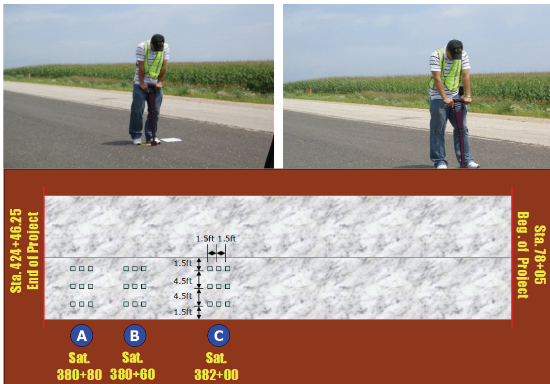
Figure 7-13. Nine moisture measurements for each location using a portable TDR
