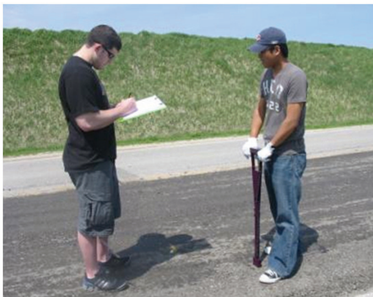
Figure 5-9. Nine moisture measurements for each location using a portable TDR
