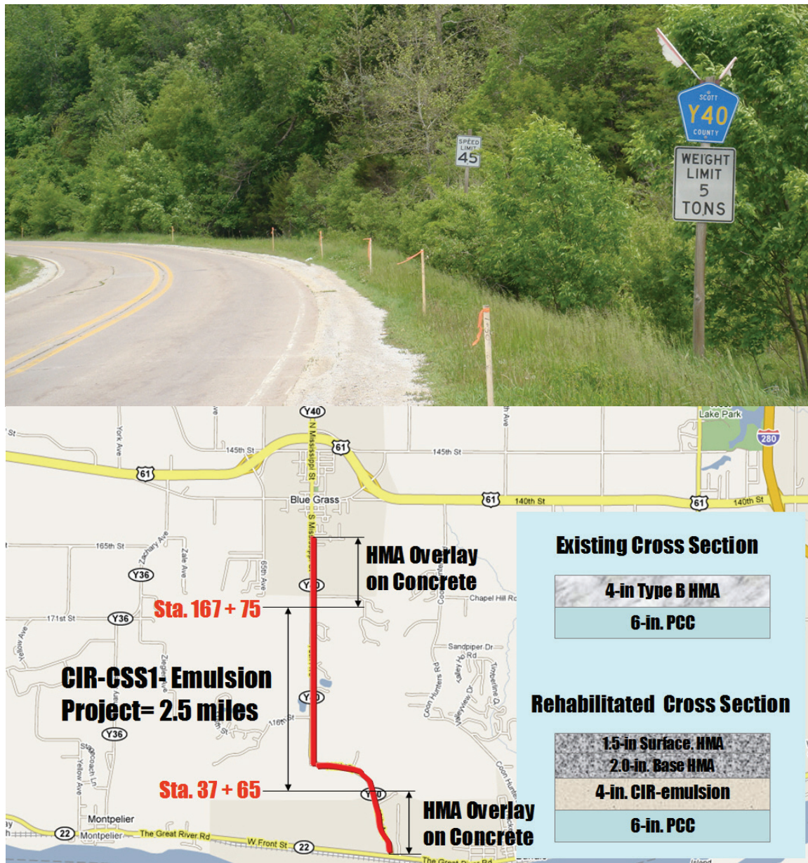
Figure 6-2. Comparison of pavement cross section of CIR-CSS-1-emulsion project site in Scott County
