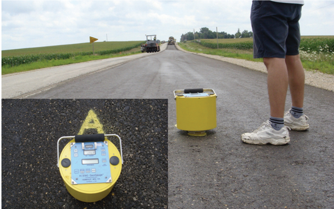
Figure 7-20. Measuring stiffness of the CIR-foam layer using geo-gauge
