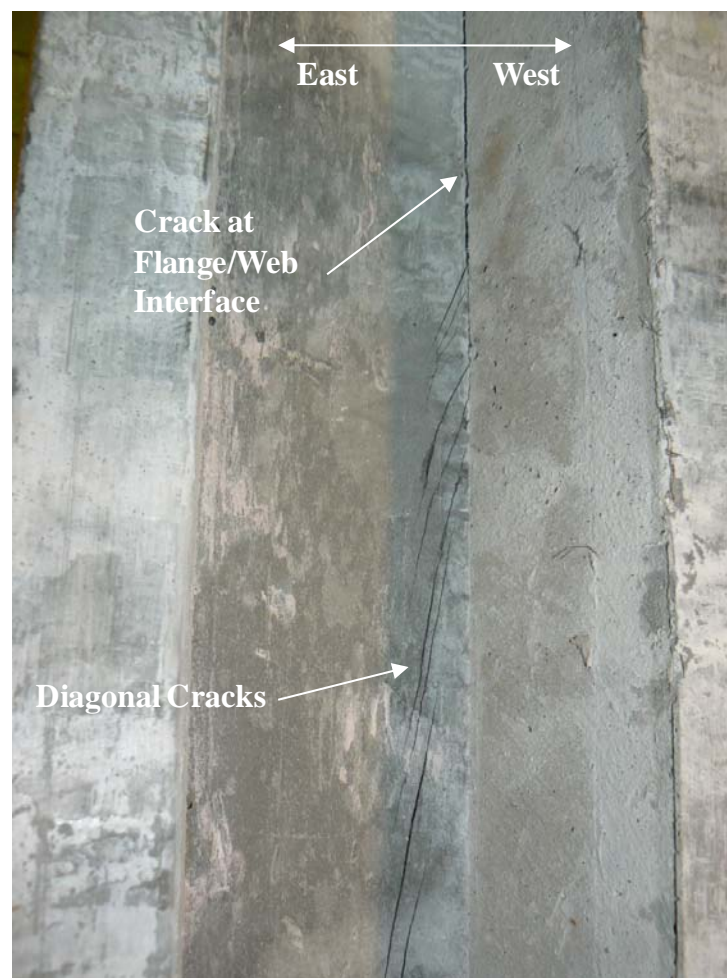
Figure 4.32. Diagonal cracking in test unit L2 at a lateral load of 5.2 kips (23 kN) (pull)
