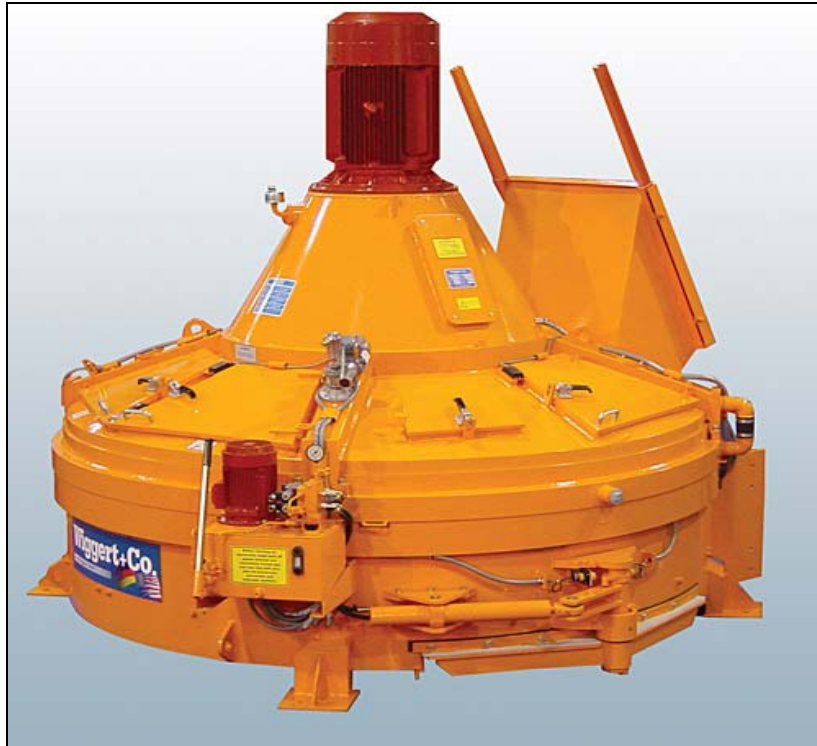
Figure 37. Countercurrent concrete mixer (Advanced Concrete Technologies 2007)
