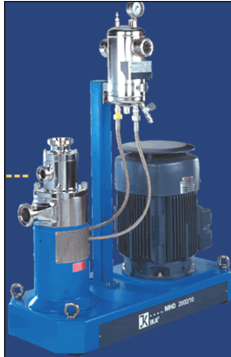
Figure 40. Powder-liquid high shear mixer (IKA 2007)
