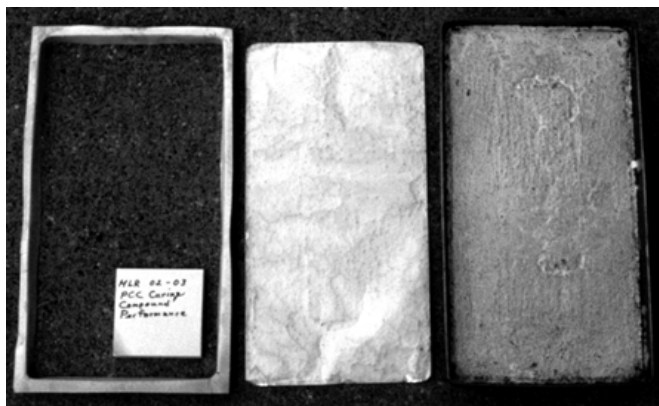
Figure 2 Rim, Foil, and Concrete in Mold
