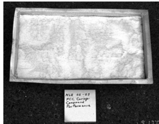
Figure 3 Rim, Foil, and Concrete in Mold Assembled for Testing
