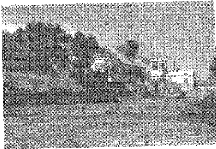
Figure 3 The Benton County End Loader Dumping Bituminous Shingles into the Maxigrind
