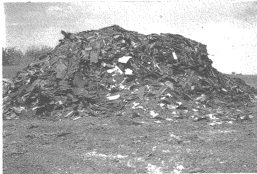
Figure 2 A Pile of Benton County "Torn Off" Bituminous Shingles
