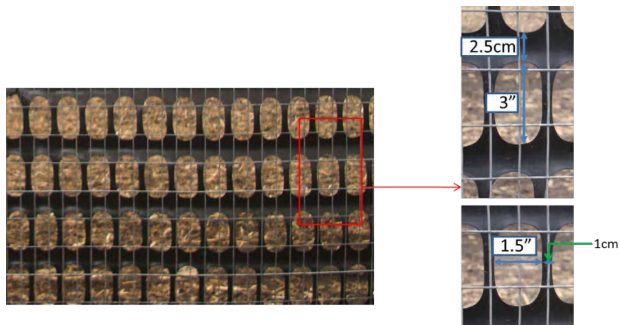
Figure 14. Detail view showing layout of plastic fence.
