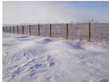
Figure 37. Snow deposition profiles (A1 fence, January 20, 2011).
