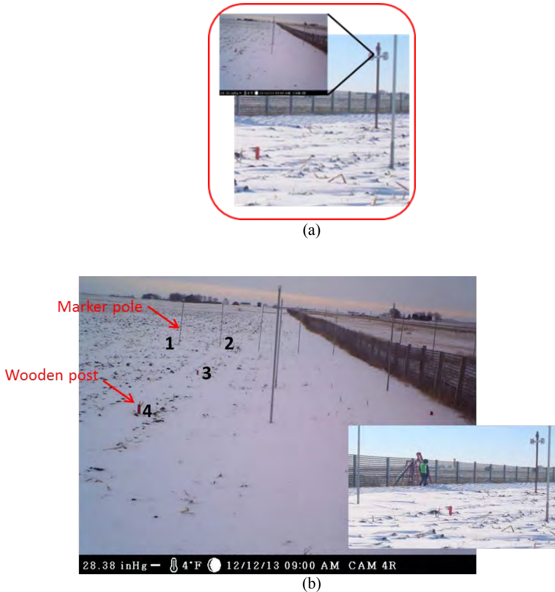
Figure 114. Protocol 2 for snow depth estimation: a) images acquired for processing: b) view of the experimental site on December 12, 2013 (relocation coefficient = 0.71).
