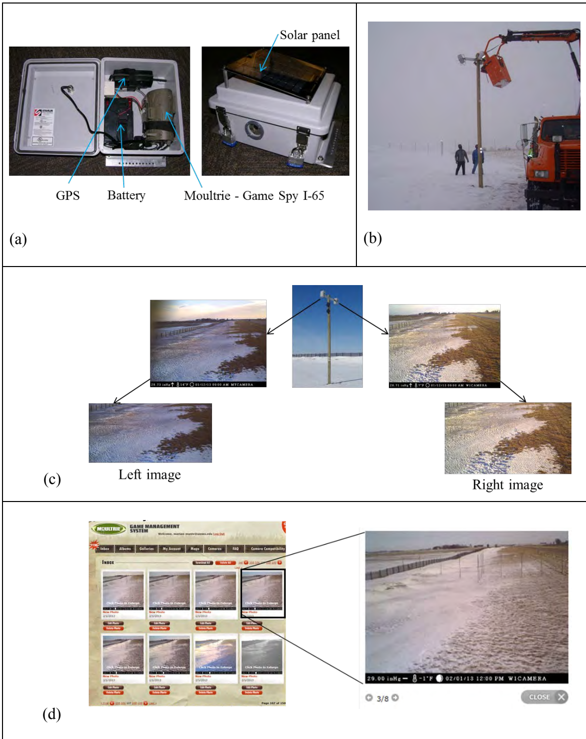
Figure 46. The image-based system used for site monitoring: a) the camera assembly; b) camera installation in the pole; c) raw images acquired for CRP processing; d) the real-time, web-based image-management platform.
