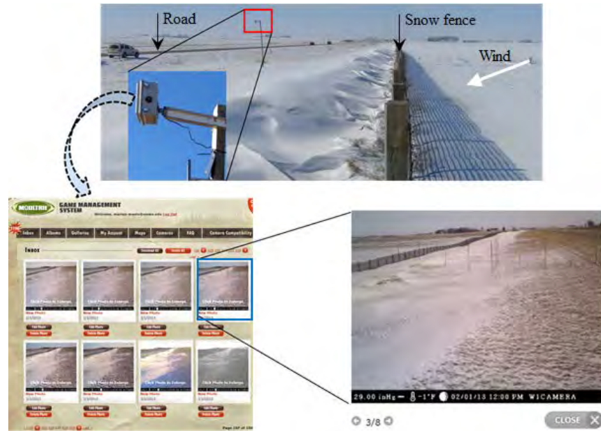
Figure 27. Field set-up and information provided by the real-time monitoring system.
