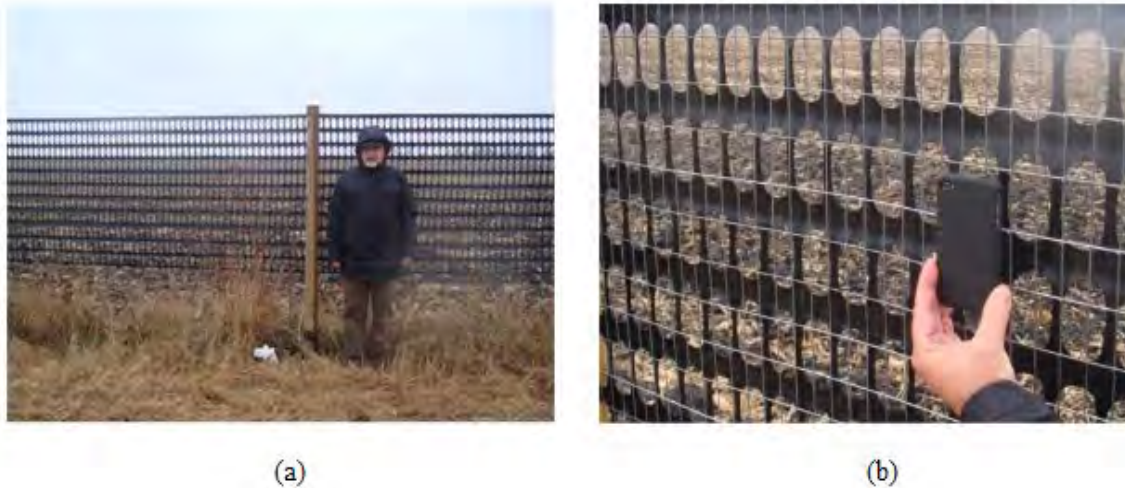
Figure 12. (a) View of one of the lightweight plastic snow fences tested at the field site (A1 fence: P=50\% , G/H=0.34 , H \cong 1.9 ); (b) Close view showing the 2 mm diameter welded wire frame used to support the plastic fence.
