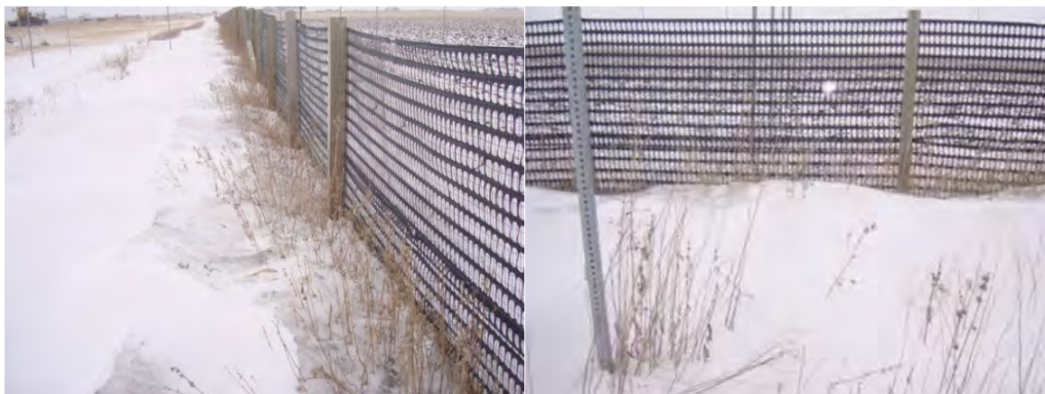
Figure 93. Views showing snow deposition close to the fence on January 22, 2014 immediately after the end of one of the significant snow events occurring during the third winter season: a) B1 fence ( P=30\% , G/H=0.25 ; b) B2 fence ( P=30\% , G/H=0.2 ); and c) A3 fence ( P=50\% and G/H=0.08 ). The blue lines indicate bottom of the fence.
