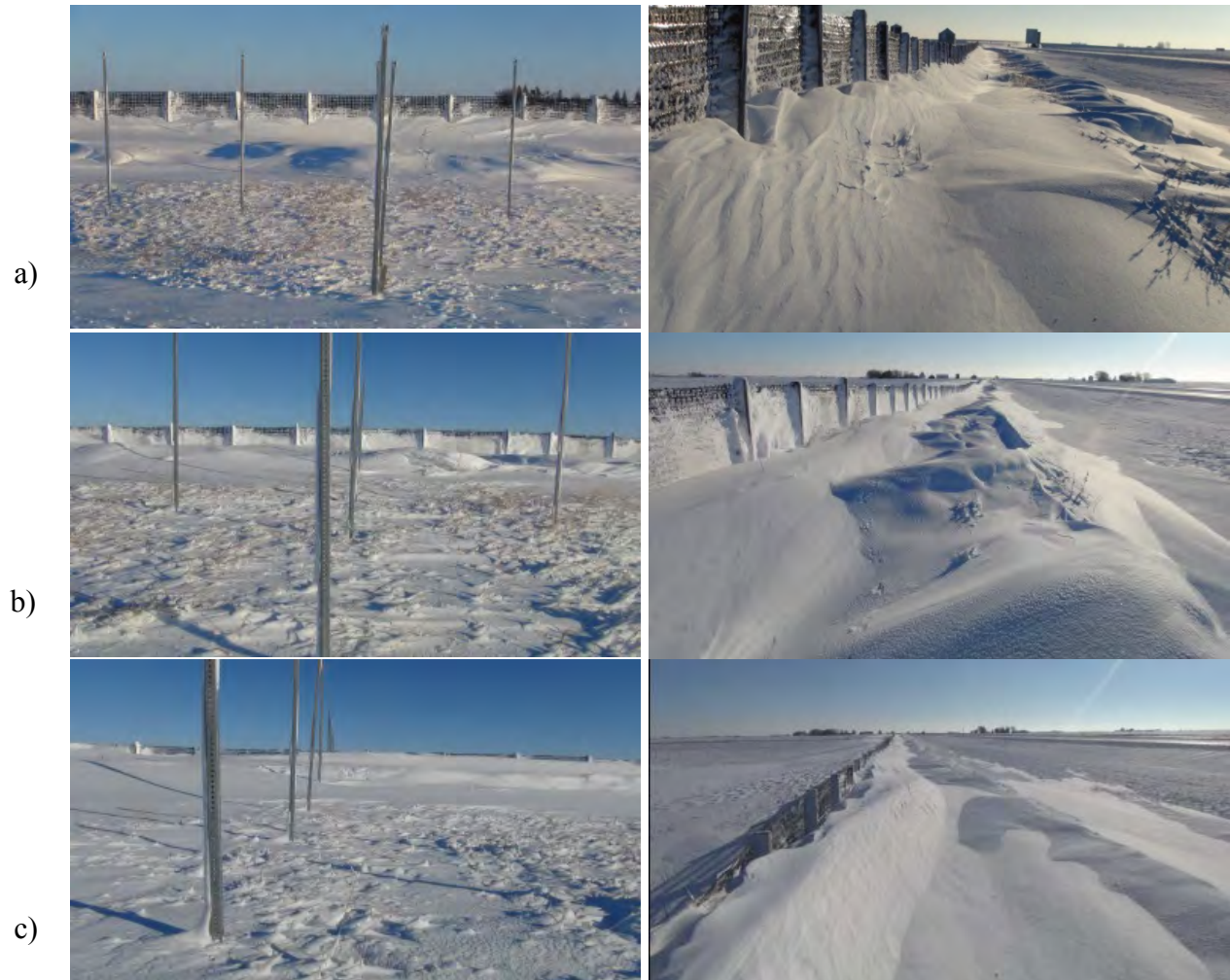
Figure 95. Views showing snow deposition close to the fence immediately after the end of the largest snow event during the third winter season: a) B1 fence ( P=30\% , G/H=0.25 ; b) B2 fence ( P=30\% , G/H=0.2 ); and c) A3 fence ( P=50\% and G/H=0.08 ).
