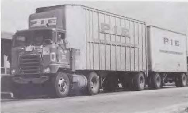
65-Foot Twin-Trailer (Double Bottom) Truck
