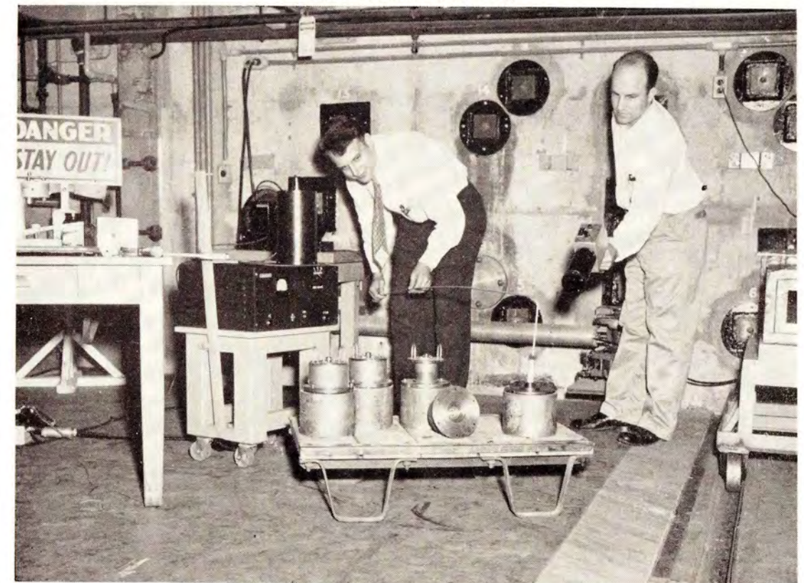
ABOVE: Removing isotopes from the atomic pile BELOW: Putting radioisotopes in a lead shipping container (Courtesy United States Army)
