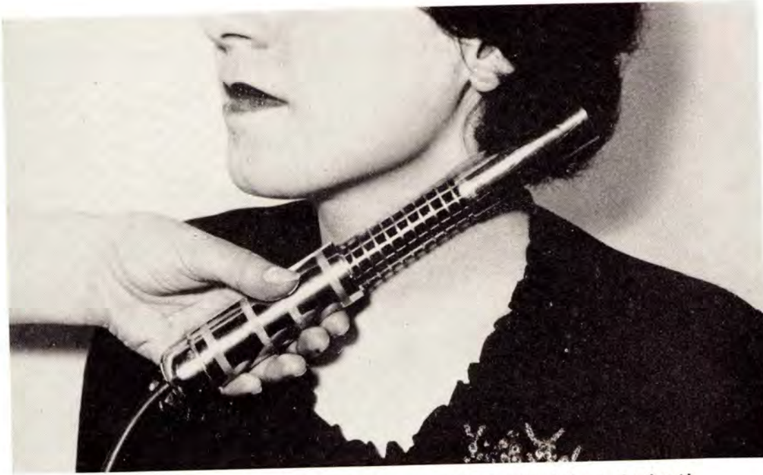
ABOVE: A Geiger counter is used to detect the presence of radioactive iodine in the thyroid
