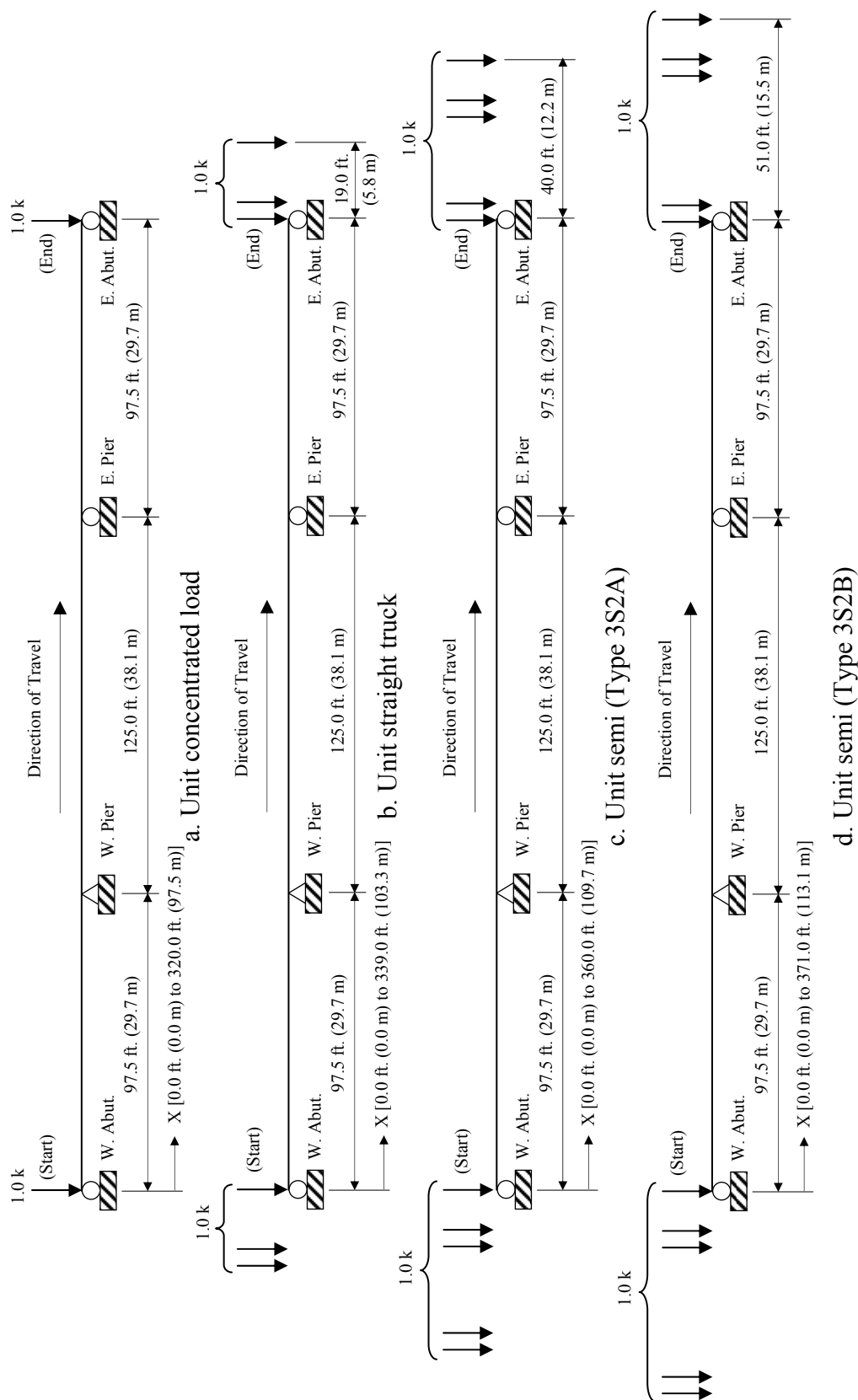
Figure 5.6. Positioning and length of travel for the unit concentrated load and unit trucks in the south girder static analyses
