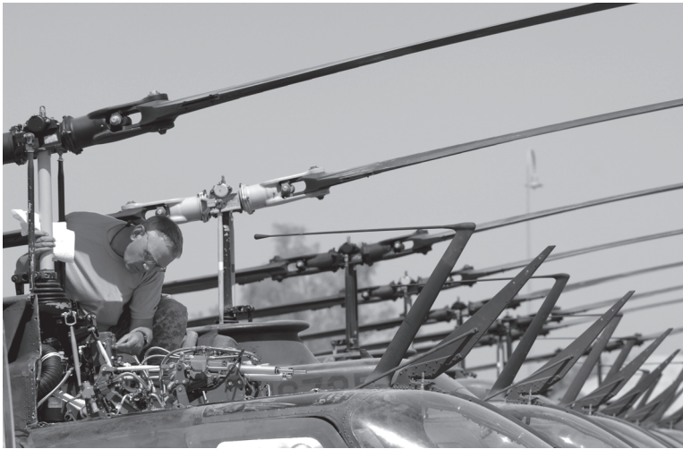
Staff Sgt. Marshall Lantz, Det. 1, 1 134th Security and Support Battalion crew chief, performs a receiving inspection on an OH-58 Kiowa. The helicopters were shipped to Iraq and then flown to Camp Taji to be used for Iraqi Air Force pilot training. (Photos by Sr. Airman Julianne Showalter, 332nd Air Expeditionary Wing)
