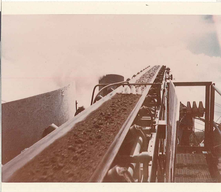
Addition of 3% moisture on cold feed by means of Spray Bar.
