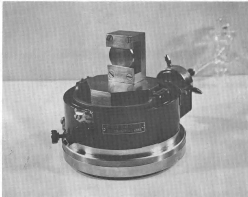
(b) Base of the X-ray adsorption apparatus showing the sample holder.
