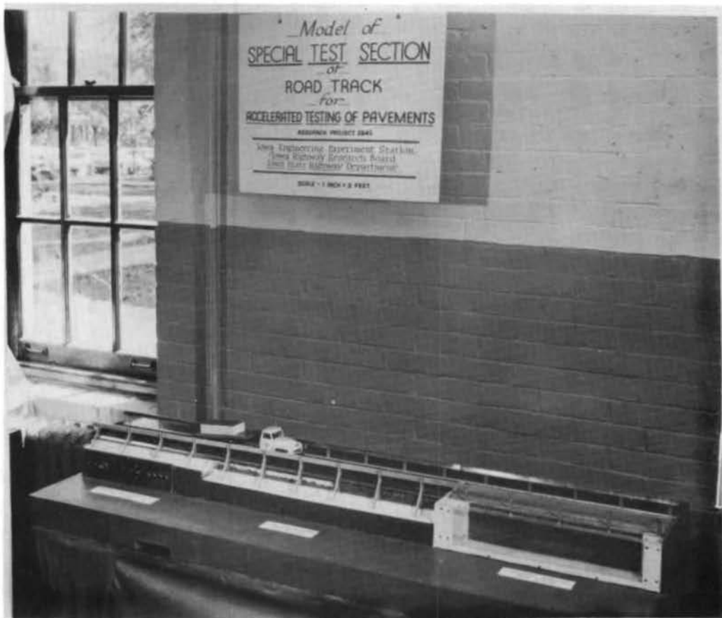
Plate IV. Model of Special Test Section
