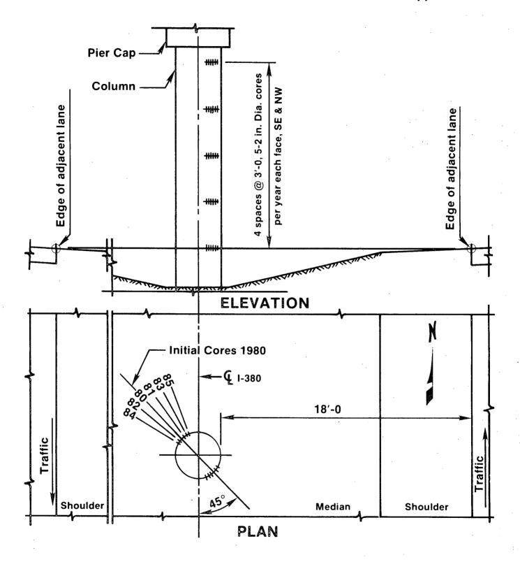
FIGURE 3 - I-380 CORE SAMPLING PLAN
