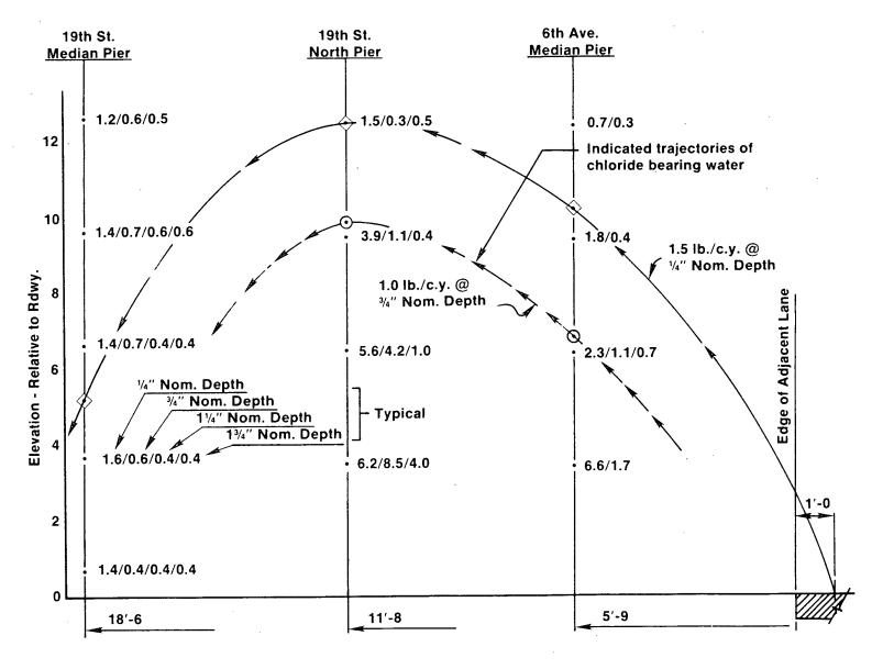
FIGURE 1 - CHLORIDE CONTENTS I-235 PIER COLUMNS
