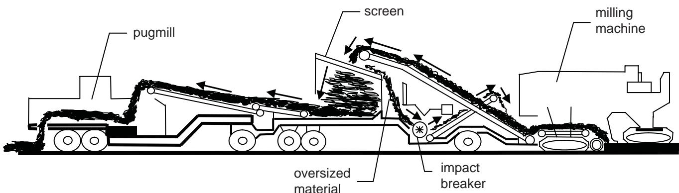
*Diagram of a typical CIR milling, screening, crushing and pugmill unit, traveling left to right, paving and compaction units not shown (based on Jahren et al., 1998, Review of Cold In-Place Recycled Asphalt Concrete Projects, IHRB Project HR-392)*
