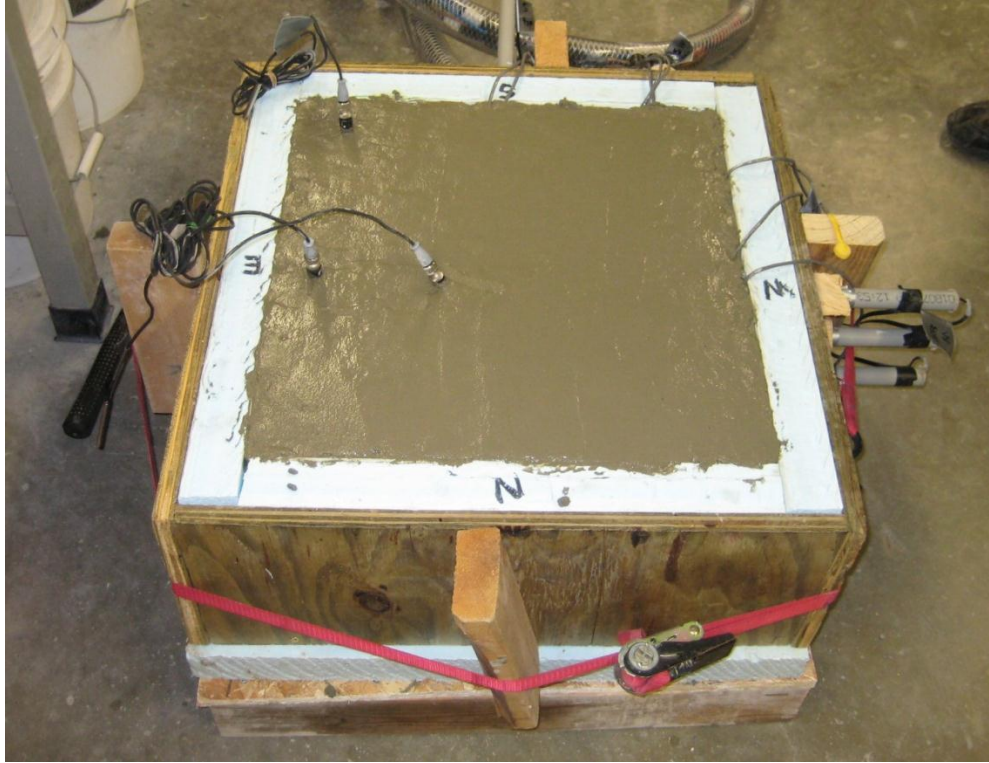
Figure 31. Freshly placed concrete in the instrumented form
