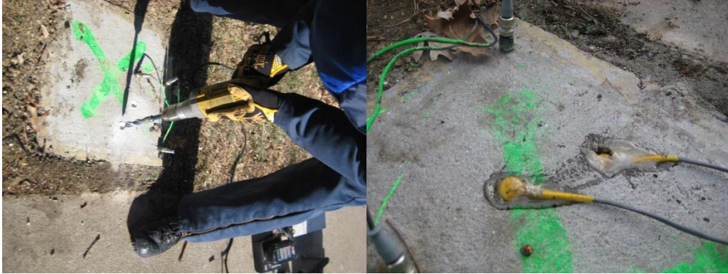
Figure 47. Installation of iButton sensors at the surface of the instrumented slab during test phase 4
