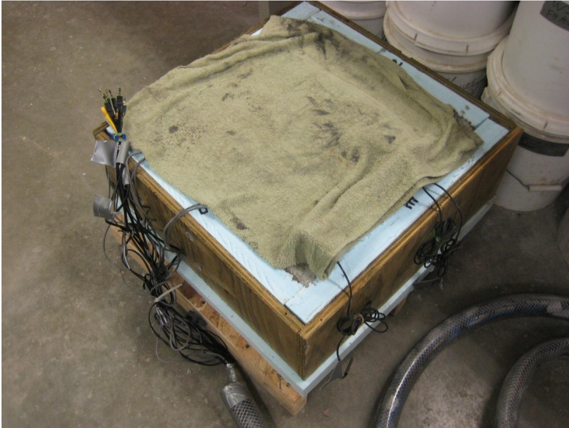
Figure 34. Instrumented slab in ISU PCC laboratory during test phase 1
