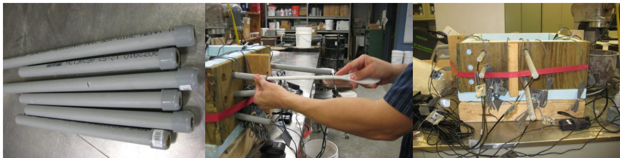
Figure 26. MEMS sensor installation in concrete slab form
