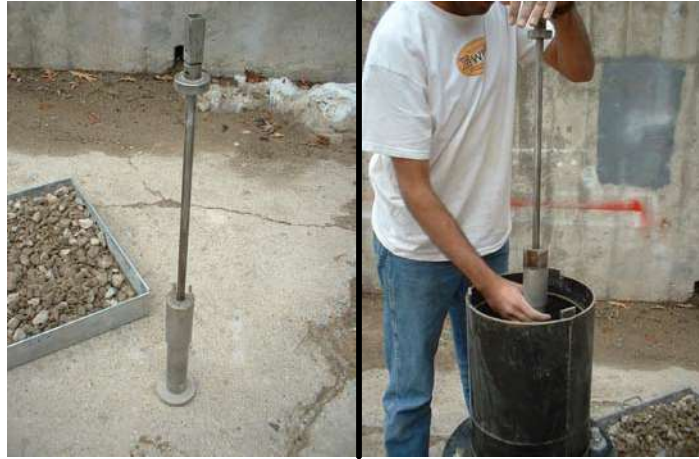
Figure B4. Marshall impact hammer (left) and compaction procedure (right)
