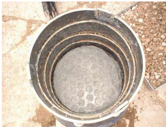
Figure B3. Aggregate compaction mold with screens placed over the base mold
