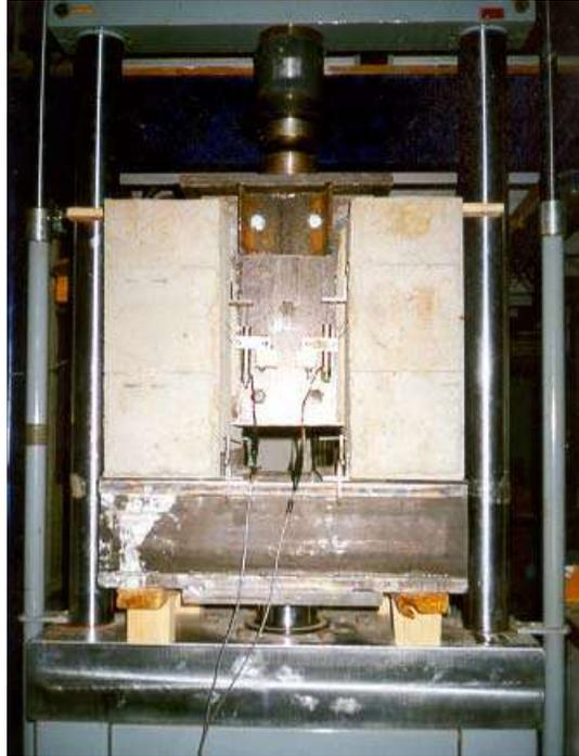
Figure 4.12. Photograph of push-out test set-up.
