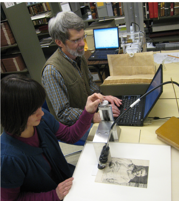
Barrett's research assistant Jessica White (MFA Printmaking, UICB Certificate 2009) tests a 15th century book with a non-destructive XRF (x-ray fluorescence) spectrometer. The instrument provides data on calcium, iron, and other elemental content in the paper.
