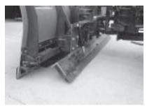
S lush blades made of one-andone-half-inch rubber will be added behind the normal carbide snow plow blade and tested for its ability to clean the road in one pass, instead of making a second round to clean the remaining slush that the front plow missed. The system being tested in Neola will allow the operator to use the carbide or carbide and rubber blades, while the Boone application will be designed to run each unit independently or operate them together as a unit.
