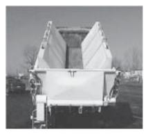
Because of the late arrival of test equipment last year, these tanks are again being tested this winter. The wedge-shaped tanks in the truck bed provide maximum
